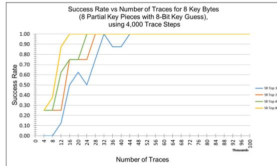
Figure 6.36: Success rates of 8-bit CPA selection function key guess size attacking 8 key bytes using 2 rounds of Keccak.
