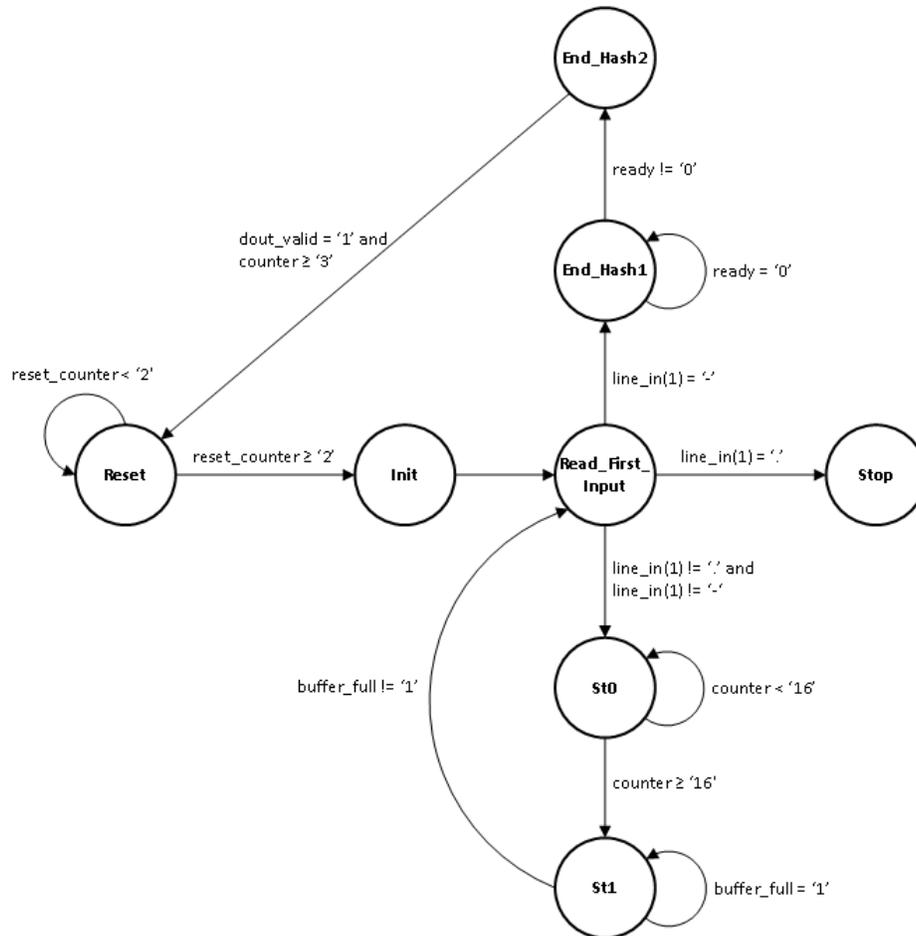
Figure 4.3: The high-speed core test bench state machine [16].
