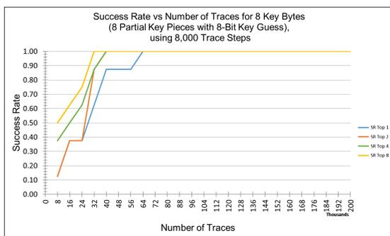
Figure 6.8: Success rates of 8-bit CPA selection function key guess size attacking 8 key bytes using 24 rounds of Keccak.
