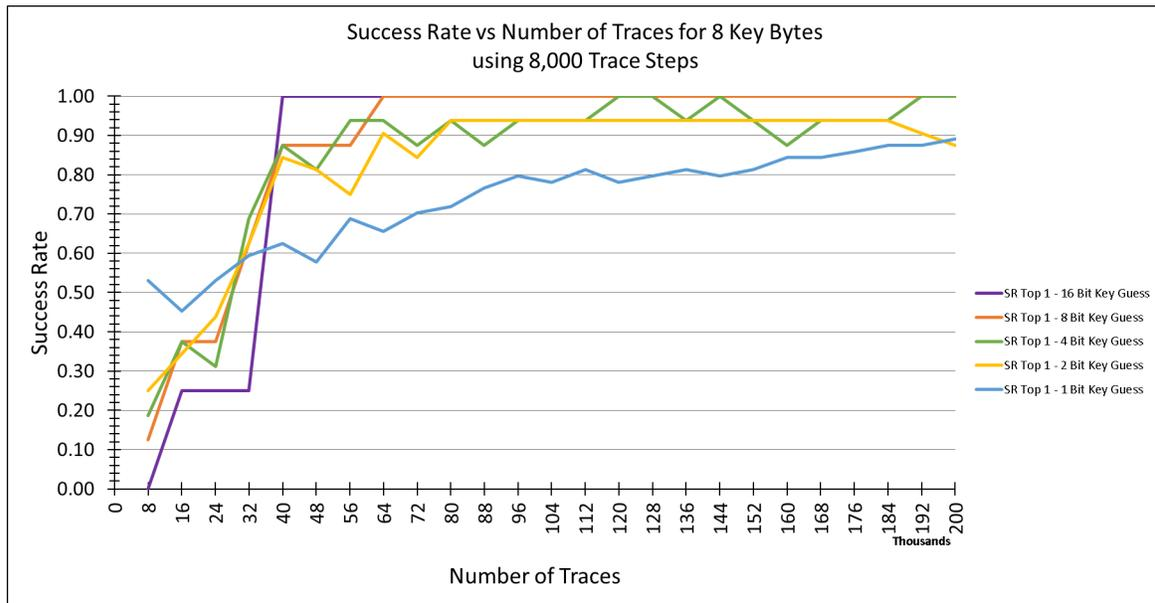
Figure 6.12: Success rates where the correct key is ranked first according to the correlation result for 1-bit, 2-bit, 4-bit, 8-bit and 16-bit CPA selection function key guess sizes when attacking 8 key bytes using 24 rounds of Keccak.
