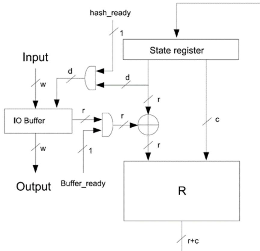
Figure 4.1: The high-speed core with one round per clock cycle [16].
