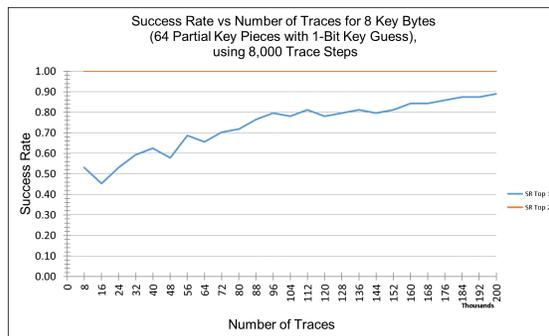
Figure 6.2: Success rates of 1-bit CPA selection function key guess size attacking 8 key bytes using 24 rounds of Keccak.
