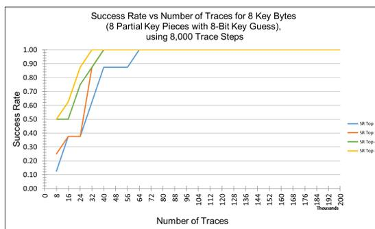
Figure 6.9: Success rates of 8-bit CPA selection function key guess size attacking 8 key bytes using 2 rounds of Keccak.
