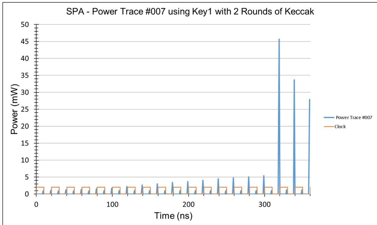
Figure 5.17: Simple power analysis of power trace #007 using Key1 with 2 rounds of Keccak.
