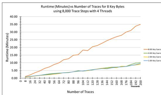
Figure 6.14: Runtime of 1-bit, 2-bit, 4-bit, and 8-bit CPA selection function key guess sizes using 24 rounds of Keccak.
