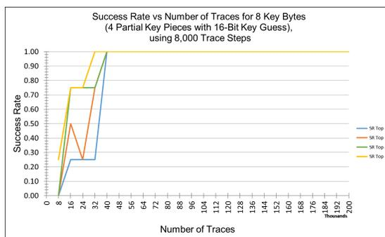
Figure 6.11: Success rates of 16-bit CPA selection function key guess size attacking 8 key bytes using 2 rounds of Keccak.
