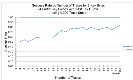
Figure 6.33: Success rates of 1-bit CPA selection function key guess size attacking 8 key bytes using 2 rounds of Keccak.
