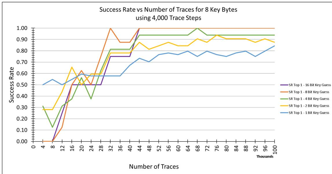
Figure 6.38: Success rates of the correct key that is ranked as top guess according to the correlation result for 1-bit, 2-bit, 4-bit, 8-bit and 16-bit CPA selection function key guess sizes attacking 8 key bytes using 2 rounds of Keccak.
