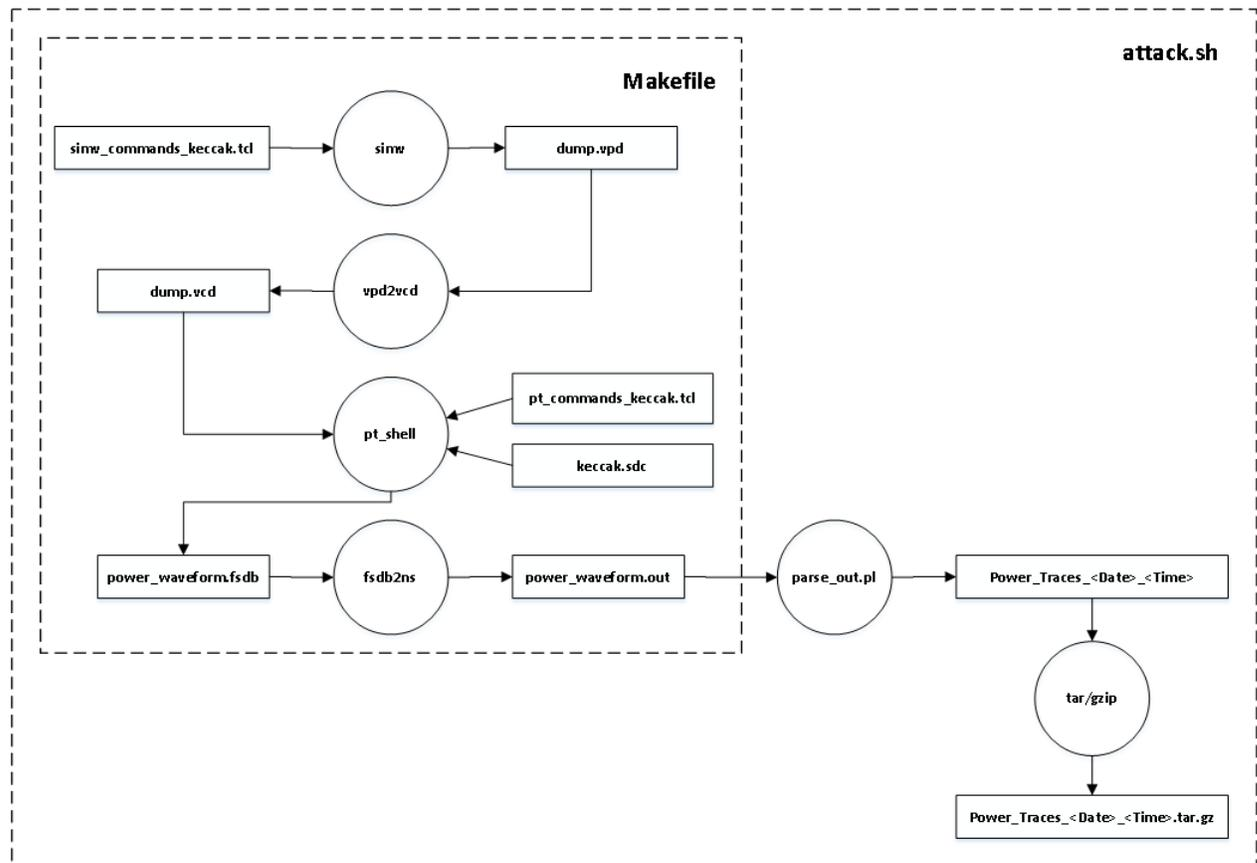
Figure 5.6: Simulation and power modeling flow.
