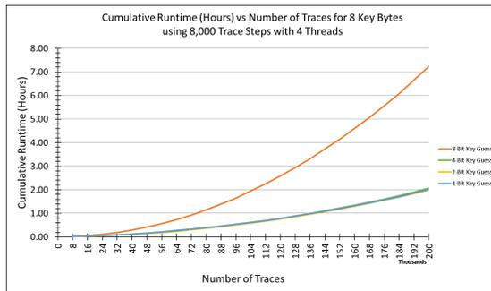
Figure 6.18: Cumulative runtime of 1-bit, 2-bit, 4-bit, and 8-bit CPA selection function key guess sizes using 24 rounds of Keccak.
