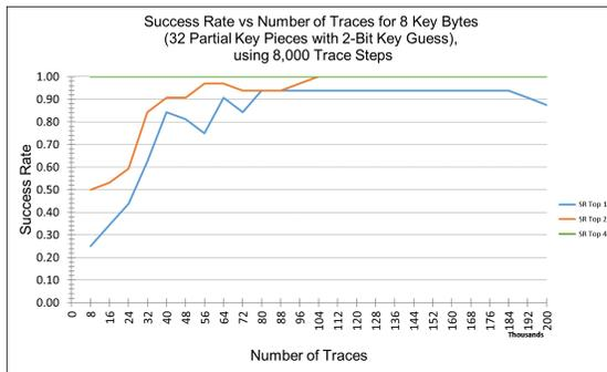
Figure 6.4: Success rates of 2-bit CPA selection function key guess size attacking 8 key bytes using 24 rounds of Keccak.
