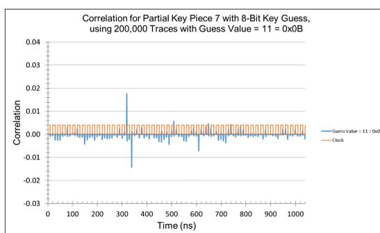
Figure 5.30: CPA time domain - examining the wrong key byte guess value for 24 rounds of Keccak using 200K traces that used Key1.
