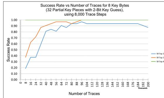
Figure 6.5: Success rates of 2-bit CPA selection function key guess size attacking 8 key bytes using 2 rounds of Keccak.
