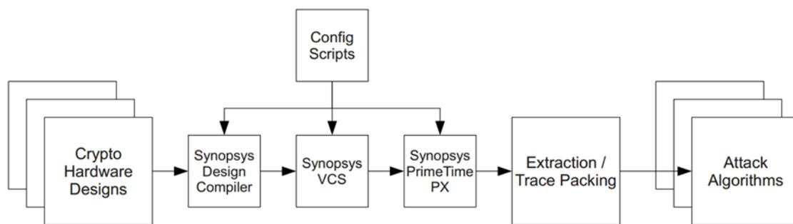
Figure 3.1: Ken Smith’s thesis: ASIC top-level simulation flow [9].
