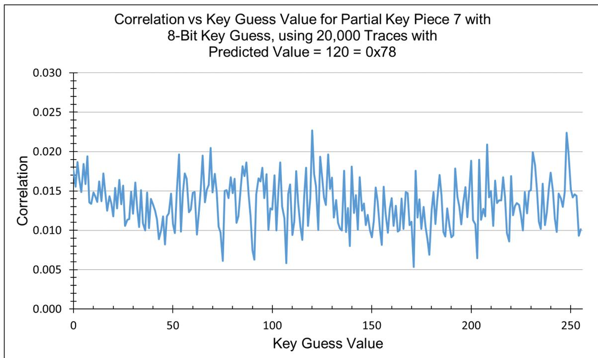
Figure 5.26: CPA predicted the wrong key value for Key Piece 7 using 2 rounds of Keccak.
