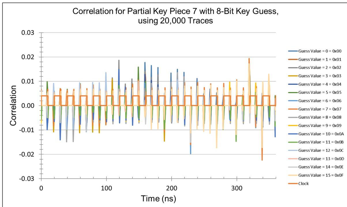
Figure 5.20: CPA time domain - 2 rounds of Keccak using 20K traces with Key1.
