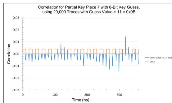
Figure 5.24: CPA time domain - examining the wrong key byte guess value for 2 rounds of Keccak using 20K traces that used Key1.
