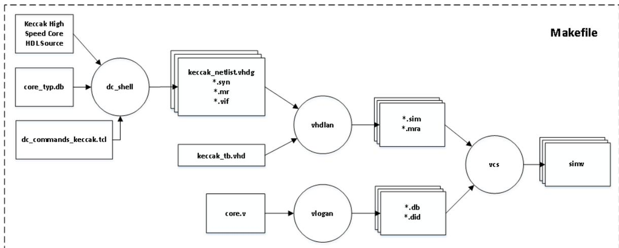
Figure 5.4: Hardware synthesis and simulation executable generation flow.
