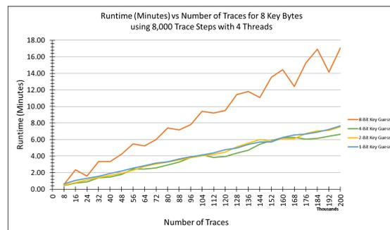
Figure 6.15: Runtime of 1-bit, 2-bit, 4-bit, and 8-bit CPA selection function key guess sizes using 2 rounds of Keccak.
