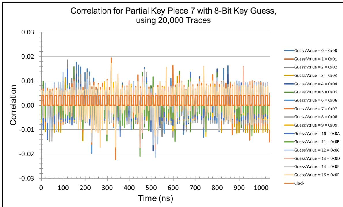
Figure 5.19: CPA time domain - 24 rounds of Keccak using 20K traces with Key1.
