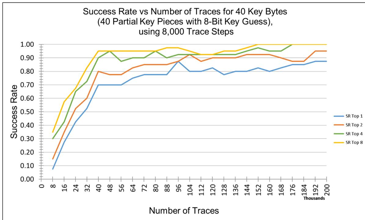
Figure 6.24: Success rates of 8-bit CPA selection function key guess size attacking 40 key bytes using 2 rounds of Keccak.
