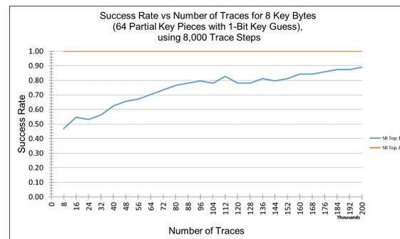
Figure 6.3: Success rates of 1-bit CPA selection function key guess size attacking 8 key bytes using 2 rounds of Keccak.
