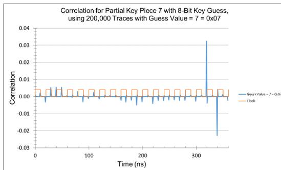
Figure 5.31: CPA time domain - examining the correct key byte guess value for 2 rounds of Keccak using 200K traces that used Key1.
