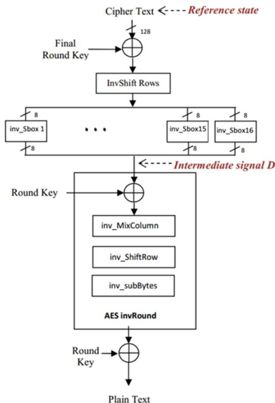
Figure 3.3: AES round 10 CPA attack using Hamming distance model [11].
