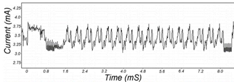
Figure 2.11: SPA trace showing DES algorithm's initial permutation, 16 rounds, and final permutation [6].
