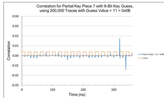
Figure 5.32: CPA time domain - examining the wrong key byte guess value for 2 rounds of Keccak using 200K traces that used Key1.
