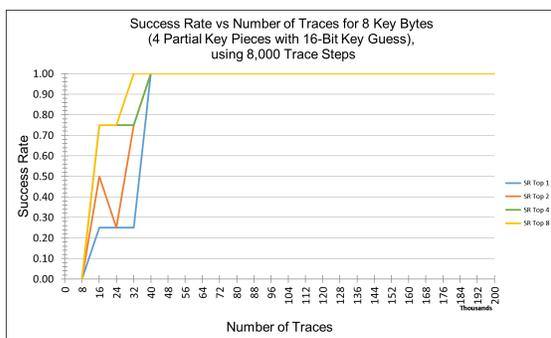
Figure 6.10: Success rates of 16-bit CPA selection function key guess size attacking 8 key bytes using 24 rounds of Keccak.
