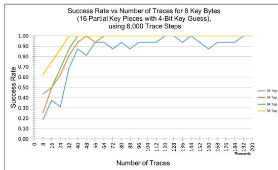
Figure 6.6: Success rates of 4-bit CPA selection function key guess size attacking 8 key bytes using 24 rounds of Keccak.
