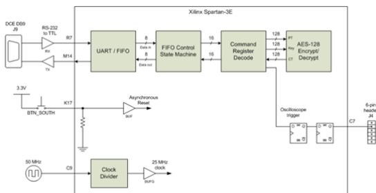
Figure 3.4: Xilinx Spartan-3E FPGA block diagram [12].
