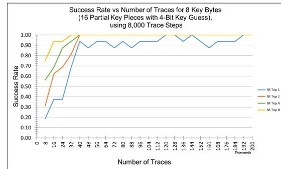
Figure 6.7: Success rates of 4-bit CPA selection function key guess size attacking 8 key bytes using 2 rounds of Keccak.
