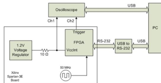
Figure 3.5: CPA platform setup using FPGA development board [12].
