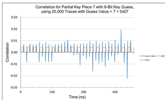
Figure 5.23: CPA time domain - examining the supposed “correct” key byte guess value for 2 rounds of Keccak using 20K traces that used Key1.
