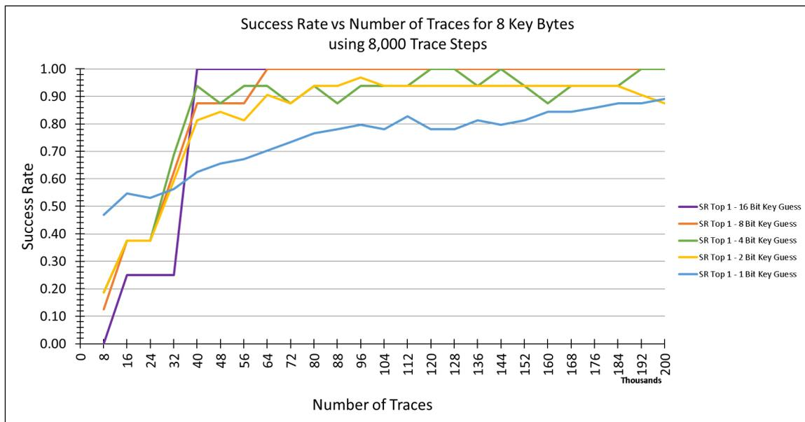
Figure 6.13: Success rates where the correct key is ranked first according to the correlation result for 1-bit, 2-bit, 4-bit, 8-bit and 16-bit CPA selection function key guess sizes when attacking 8 key bytes using 2 rounds of Keccak.
