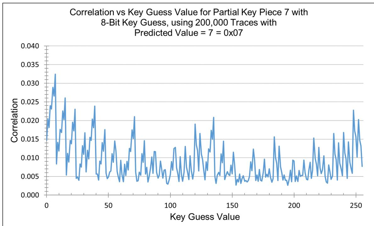
Figure 5.34: CPA predicted the correct key value for Key Piece 7 using 2 rounds of Keccak.
