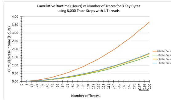
Figure 6.19: Cumulative runtime of 1-bit, 2-bit, 4-bit, and 8-bit CPA selection function key guess sizes using 2 rounds of Keccak.
