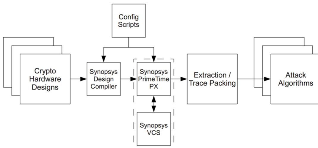
Figure 3.2: Garrett Smith’s thesis: modified ASIC top-level simulation flow [7].
