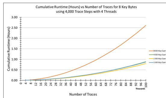
Figure 6.40: Cumulative runtime of 1-bit, 2-bit, 4-bit and 8-bit CPA selection function key guess sizes using 2 rounds of Keccak.
