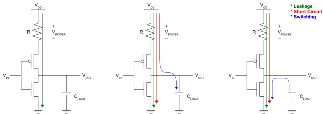
Figure 2.10: Idle consumption (left), charging (middle), discharging (right) [7] [8].
