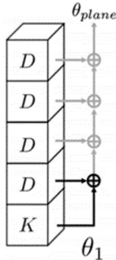
Figure 5.14: MAC-Keccak selection function target for one unknown key piece [14].
