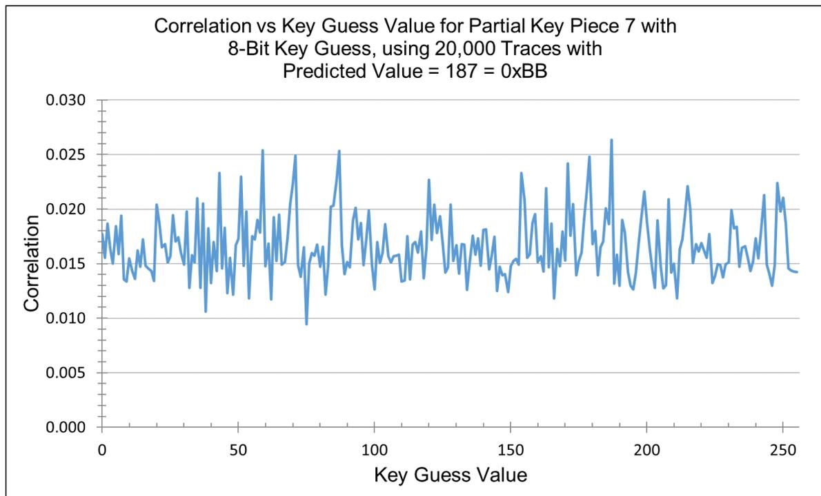
Figure 5.25: CPA predicted the wrong key value for Key Piece 7 using 24 rounds of Keccak.
