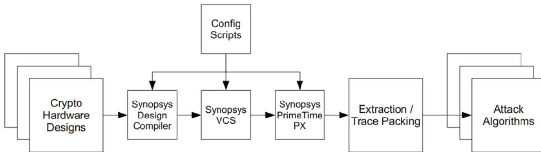
Figure 5.1: ASIC top-level simulation flow [9].
