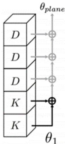
Figure 5.38: MAC-Keccak selection function target for two unknown key pieces [14].
