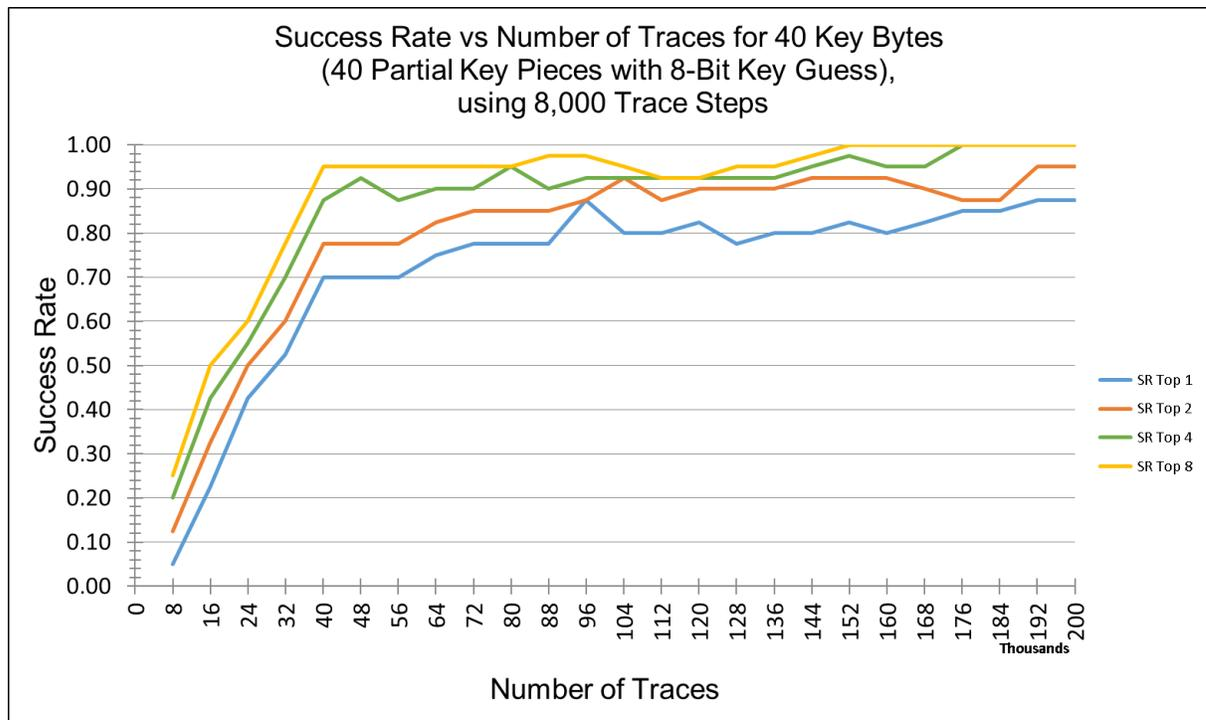
Figure 6.23: Success rates of 8-bit CPA selection function key guess size attacking 40 key bytes using 24 rounds of Keccak.
