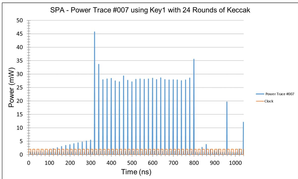
Figure 5.16: Simple power analysis of power trace #007 using Key1 with 24 rounds of Keccak.
