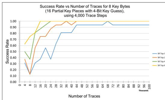
Figure 6.35: Success rates of 4-bit CPA selection function key guess size attacking 8 key bytes using 2 rounds of Keccak.
