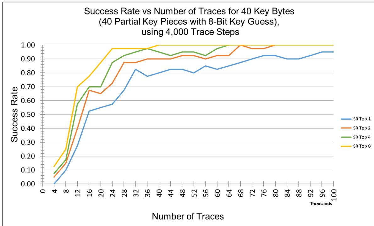
Figure 6.43: Success rates of 8-bit CPA selection function key guess size attacking 40 key bytes using 2 rounds of Keccak.
