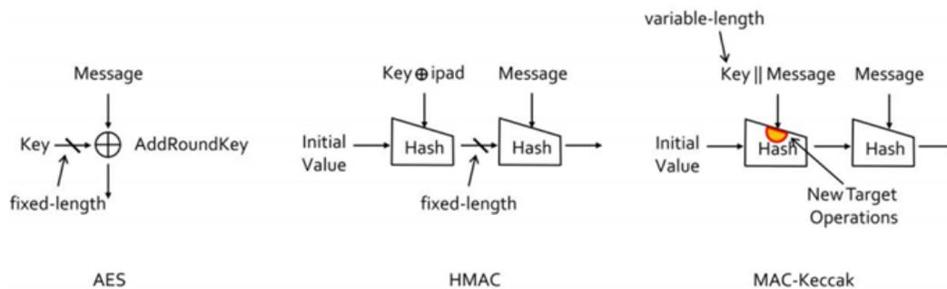
Figure 3.9: The difference between the CPA of AES, HMAC, and MAC-Keccak [14].
