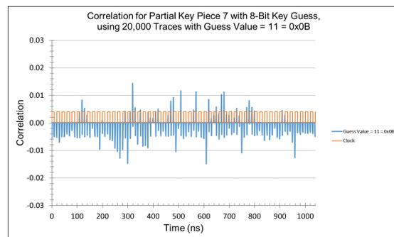
Figure 5.22: CPA time domain - examining the wrong key byte guess value for 24 rounds of Keccak using 20K traces that used Key1.
