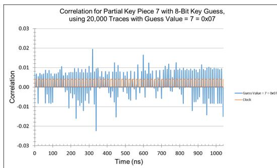
Figure 5.21: CPA time domain - examining the supposed “correct” key byte guess value for 24 rounds of Keccak using 20K traces that used Key1.
