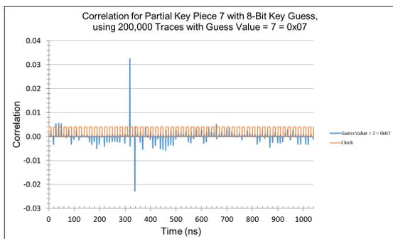
Figure 5.29: CPA time domain - examining the correct key byte guess value for 24 rounds of Keccak using 200K traces that used Key1.
