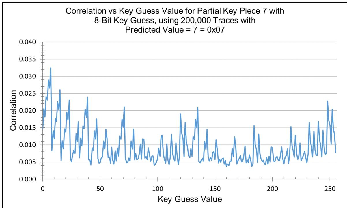
Figure 5.33: CPA predicted the correct key value for Key Piece 7 using 24 rounds of Keccak.
