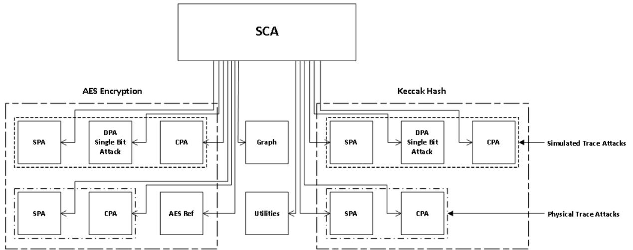
Figure 5.10: Top level class diagram of the attack framework.
