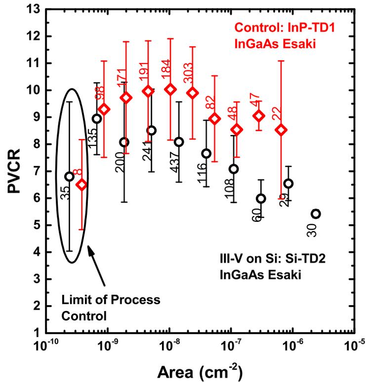
**Figure 7.10:** Devices are sorted by area and display the mean, range, and population. Using the nearest neighbor area to compare between InP-TD1 and Si-TD2 it can be seen that sample variation overlaps and that the means begin to converge. Below  $8.7 \times 10^{-10} \text{ cm}^2$ , t-tests confirm that there is at most 1% error in assuming equivalent PVCN.
