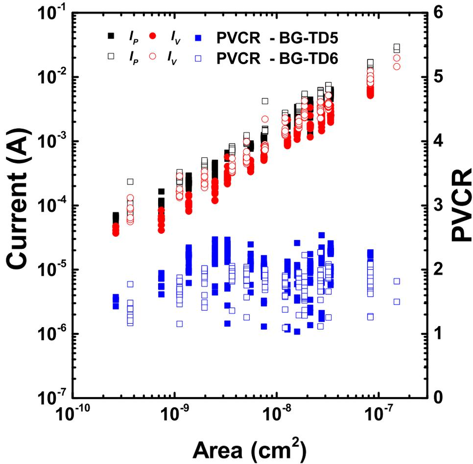
**Figure 6.16:**  $I_V$  and  $I_P$  vs. area for BG-TD5 and BG-TD6 show an increased  $J_P$  when reducing the  $i$ -layer thickness between the n and p regions, due to an increased electric field allowing increased carrier tunneling. Similarly, PVCr increases when the  $i$ -layer thickness is increased likely due to the increased screening that a wider tunnel region presents for excess currents.
