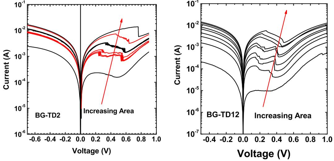
(a) Family of  $I$ - $V$  Curves for BG-TD2(b) Family of  $I$ - $V$  Curves for BG-TD12
