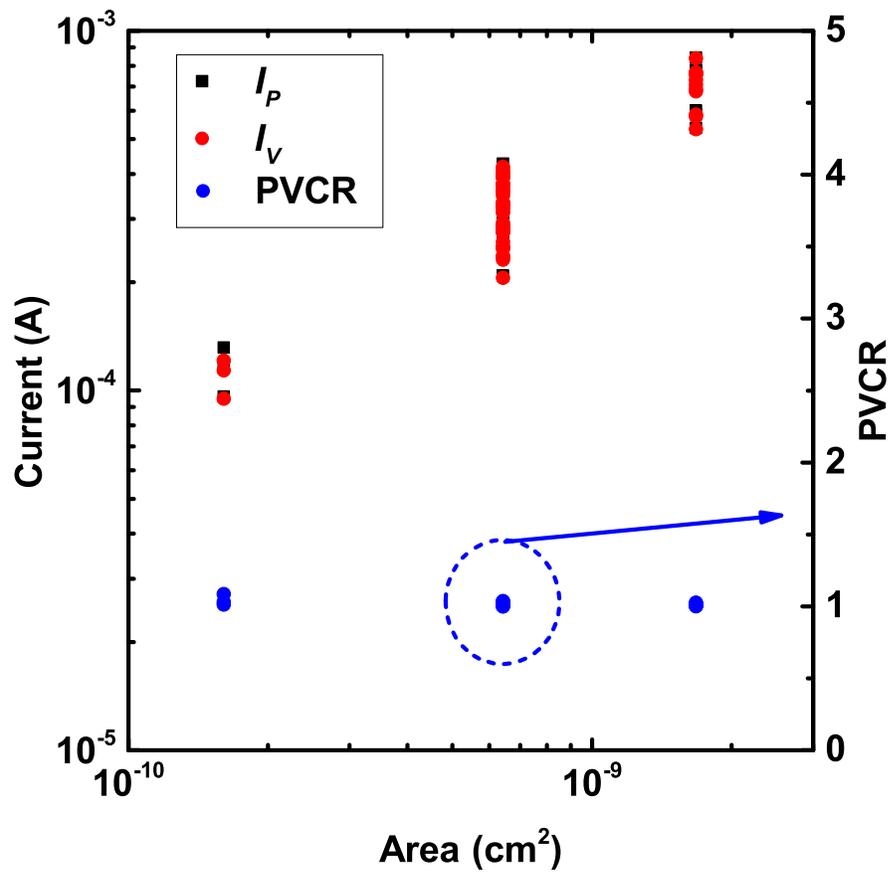
**Figure 5.14:** LSG-5 displays scaling with area, however due to undercut during wet etch most devices were etched away.
