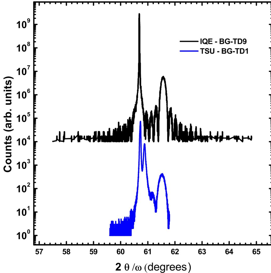
**Figure 6.39:** HRXRD of BG-TD1 and BG-TD9 samples indicates the presence of an offcut as well as the lack of a secondary peak near the GaSb substrate peak for BG-TD9, a correction of  $0.7^\circ$  was included to align the GaSb peaks. The excellent crystal structure of both samples would indicate that dislocation defects should have minimal impact on device performance.
