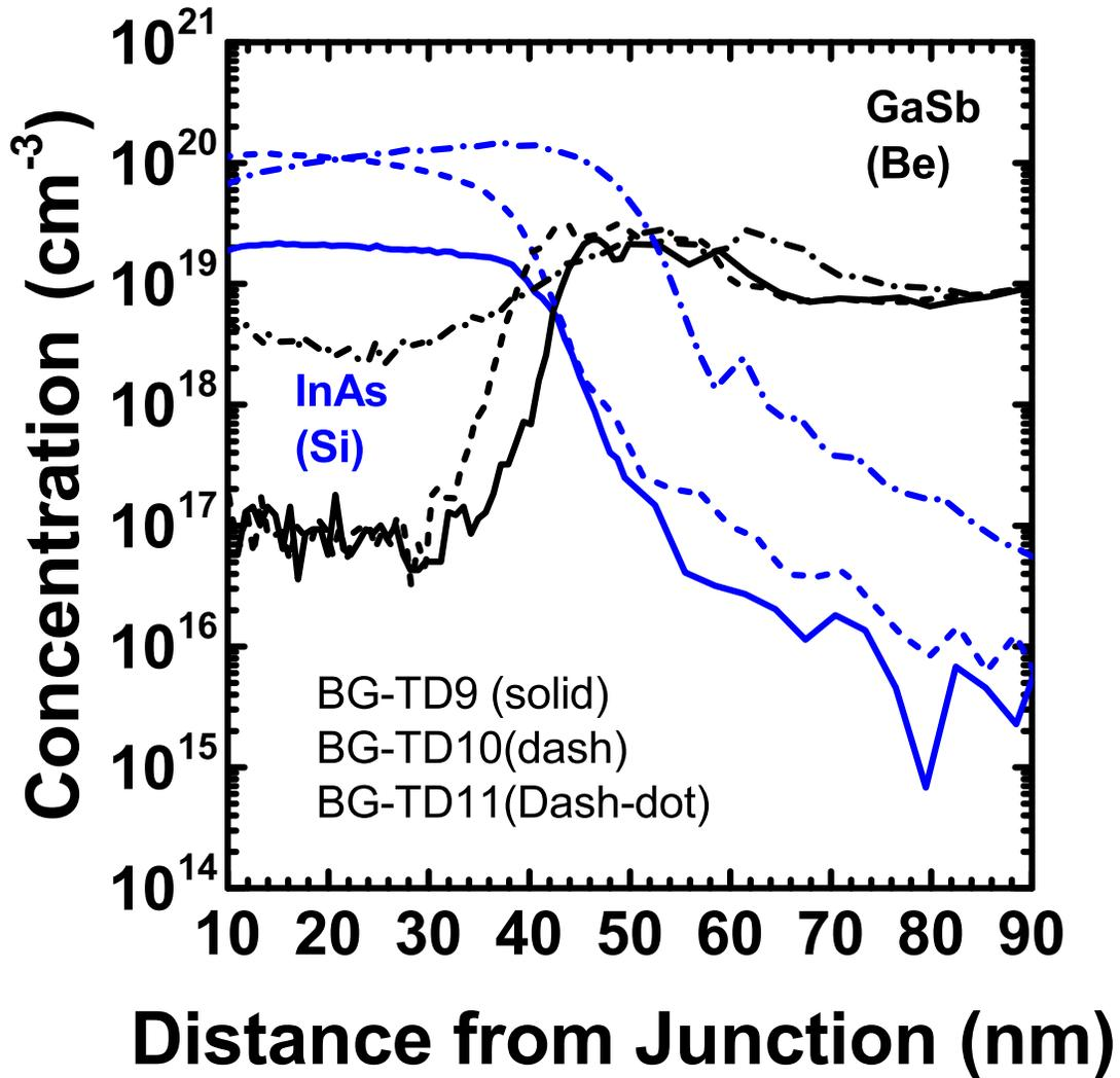
**Figure 6.30:** SIMS was performed on the samples to determine dopant levels present within the sample. BG-TD9, BG-TD10, and BG-TD11 were found to have Si and Be doping levels near the targeted values. As levels within the GaSb film region were near the detection limit, and should not produce a satellite peak in HRXRD measurements.
