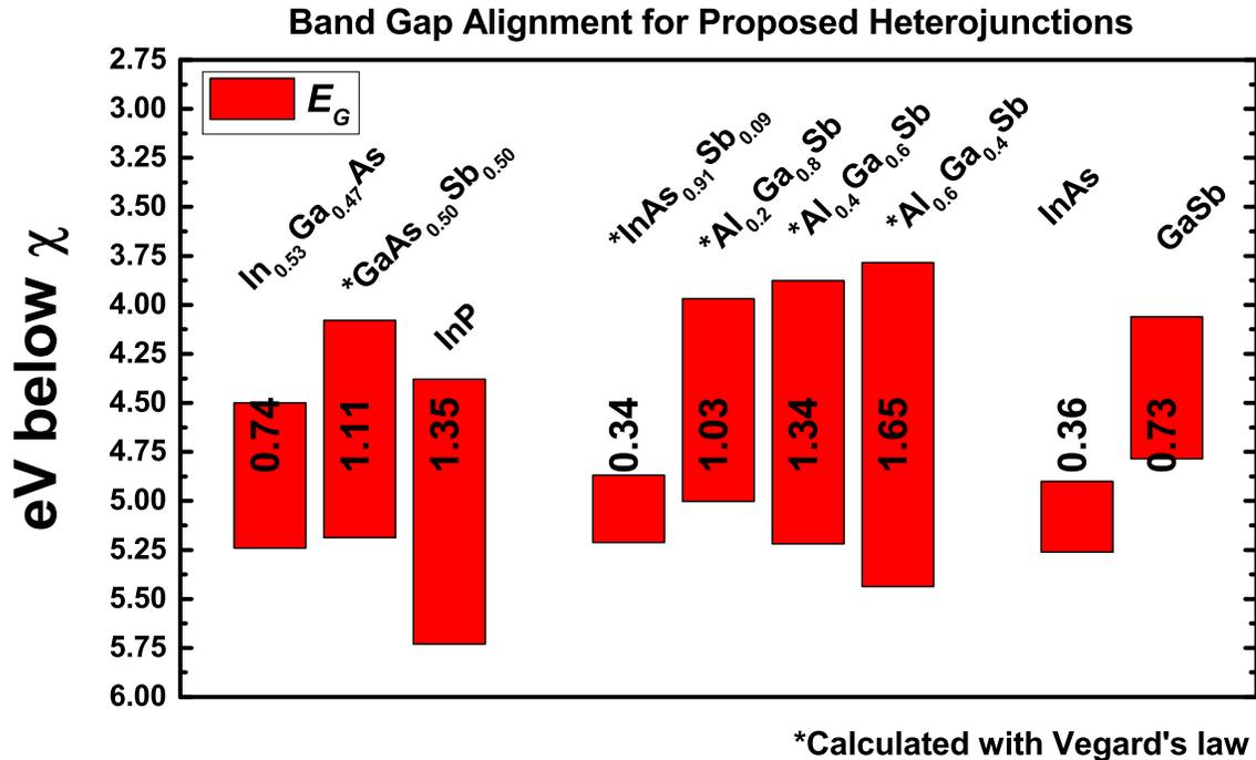
**Figure 1.2:** Band gap line up for several binary and ternary semiconductors to be used in this work. Ternary compound band gaps were calculated using Vegard's rule, and are approximate. A more accurate set of band alignments could be extracted from the band information in Figs. A.1 and A.2 from Vurgaftman et al. [33]
