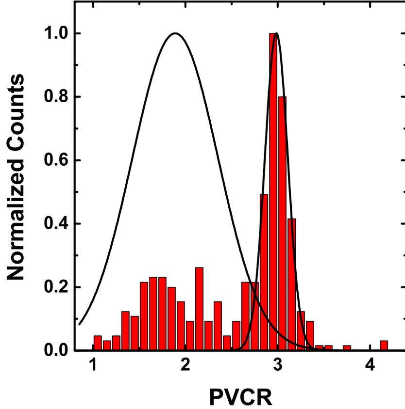
**Figure 6.11:** From the histogram of PVCr values, there appears to be a bimodal distribution of PVCr as shown by the two peak fits. It possible that there are processing factors in play that would cause such a characteristic to appear.
