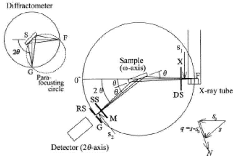
**Figure 3.7:** A typical HRXRD measurement set up shown by Shinoda et al. [133].<sup>3</sup>
