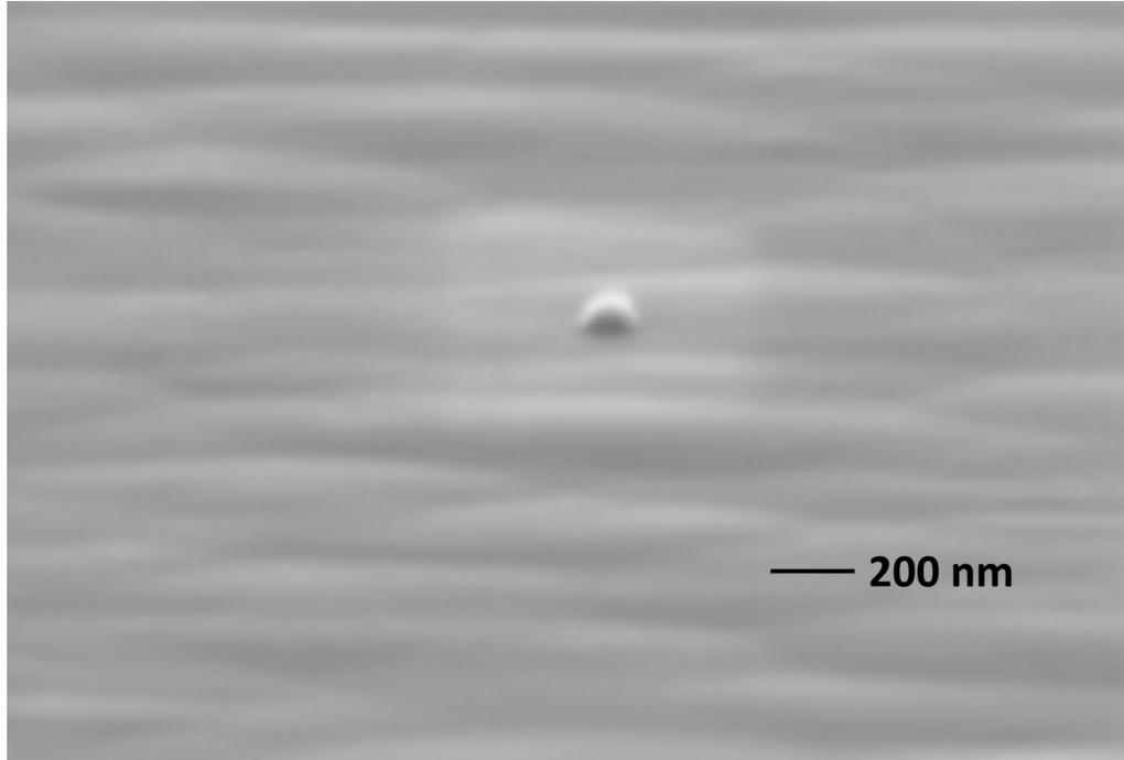
**Figure 4.12:** Surface roughness is very apparent for sample SSG-TD3 from SEM micrographs, indicating probable large defect densities and a relaxed layer.
