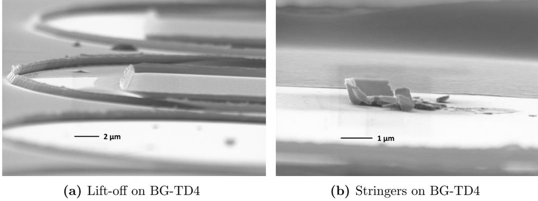
**Figure 6.19:** Intitial lift off processes for L1 lead to stringers which would cause shorting between the contact and the mesa. This creates additional shunt paths which reduce PVCR.
