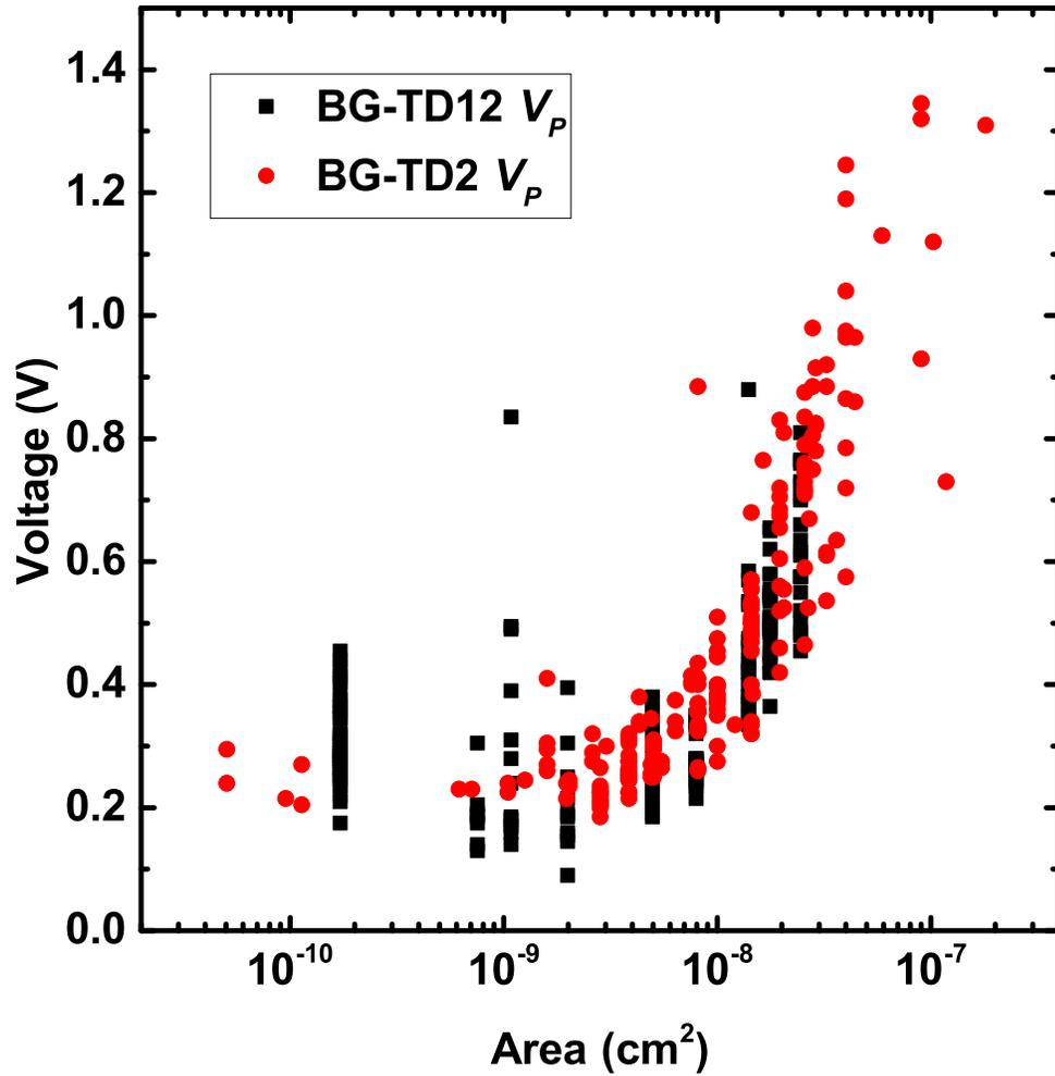
**Figure 6.47:** Typical minimum  $V_P$  values for the series 2  $i$ -layer devices appear to fall between 0.3 V and 0.2 V, indicating minimal influence from  $R_S$ .
