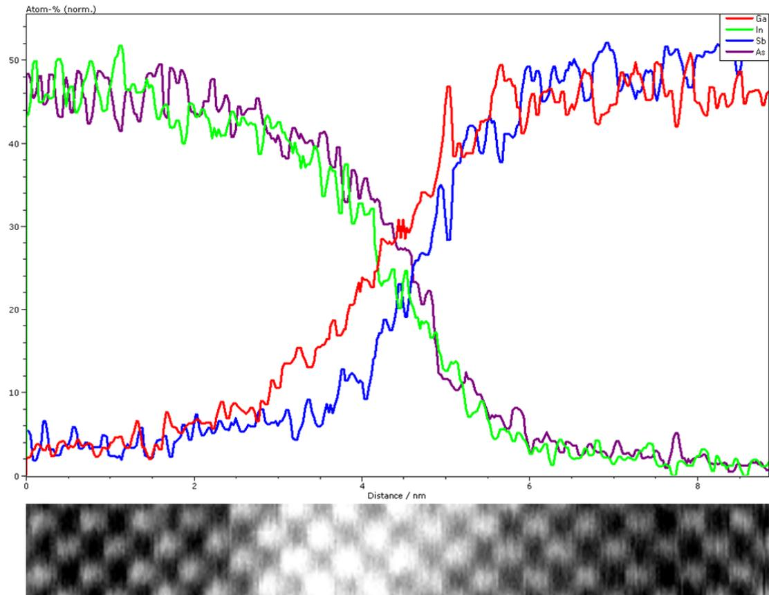
**Figure 6.42:** XPS during TEM analysis of the BG-TD1 junction shows an InSb like interface and was found to be largely defect free.
