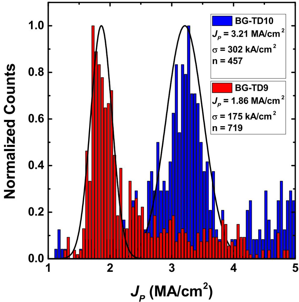
**Figure 6.34:** Normalized  $J_p$  histograms for series 2 study showing  $1.82 \text{ MA/cm}^2$  and  $3.21 \text{ MA/cm}^2$   $J_p$  for BG-TD9 and BG-TD10. Based on the SIMS data,  $J_p$  may be pushed higher if both dopants can exceed  $1 \times 10^{20} \text{ cm}^{-3}$ .
