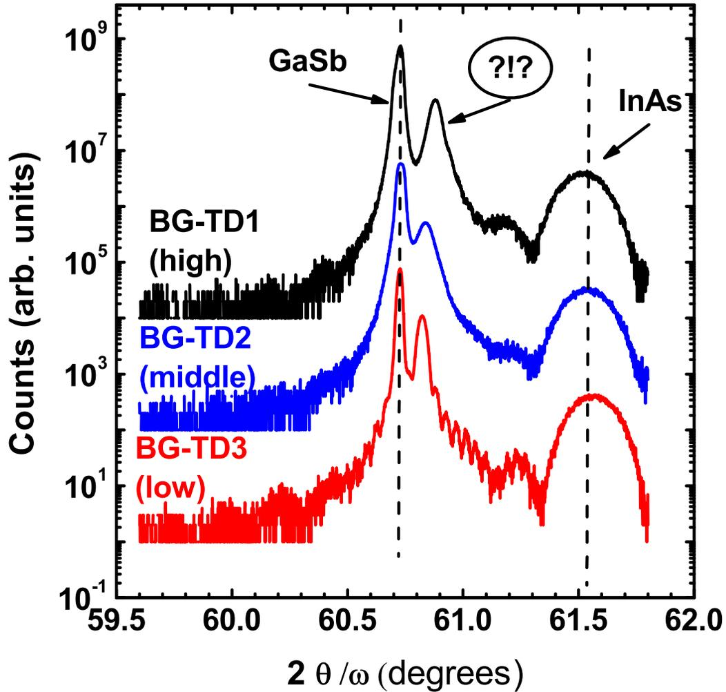
**Figure 6.3:**  $\omega/2\theta$  curves for the InAs/GaSb tunnel diodes exhibit an additional sharp peak near the GaSb line. This peak may be indicative of a variation in film composition for the 300 nm GaSb region.
