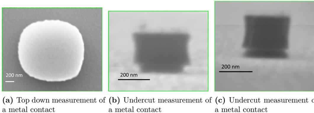
**Figure 3.4:** (a) Mesa areas are measured with a top down image capture and extracted by a Matlab<sup>TM</sup> script which provides a best fit for the area. (b) Undercut of the metal contact is measured from two perpendicular angles to capture the anisotropy of the wet etch for inclusion in area correction calculations.
