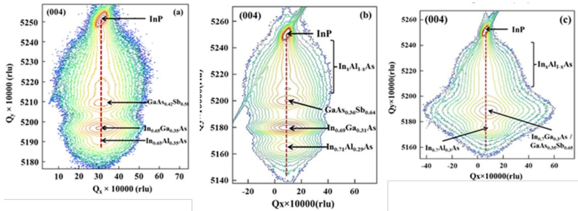
**Figure 3.9:** RSM of InGaSb/GaAsSb device, the lack of a sharp peak region indicates a highly defected  $\text{In}_{0.70}\text{Ga}_{0.30}\text{As}/\text{GaAs}_{0.35}\text{Sb}_{0.65}$  region as well as significant relaxation of the lattice [34].<sup>5</sup>
