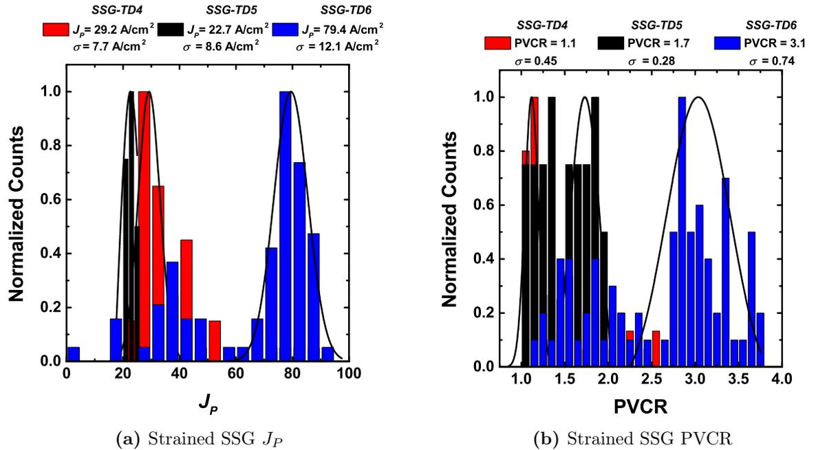
**Figure 4.16:**  $J_p$  and PVCR histograms for strained SSG samples. (a)  $J_p$  values decreased with tensile strain which may indicate an unfavorable change in  $m^*$ . However, the strain samples are also likely affected by the increased  $E_G$  seen at the tunneling interface [30]. (b) PVCR are, on average low, indicating a number of defects are increasing excess current and masking strain effects on PVCR.
