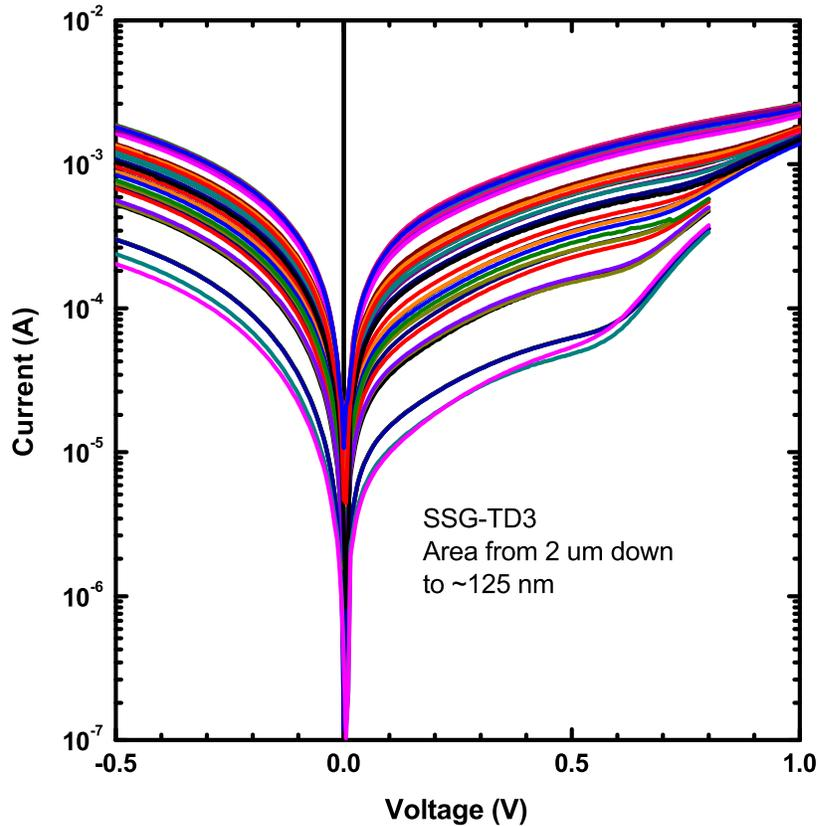
**Figure 4.11:** Typical  $I$ - $V$  characteristics for SSG-TD3. This device was designed to be closer to InAs in effective  $E_G$ , however high defect density affected the devices to the point that excess current completely masks the tunnel region of the  $I$ - $V$  curves.
