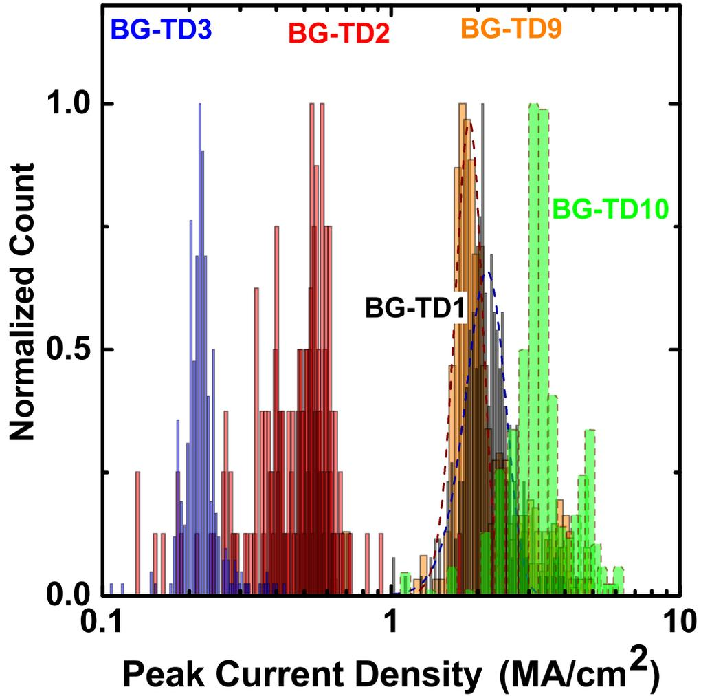
**Figure 6.38:**  $J_P$  histograms for the Series 1 and Series 2 BG diodes. BG-TD1 and BG-TD9 were nearly identical and BG-TD10 exhibits  $J_P$  greater than 3 MA/cm<sup>2</sup>.
