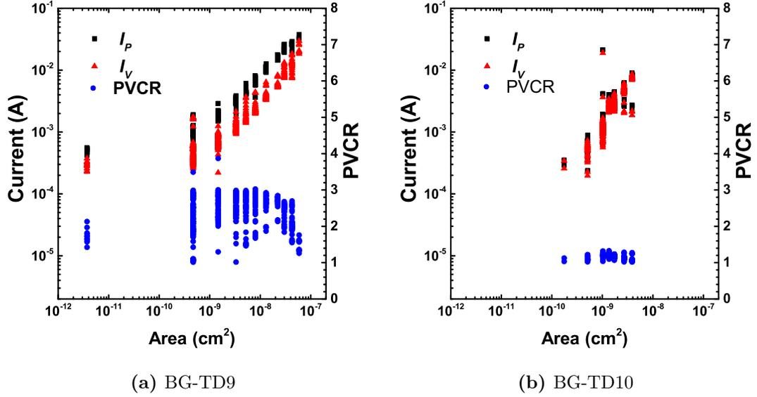
**Figure 6.33:** Current was shown to scale for both BG-TD9 and BG-TD10 with area.
