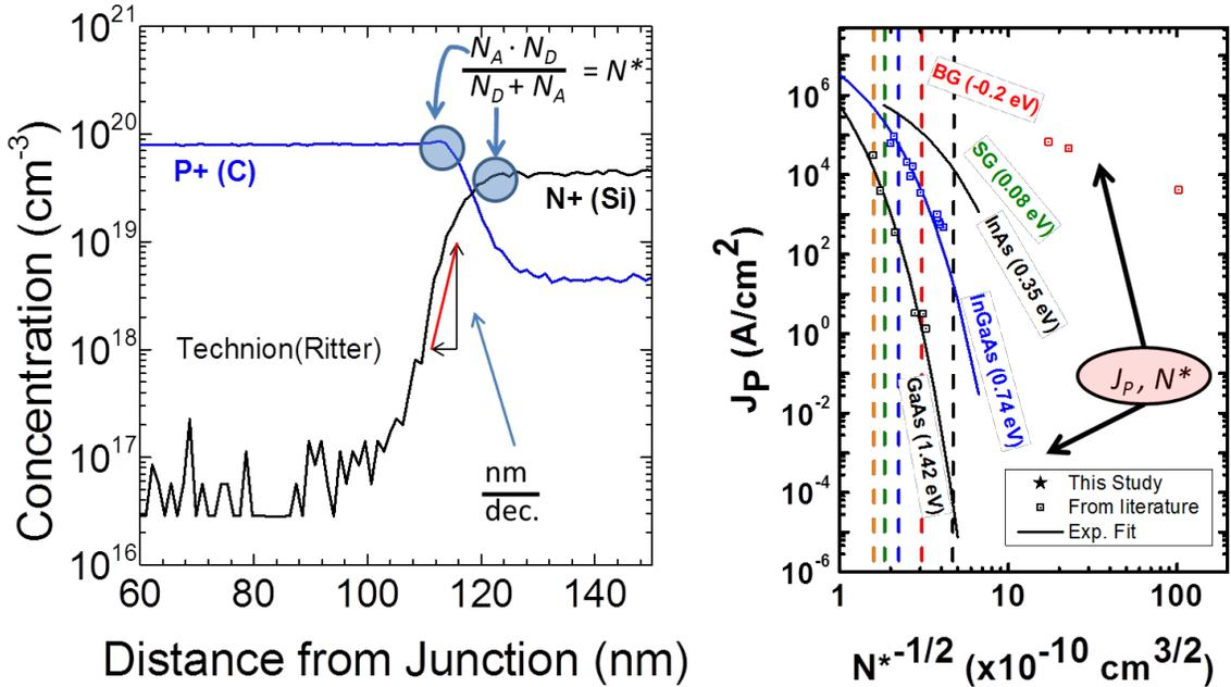
**Figure 3.6:** SIMS plot of a  $200 \text{ kA}/\text{cm}^2$   $J_P$  device showing the dopant species and level on either side of the junction. (a) The inlays detail the methods for calculating the junction abruptness as well as  $N^*$ . (b) Figure of merit plot showing where  $J_P$  and  $N^*$  will be applied to compare devices [50, 57, 132].
