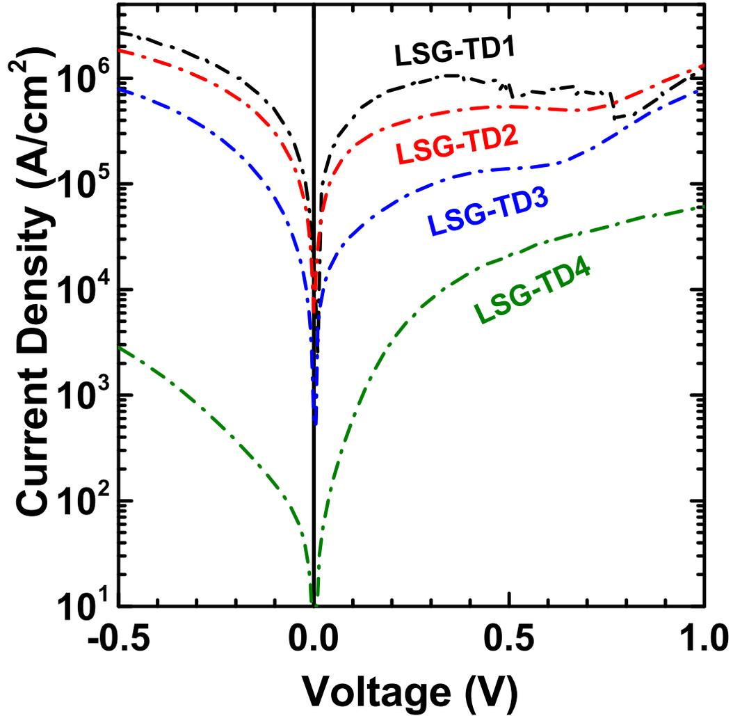
**Figure 5.4:** Family of  $J$ - $V$  curves for similarly sized devices in the LSG series. LSG-1 exhibits the best  $J_P$  and PVCR, at  $872 \text{ kA/cm}^2$  and 3.05, respectively. LSG-2 and LSG-3 show modest PVCR and  $J_P$  commensurate with their doping density, at  $521 \text{ kA/cm}^2$  and  $356 \text{ kA/cm}^2$ . LSG-4 presents an interesting case, as no NDR is observed, but the doping is only 1/5 that of LSG-3 indicating a promising candidate material system for a TFET.
