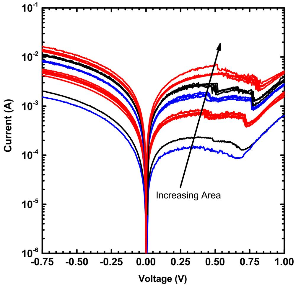
**Figure 5.8:** Family of  $I$ - $V$  curves for LSG-TD1 show excellent current scaling area is reduced.
