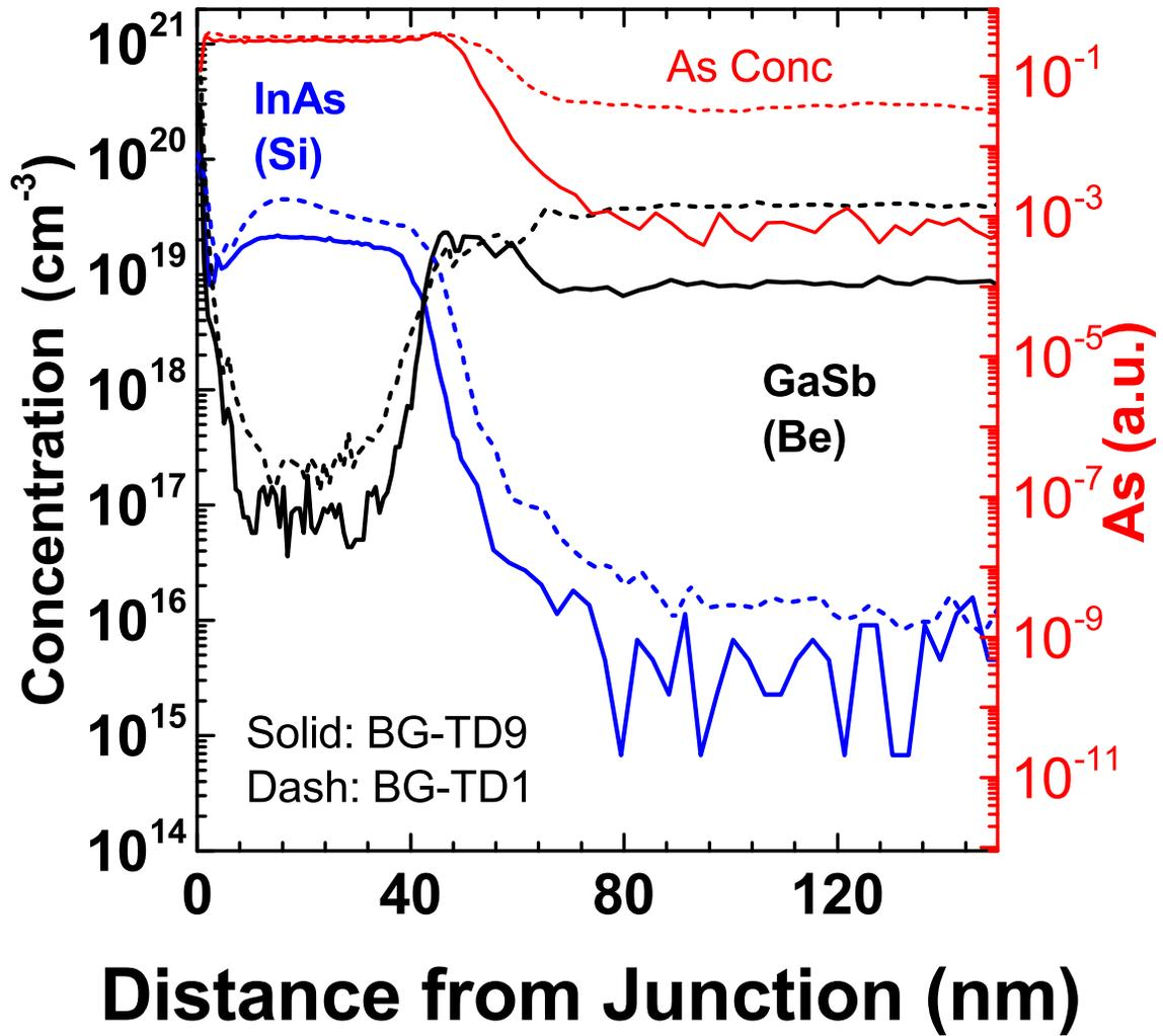
**Figure 6.40:** SIMS of BG-TD1 and BG-TD9 samples indicates the presence of an As in BG-TD1. Doping for BG-TD9 was slightly lower than that of BG-TD1
