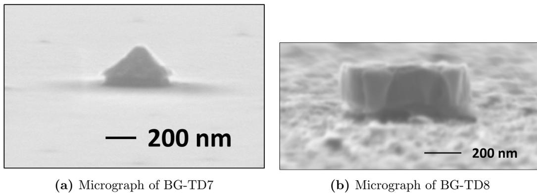
**Figure 6.27:** As shown in the SEM micrographs (a) and (b), processing issues confound area analysis by leaving uneven contacts and possible shorts to the mesa.
