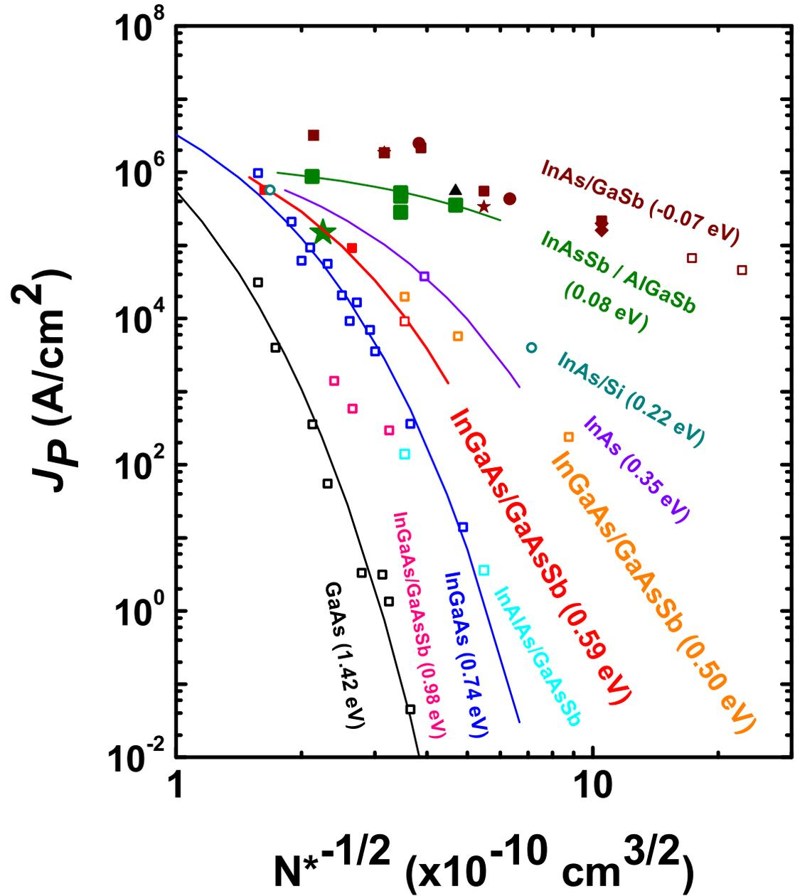
**Figure 6.50:** Figure of merit plot with data from all BG samples in this dissertation overlaid with other reported tunnel diodes.
