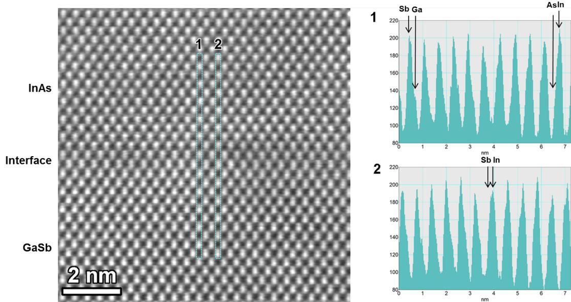
**Figure 6.6:** TEM analysis of the TD7A junction shows an InSb like interface and was found to be largely defect free.
