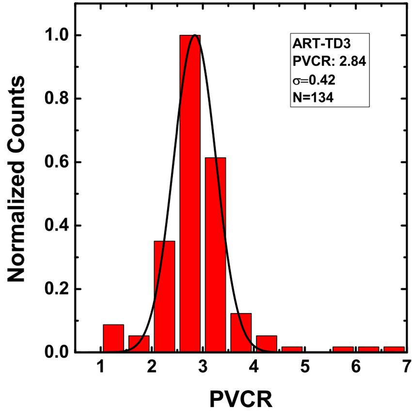
**Figure 7.17:** Histogram of PVCR from which a value of 2.84 was extracted from a Gaussian fit.
