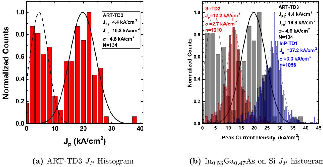
**Figure 7.15:** (a) A bimodal distribution of  $J_P$  caused by large area defects required a two peak extraction. (b) Histogram of  $J_P$  for ART-TD3, which shows the  $J_P$  value as compared to the control and buffer layer samples.
