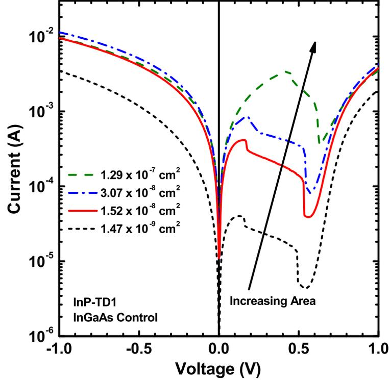
**Figure 7.6:** Representative  $I$ - $V$  characteristics for InP-TD1 device areas ranging from  $0.25 \mu\text{m}^2$  to  $100 \mu\text{m}^2$ . NDR was present at room temperature, indicating the presence of good tunnel junctions.
