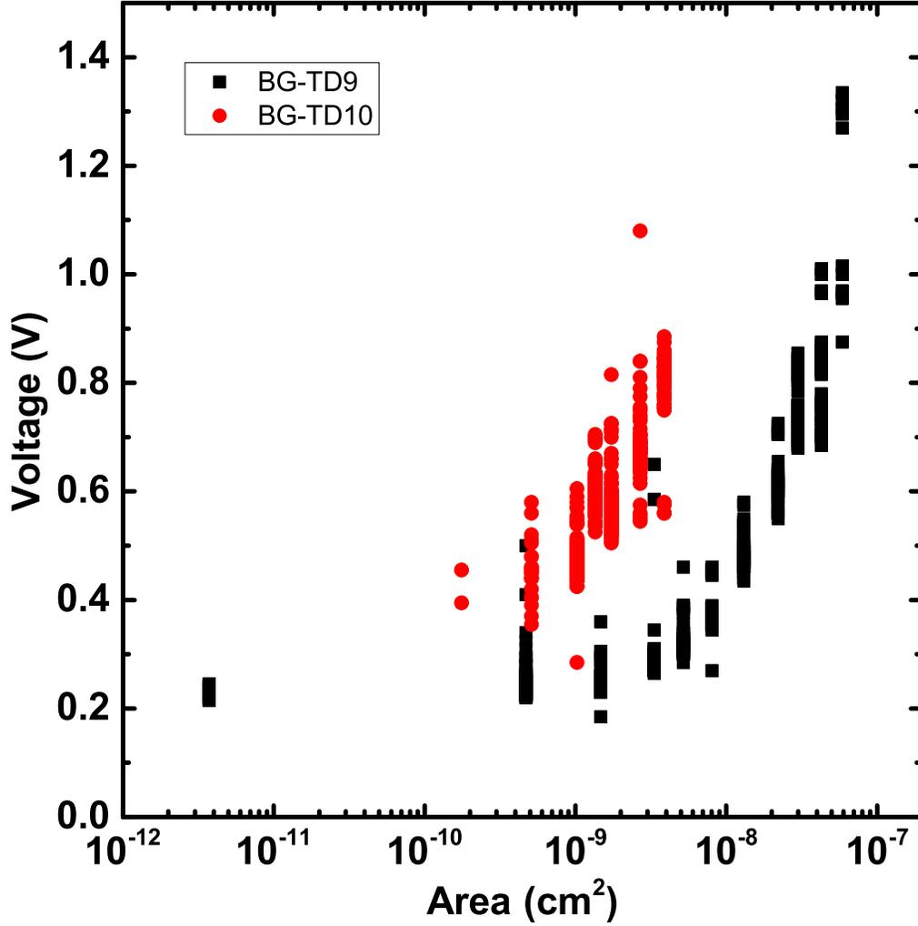
**Figure 6.32:** Typical minimum  $V_P$  values for series 2 devices appear to fall between 0.3 V and 0.2 V, with greater influence from  $R_S$  for BG-TD10 due to the higher  $J_P$ .
