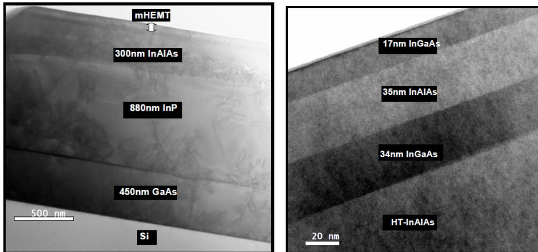
(a) Cross-sectional TEM of mHEMT device showing substrate and buffer
