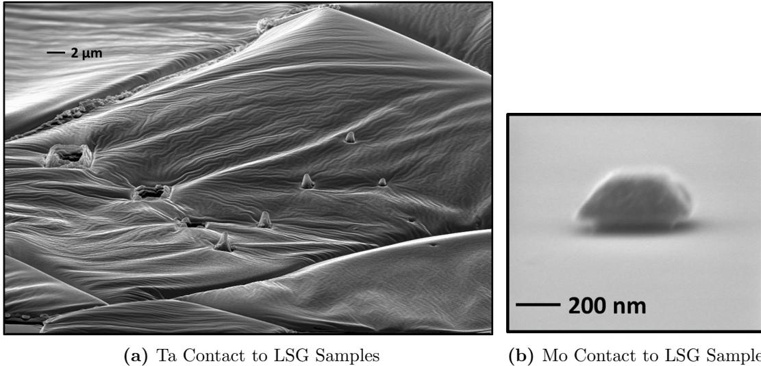
**Figure 5.3:** (a) Initial attempts to utilize liftoff processes for refractory metal contacts to the LSG samples required a major shift in procedure. (b) Changing from lift-off to a metal first and etch back process eliminated issues with sidewall metal coating *and* had the benefit of producing smaller L1 contacts. Processes for both Mo and W were developed for L1 contacts, but the limited availability of W lead to Mo utilization as the contact for most devices.
