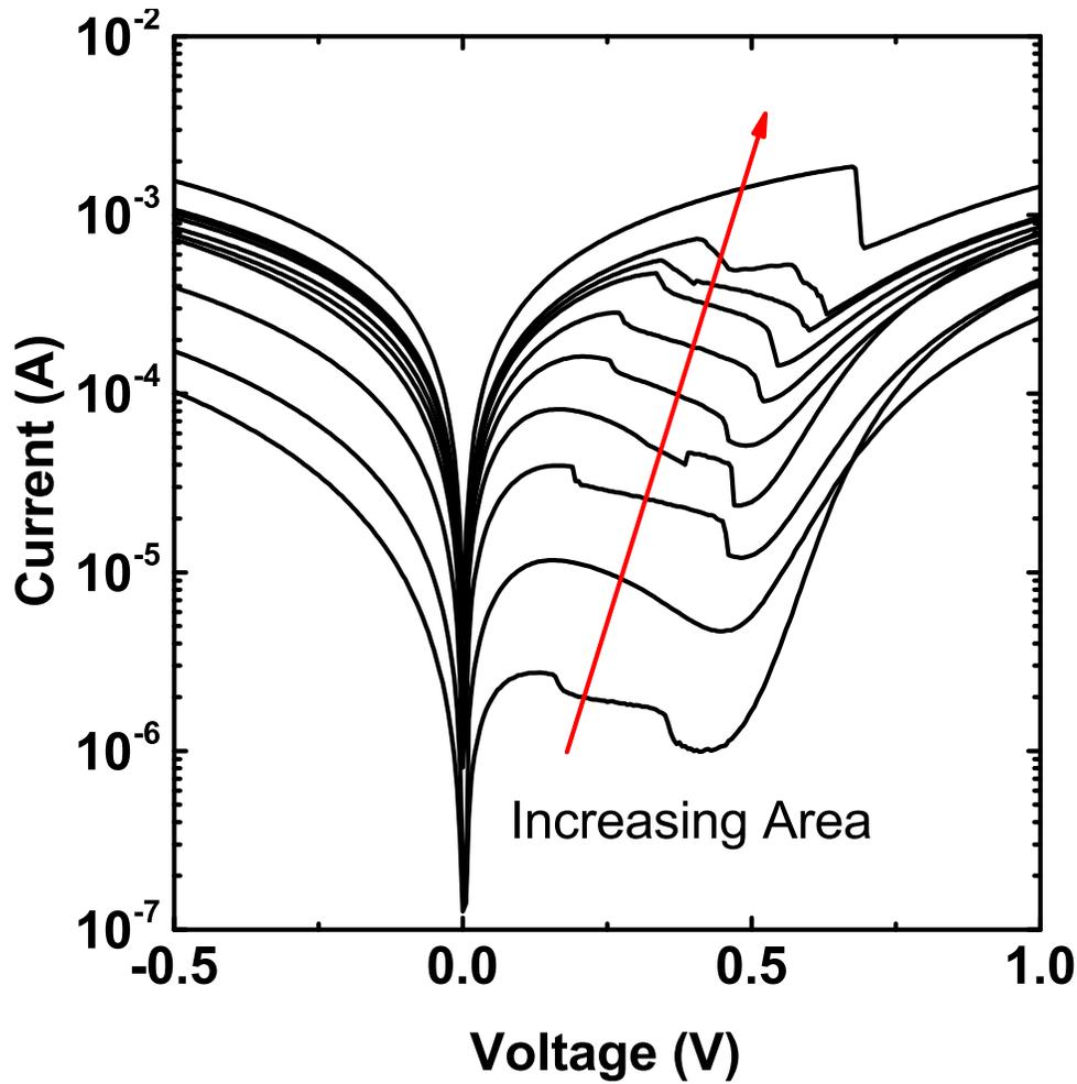
**Figure 7.14:** Sample ART-TD3 exhibits a reduced NDR region, this is very likely due to the roughness of sample surface. Because the sample is more rough than Si-TD2, it displays poorer PVCR characteristics which are commensurate with the level of defects within the film.
