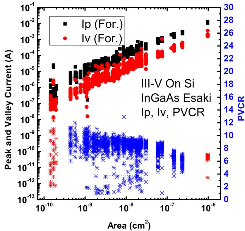
**Figure 7.9:**  $J_V$ ,  $J_P$ , and PVCr values for Si-TD2 are plotted against device area. Generally, there is a wider spread in the data with respect to InP-TD1. A PVCr around 8.6 exhibits greater variability due to a greater defect density leading to higher  $J_V$  values.
