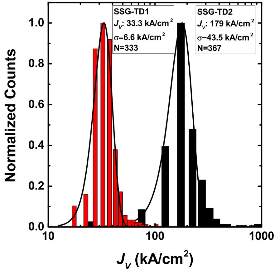
**Figure 4.6:**  $J_V$  histogram for SSG-TD1 and SSG-TD2 showing extracted values to be 33.3  $\text{kA/cm}^2$  and 179  $\text{kA/cm}^2$ , respectively.  $\sigma$  values are between 20% and 25%, indicating that area variation between devices is likely higher than the fitted value.
