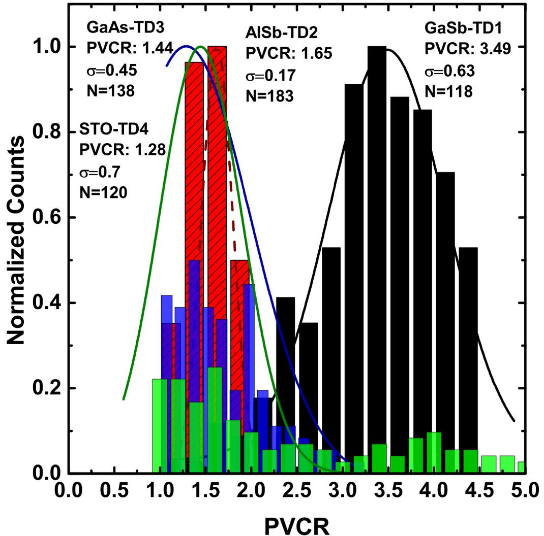
**Figure 8.5:** Normalized PVCR histograms for BG on Si study, with GaAs-TD3 and STO-TD4 scaled for visibility, showing that median values for PVCR are quite similar across devices on a buffer. However, samples with the smallest defect density show significantly higher PVCR range.
