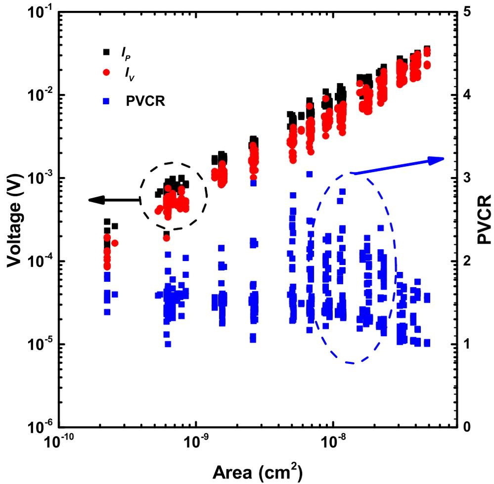
**Figure 5.9:** Current *vs.* area plot for LSG-TD1 which shows excellent scaling with area. PVCRCR is also plotted *vs.* area, and appears to have a peak which may be due to a number of leakage paths.
