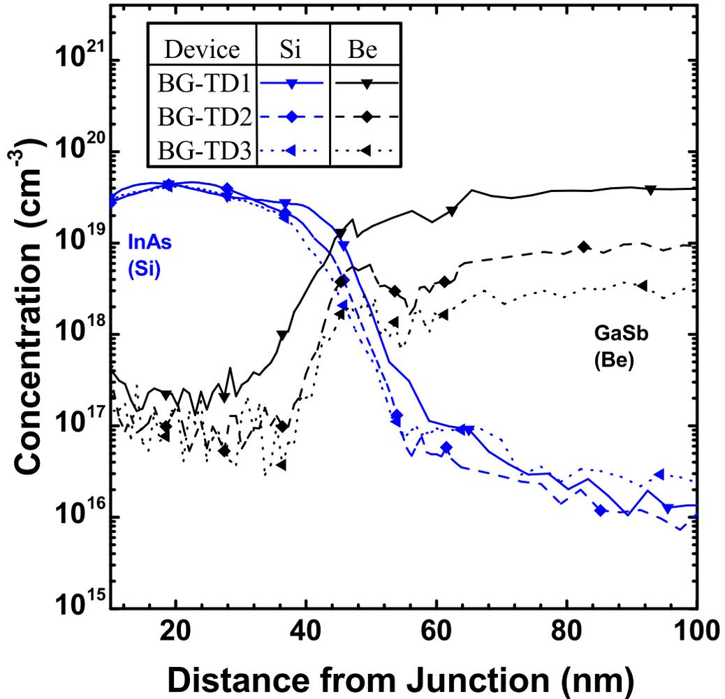
**Figure 6.5:** SIMS was performed on the samples to determine dopant levels present within the sample. BG-TD1, BG-TD2, and BG-TD3 were found to have Si and Be doping levels near the targeted values. Detectable levels of As were found to be within the GaSb film region.
