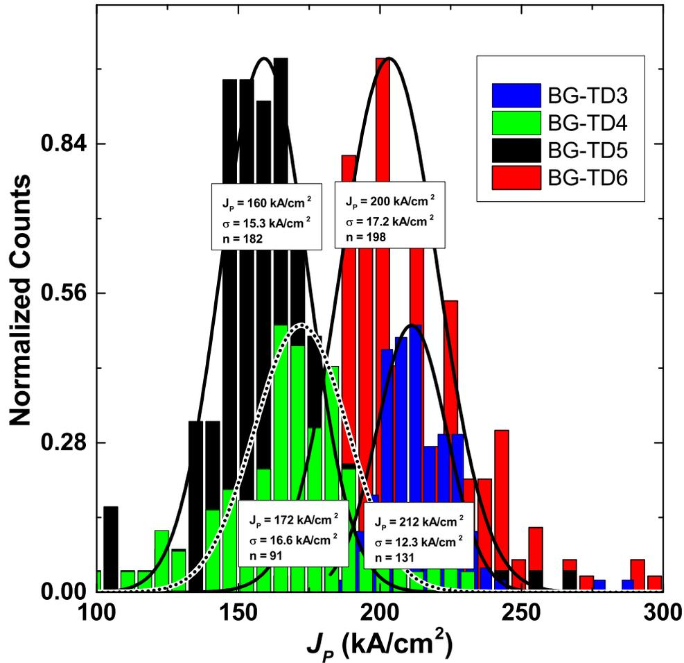
**Figure 6.18:** Normalized  $J_P$  histograms for InAs  $i$ -layer study showing the effect of InAs thickness on  $J_P$ . As expected, decreasing the  $i$ -layer thickness causes an increase in  $J_P$ . Confounding the results are the values from BG-TD3 and BG-TD5, which both have a 3 nm  $i$ -layer but is likely related to growth system drift.
