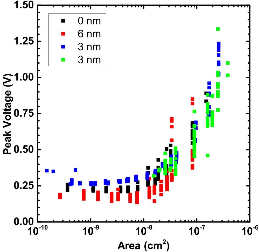
**Figure 6.17:** Typical minimum  $V_P$  values for the InAs  $i$ -layer devices appear to fall between 0.3 V and 0.2 V, indicating minimal influence from  $R_S$ .
