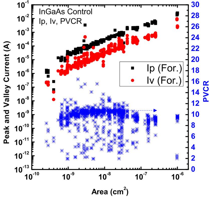
**Figure 7.8:**  $J_V$ ,  $J_P$ , and PVCRC values for InP-TD1 are plotted against device area. Current scales with area and 10.6 is the approximate value of PVCRC. Low PVCRC values indicate a rise in  $J_V$  which are associated with defects and yield issues.
