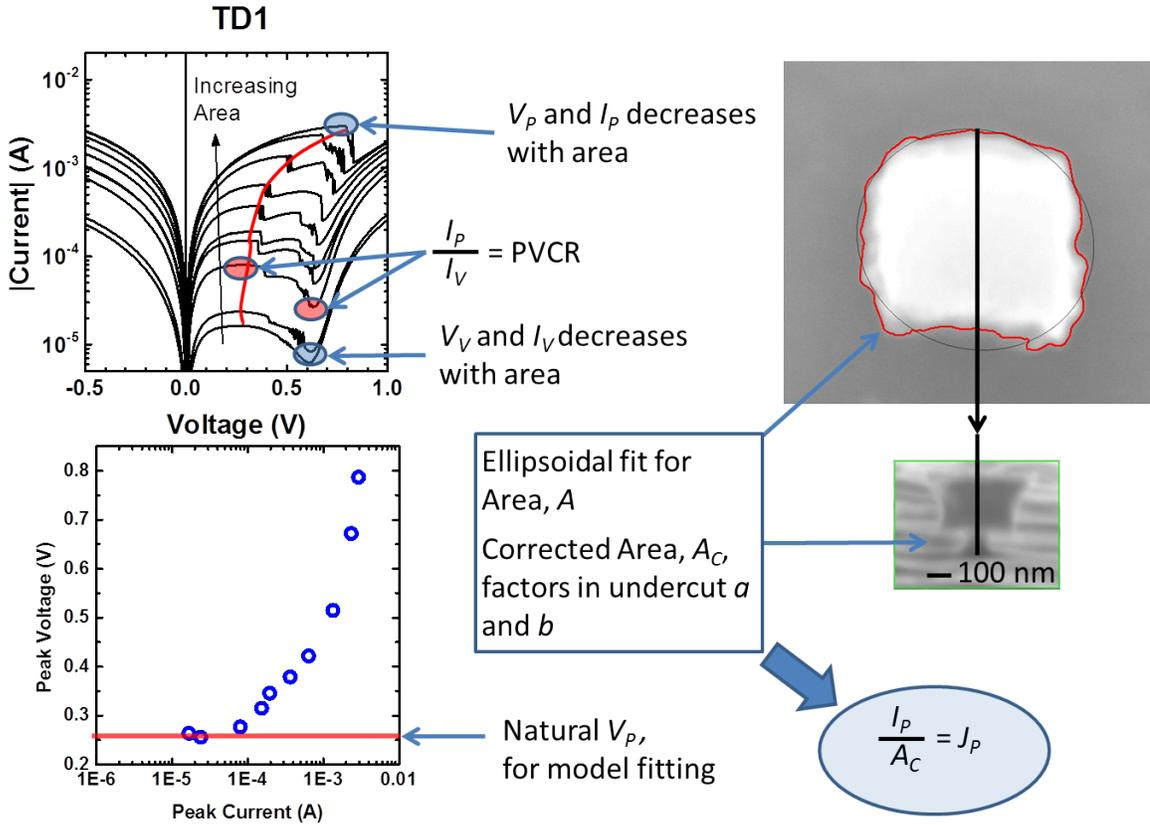
**Figure 2.7:** Utilizing sample SSG-TD1 as an example, key concepts for understanding Esaki diodes are shown above. a.  $I$ - $V$  characteristics for SSG-TD1 as devices are scaled down with area,  $I_P$ ,  $I_V$ ,  $V_P$ , and  $V_V$ , are all very apparent for each discrete device.  $R_S$  influence is reduced with area, and eventually  $V_P$  will reach a minimum value.  $J_P$  is calculated from the corrected device area and  $I_P$ . PVCR is calculated from  $I_P$  and  $I_V$
