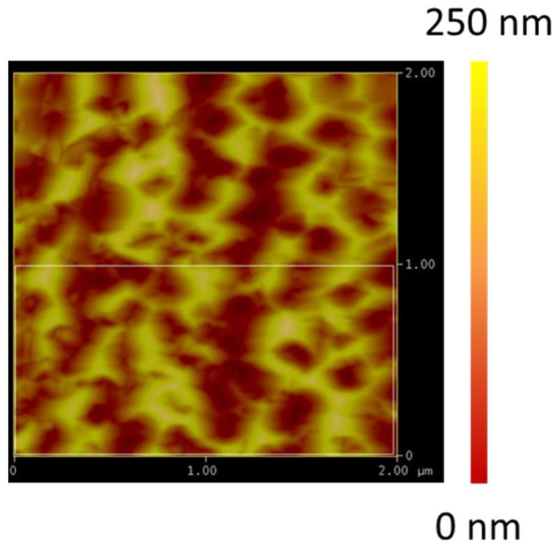
**Figure 7.13:** AFM of Si-TD3 showing an exceedingly rough surface with RMS values of 25.7 nm. This sample was not on an epi-ready ART wafer, as such, this roughness should not be considered typical for future samples that may be grown on ART, considering that lasers have been built using this technology [43, 45, 124].
