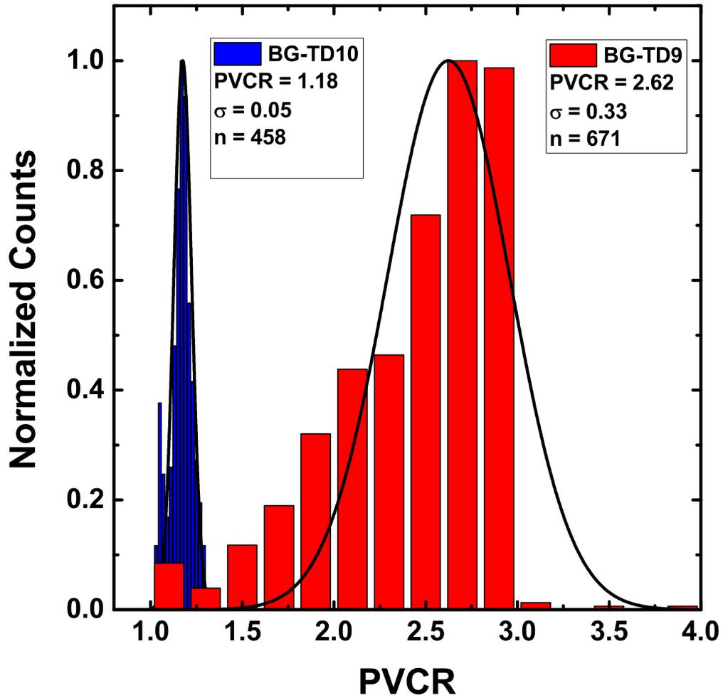
**Figure 6.36:** Normalized PVCR histograms for series 2 study showing that, after a peak value, PVCR is reduced with increased doping as has been shown in multiple other material systems.
