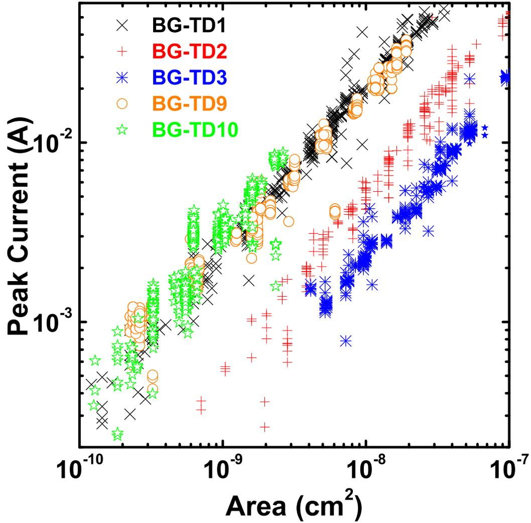
**Figure 6.37:**  $I_P$  scaled with area for the BG series 1 and series 2 diodes. The wider spread in  $I_P$  for BG-TD10 is due to the increased area variability from a two-step mesa etch process.
