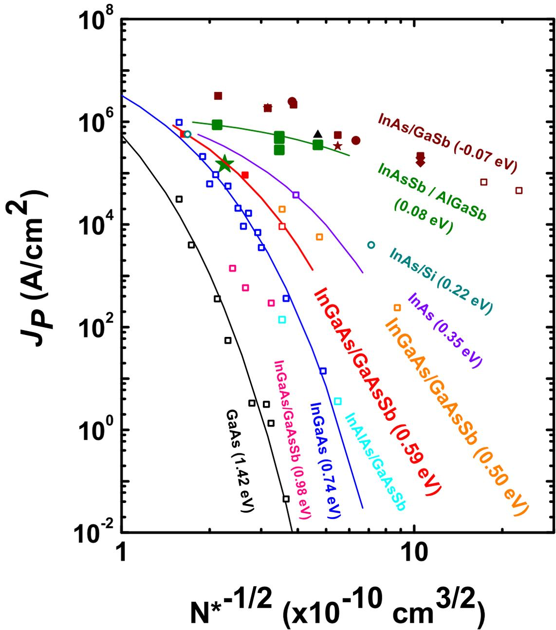
**Figure 9.1:** Final figure of merit plot with data from all samples in this dissertation overlaid with other reported tunnel diodes.
