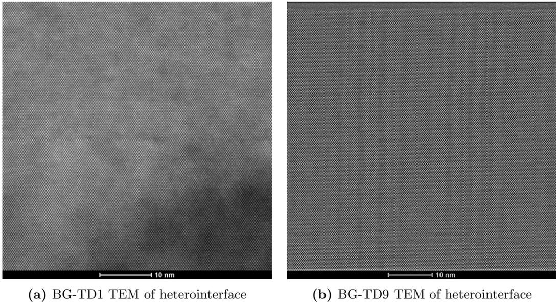
**Figure 6.41:** TEM micrographs of the heterointerfaces for both BG-TD1 and BG-TD9 exhibit no visible defects, indicating excellent crystal quality for both samples.
