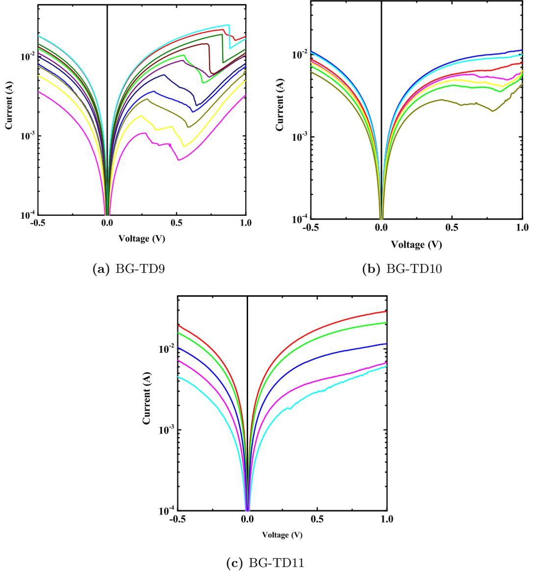
**Figure 6.31:** (a) BG-TD9 performed similarly to BG-TD1, per its design, but exhibited lower PVCR. (b) BG-TD10 generally exhibited higher  $J_P$ , but was also more difficult to measure due to  $R_S$  effects combined with the high  $J_P$ . (c) BG-TD11 exhibited some kinks in the  $I$ - $V$  characteristic, but did not show NDR at any device size. There were likely too many defects in this sample that masked the tunneling performance.
