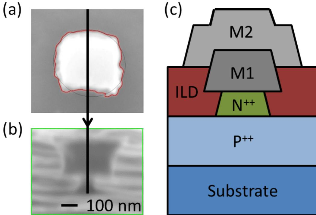
**Figure 3.11:** (a) Device areas are taken across several die to attain a representative contact area to increase the precision of the  $J_P$  and  $J_V$  data. (b) The sample is then rotated to a steep angle, often  $84^\circ$ , or higher, to measure the undercut in two perpendicular planes to account for etch anisotropy. (c) A second level metal and ILD must be used with these mesas to contact devices below  $2 \mu\text{m}$  widths
