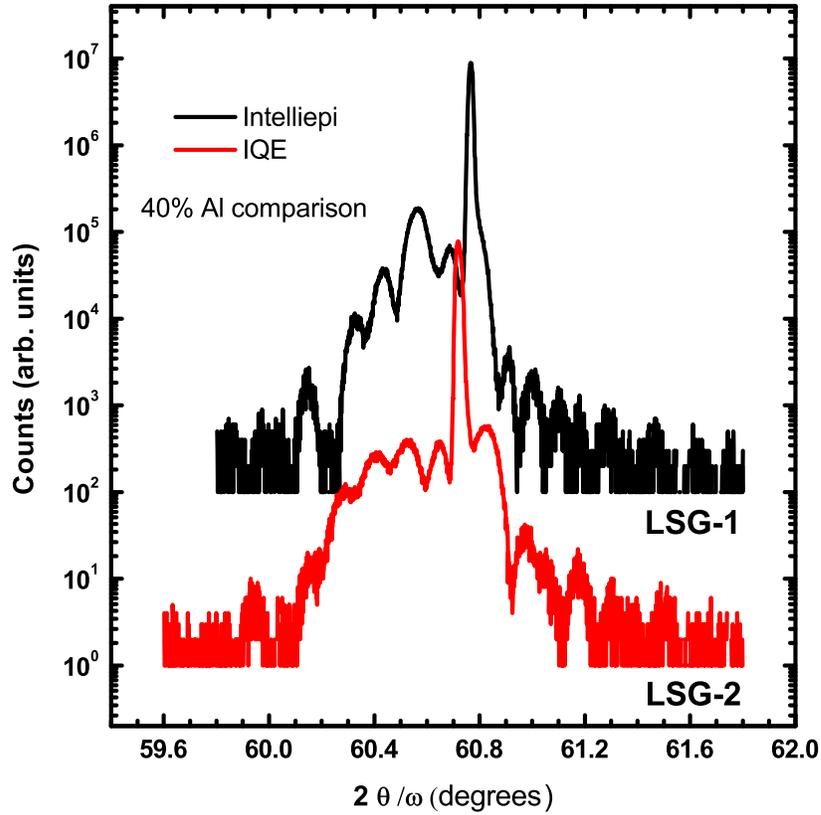
**Figure 5.10:** Comparing the  $2\theta/\omega$  profiles for LSG-1 and LSG-2, one can see some differences. Notably the substrate peak is shifted from the (400) peak location due to the  $0.35^\circ$  miss cut. LSG-1 also exhibits sharper peaks for  $\text{InAs}_{0.91}\text{Sb}_{0.09}$ , as well as more pronounced fringes, and may have a slightly lower Al content than LSG-2 due to the shoulder instead of a peak to the right of the GaSb peak.
