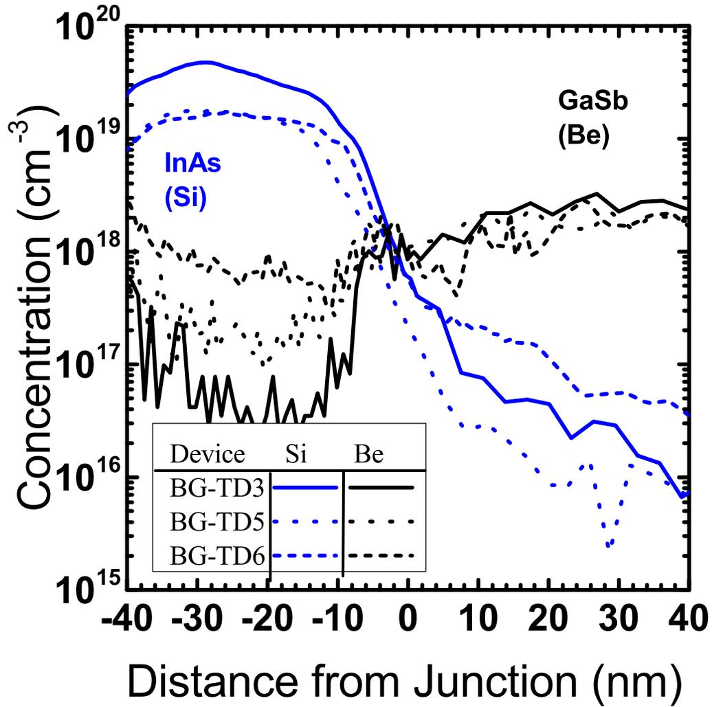
**Figure 6.14:** SIMS was performed on the samples to determine dopant levels and compare  $i$ -layer thickness.  $N^*$  values of  $2.7 \times 10^{18} \text{ cm}^{-3}$  was extracted for BG-TD3 and  $7.5 \times 10^{18} \text{ cm}^{-3}$  was extracted for BG-TD5 and BG-TD6.
