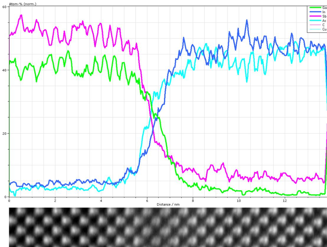
**Figure 6.43:** XPS during TEM analysis of the BG-TD9 junction shows an GaAs like interface and was found to be largely defect free.
