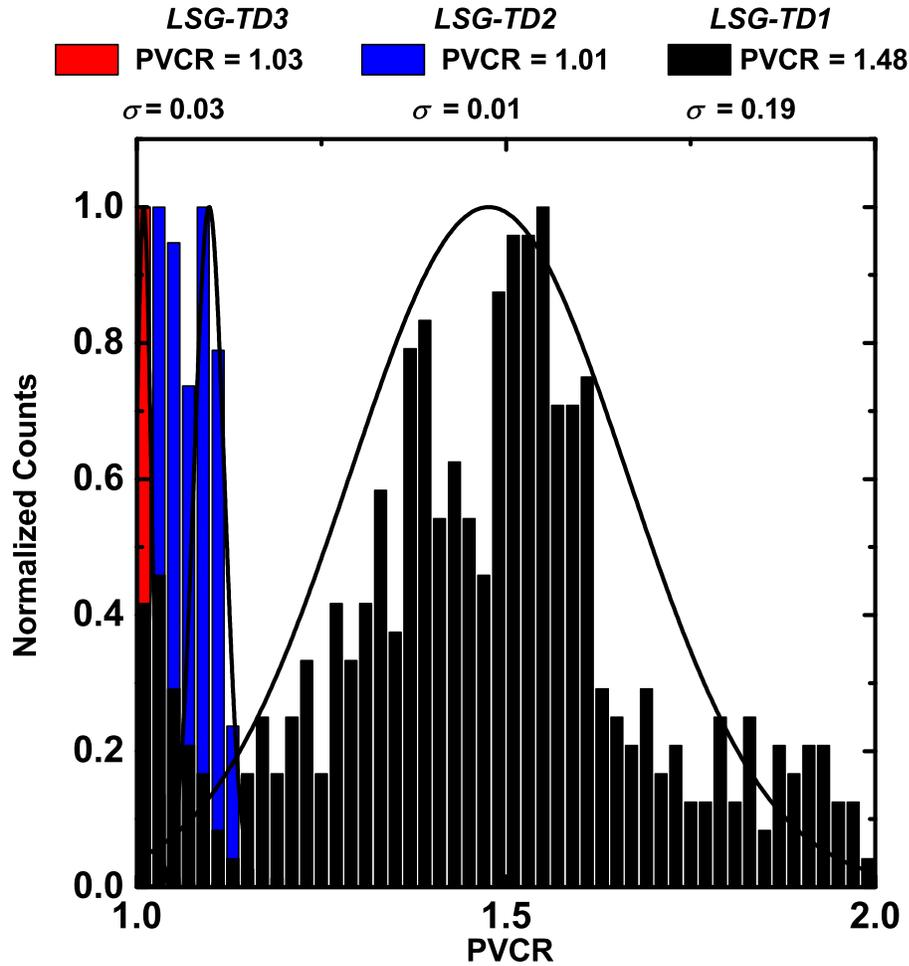
**Figure 5.7:** PVCRC values of 1.48 (LSG-TD1), 1.01 (LSG-TD2), and 1.03 (LSG-TD3) were extracted from Gaussian fits to the histogram data. LSG-1 appears to exhibit the best PVCRC performance, which may be related to the different substrate.
