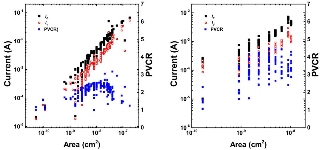
(a)  $I_p$ ,  $I_V$ , and PVCR vs. area for BG-TD2 (b)  $I_p$ ,  $I_V$ , and PVCR vs. area for BG-TD12
