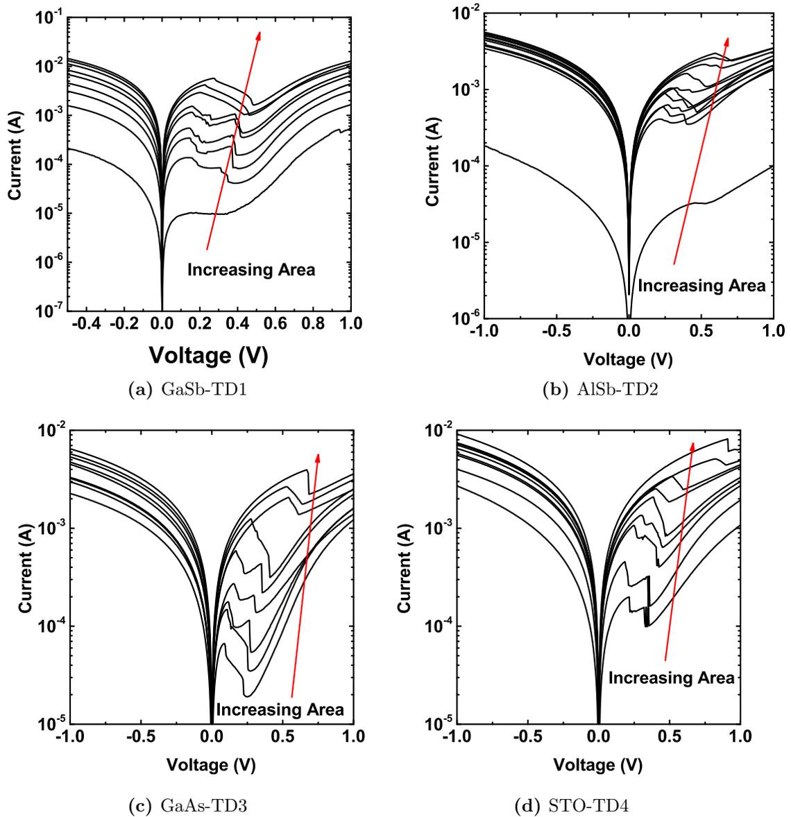
**Figure 8.4:** Representative  $I$ - $V$  characteristics for BG on Si devices with areas ranging from  $0.25 \mu\text{m}^2$  to  $4 \mu\text{m}^2$ . NDR was present at room temperature, indicating the presence of good tunnel junctions for each sample.
