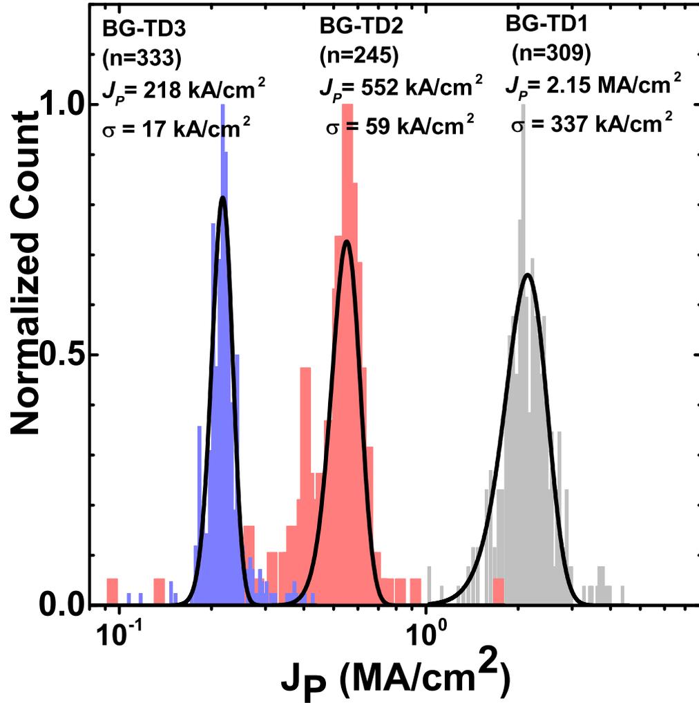
**Figure 6.10:**  $J_P$  histograms for BG series 1 diodes from which 2.2  $\text{MA/cm}^2$ , 552  $\text{kA/cm}^2$ , and 212  $\text{kA/cm}^2$   $J_P$  values were extracted for BG-TD1, BG-TD2, and BG-TD3.
