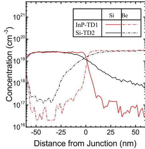
(b)  $\text{In}_{0.53}\text{Ga}_{0.47}\text{As}$  Homojunction SIMS on InP and on Si
