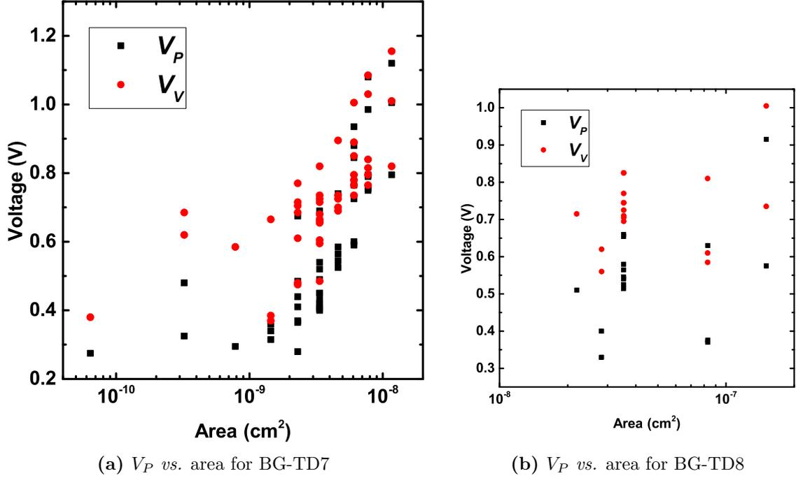
**Figure 6.24:** (a)  $V_P$  vs. area for BG-TD7 showing a  $V_P$  that should settle near 0.25 V. (b)  $V_P$  vs. area for BG-TD8 showing that is unclear where  $V_P$  should settle without additional data.  $V_P$  for both samples indicates that the samples are not limited by  $R_S$
