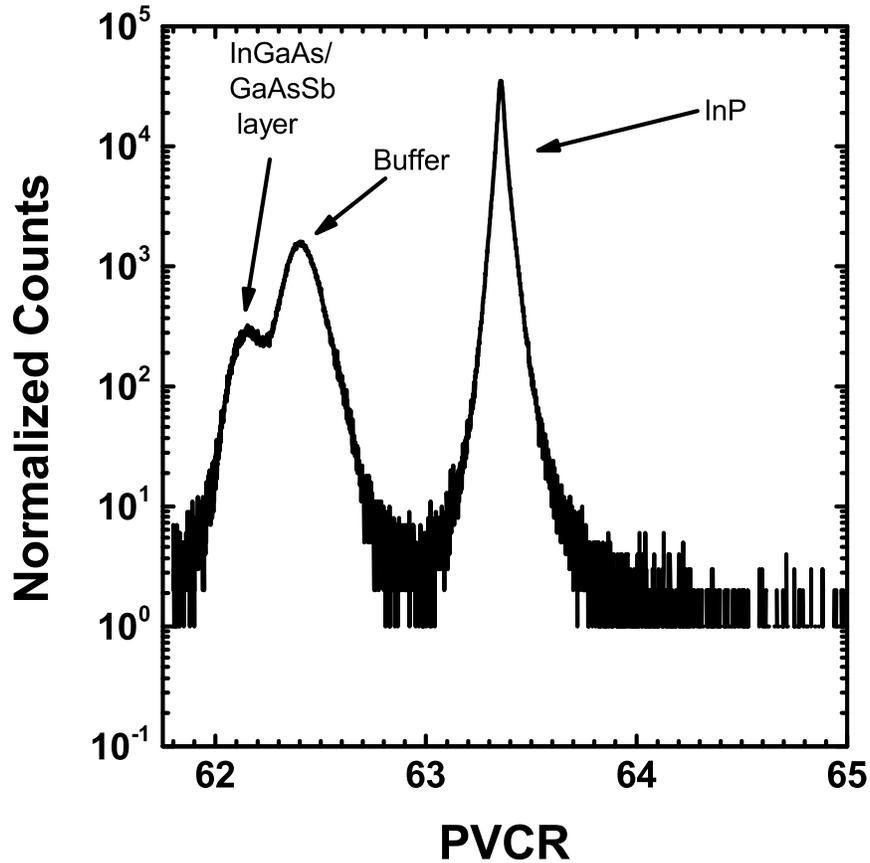
**Figure 4.10:** HRXRD for SSG-TD3 shows a fairly broad InGaAs/GaAsSb layer indicating the presence of relaxing which will adversely affect tunneling performance.
