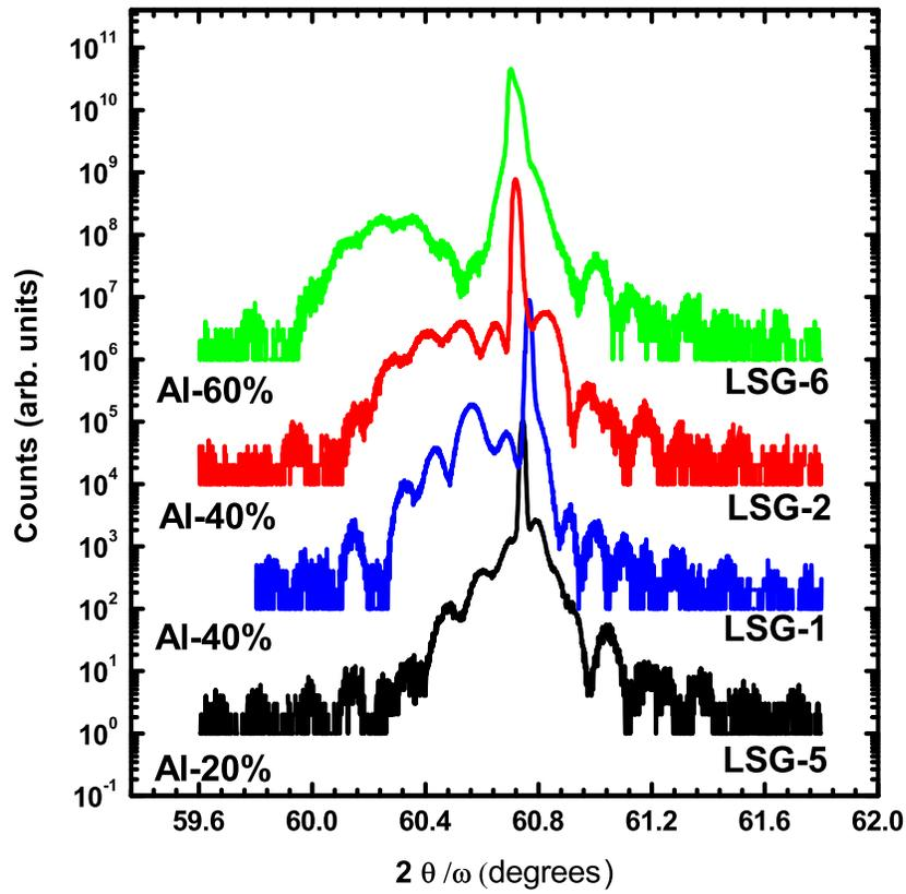
**Figure 5.18:** HRXRD of the LSG series samples. Peaks due to the Al content are shown to migrate to smaller angles commensurate with the larger lattice constant of AlSb compared to GaSb and InAs. LSG-TD6 appears to show some additional relaxation compared to the other samples, as evidenced by the broadness around the substrate peak.
