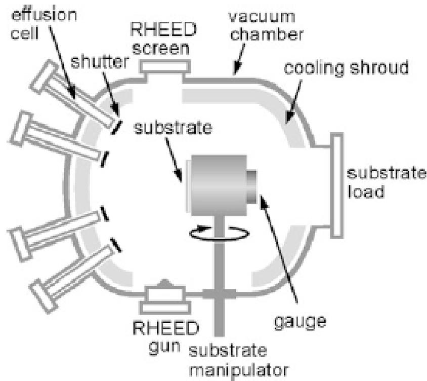
**Figure 3.1:** This schematic from Pohl [114] represents a standard MBE system. Substrates are located such that the deposition rates from the effusion cells can be calibrated to reach target composition and doping levels in the grown film.<sup>1</sup>
