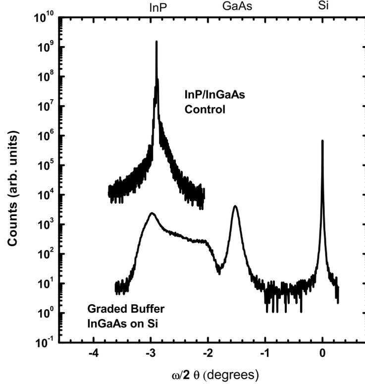
**Figure 7.5:**  $\omega/2\theta$  scan of InP-TD1 and Si-TD2, comparing the difference in peaks. Si-TD2 exhibits a broader  $\text{In}_{0.53}\text{Ga}_{0.47}\text{As}$  peak, indicating the existence of a higher defect density in the film.
