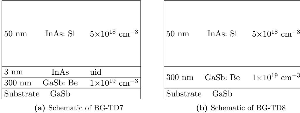
**Figure 6.21:** (a) Schematic of the film stacks for BG-TD7. This structure integrates  $\delta$ -doping into the design to push  $N^*$  higher. (b) Schematic of the film stacks for BG-TD8. This structure integrates  $\delta$ -doping into both the  $n$  and  $p$  regions to push  $N^*$  higher.
