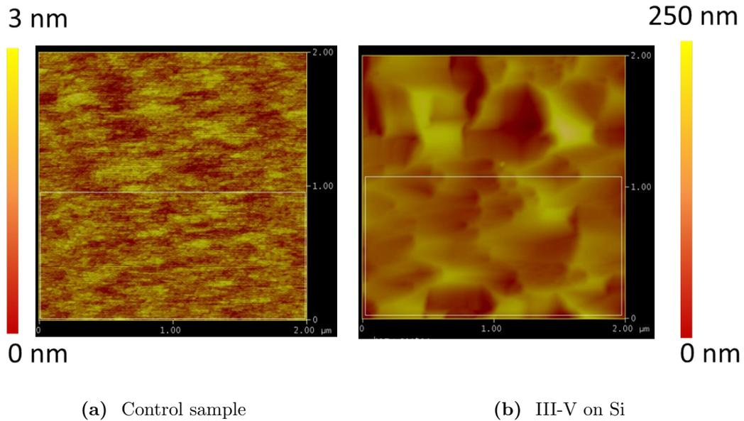
**Figure 7.3:** AFM measurements were taken from both InP-TD1 and Si-TD2. (a) InP-TD1 provided an expected smooth surface with RMS of 0.24 nm over the  $4 \mu\text{m}^2$  area. (b) Si-TD2 had regions of varying haziness, so roughness values were expected to vary across the surface, and a RMS of 14.8 was measured over the haziest region.
