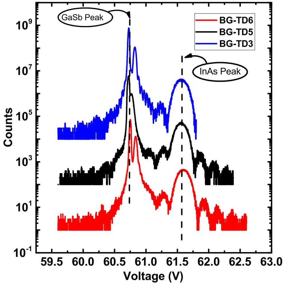
**Figure 6.13:** HRXRD of samples BG-TD5 and BG-TD6 compared against BG-TD3 show slight differences in the 300 nm film which are likely due to As remaining in the chamber following flux measurements.
