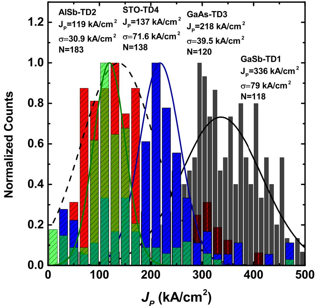
**Figure 8.7:** Normalized  $J_p$  histograms for BG on Si series showing the effect of various buffers on  $J_p$ . Varying results for  $J_p$  between the four samples may be due to the difference in thermal properties as STO-TD4 and AlSb-TD2 appear to have similar  $J_p$ , while GaSb-TD1 and GaAs-TD3 are more than double the  $J_p$  of the on Si samples.
