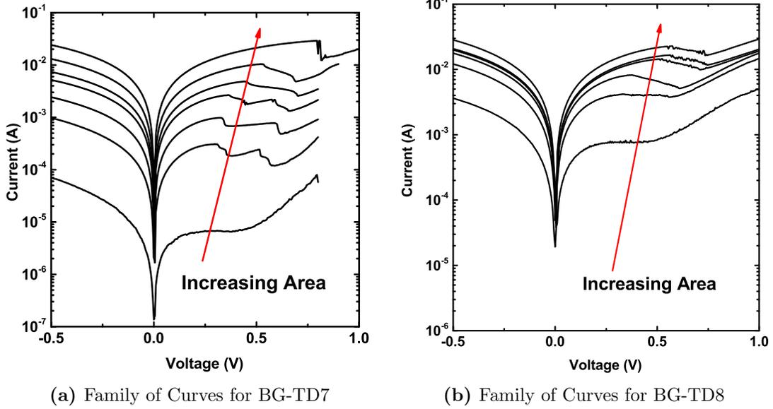
**Figure 6.22:** Family of  $I$ - $V$  curves for  $\delta$ -doped BG series. L2 metal was required to get samples to show NDR, indicating a current density over  $100 \text{ kA/cm}^2$  for the  $\delta$ -doped samples.
