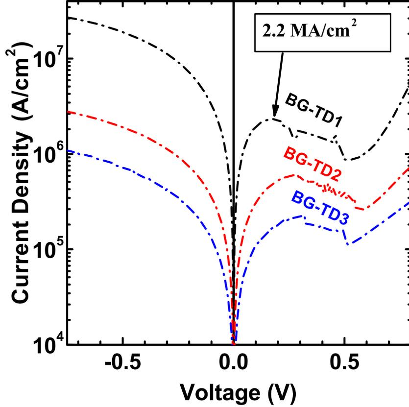
**Figure 6.9:** Representative  $I$ - $V$  curves for similarly sized devices from the BG Series 1 diodes.
