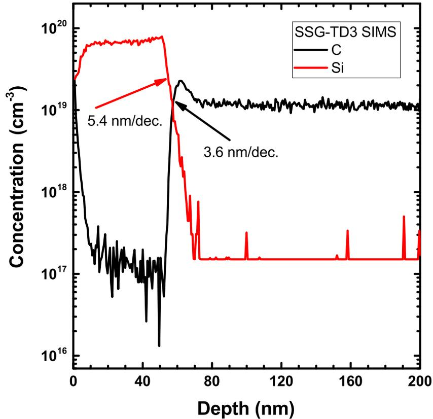
**Figure 4.9:** SIMS for SSG-TD3 exhibits steep dopant slopes of 5.4 nm/dec. for Si and 3.6 nm/dec. for C.
