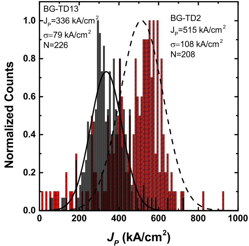
**Figure 6.48:** Normalized  $J_p$  histograms for BG  $i$ -layer series 2 study showing the effect of InAs and GaSb  $i$ -layer content on  $J_p$ . Such a large change in  $J_p$  was unexpected, as the devices are essentially the same for modeling purposes.
