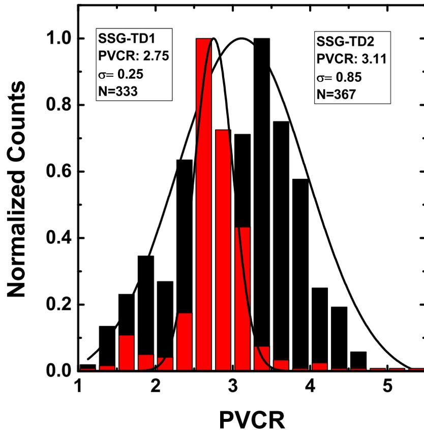
**Figure 4.4:** PVCR histogram for SSG-TD1 and SSG-TD2 showing extracted PVCR values to be 2.75 and 3.11, respectively. The distribution of values for SSG-TD1 is fairly tight, which indicates uniform performance across the wafer and few defects that would cause major changes in excess current. The broader profile of SSG-TD2 was likely process related since XRD analysis appears to show good crystallinity.
