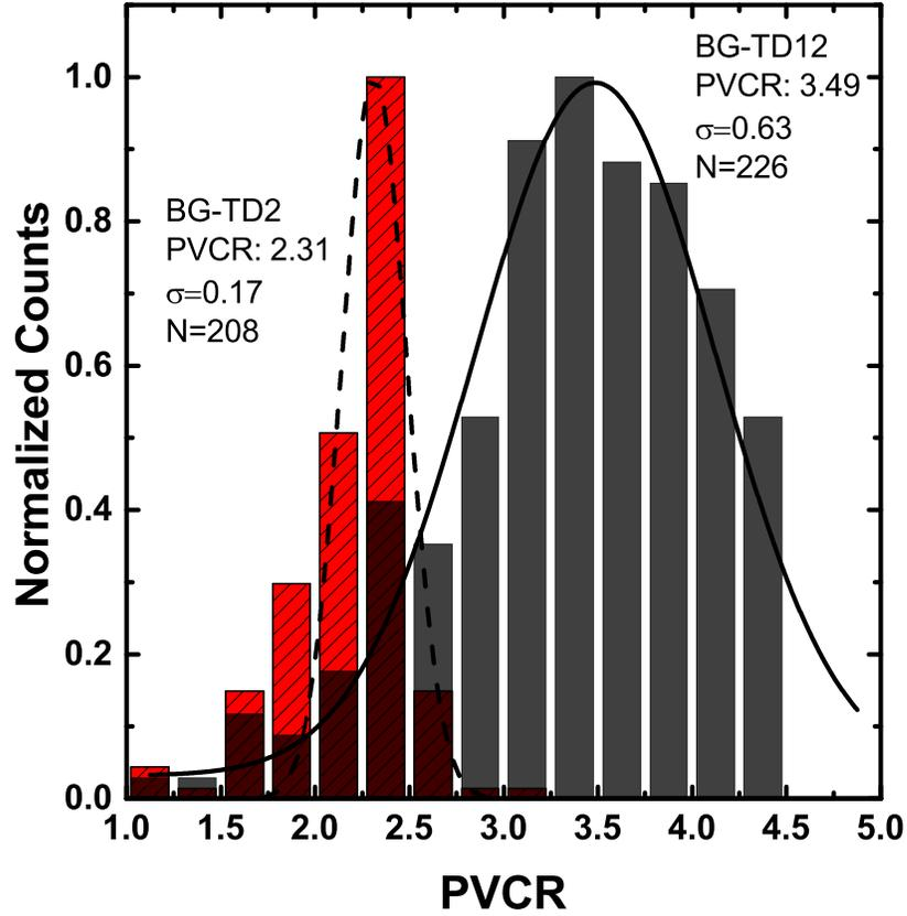
**Figure 6.49:** Normalized PVCR histograms for BG *i*-layer series 2 study showing the effect of InAs and GaSb *i*-layer content on PVCR. PVCR was expected to increase slightly, since the wider gap GaSb was expected to suppress excess current. However an increase of nearly 50% was much greater than anticipated.
