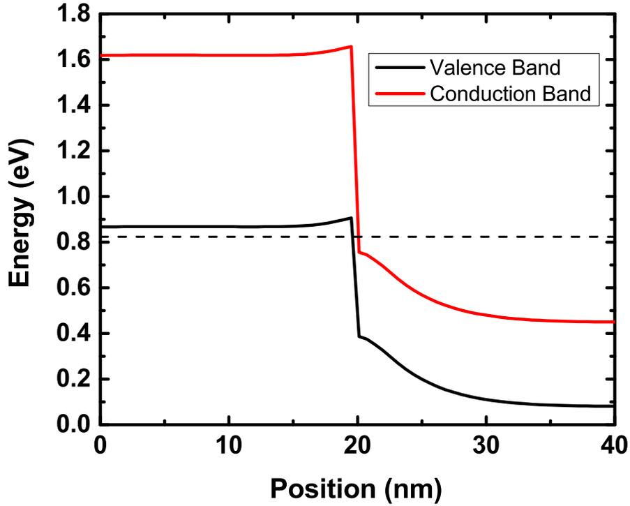
**Figure 6.1:** Band diagram courtesy of Mathieu Luisier. Type III/broken gap heterojunctions are thought to eliminate the barrier to tunneling. From above it can be seen that InAs and GaSb show a broken gap behavior, which will allow for greater tunneling currents.
