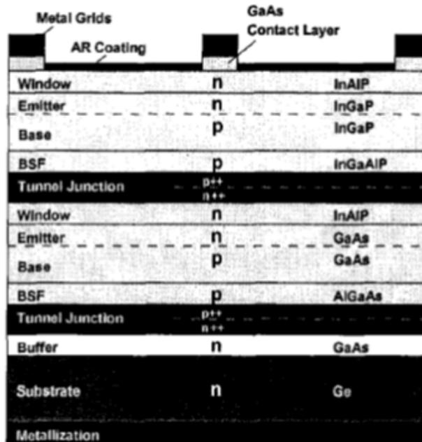
**Figure 2.11:** Example of tunnel junctions as contacts in multijunction solar cells from Miller et al. [92].<sup>1</sup>
