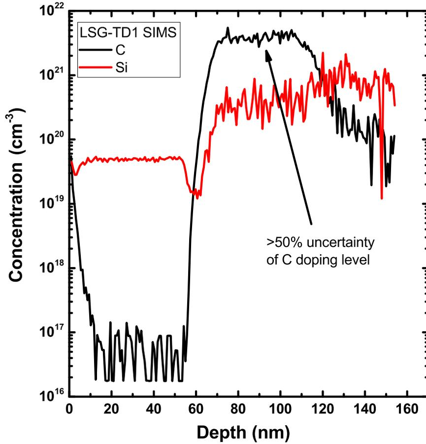
**Figure 5.12:** This SIMS plot for LSG-TD1, shows exceptionally high C levels while hitting the Si doping target. This shows an excellent junction profile, despite the uncertainty in the doping measurement.
