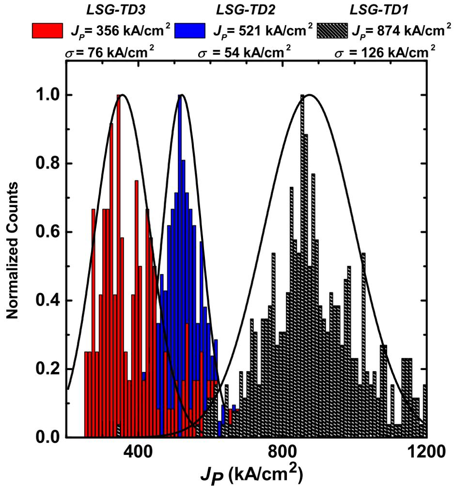
**Figure 5.6:**  $J_p$  of 874 kA/cm<sup>2</sup> was extracted from sample LSG-TD1, which was the highest reported  $J_p$  value for the InAs<sub>0.91</sub>Sb<sub>0.09</sub>/Al<sub>0.40</sub>Ga<sub>0.60</sub>Sb system reported [147]. Dopant levels for both  $p$  and  $n$ -type may be pushed higher, but reaching a 10 MA/cm<sup>2</sup> target is questionable.
