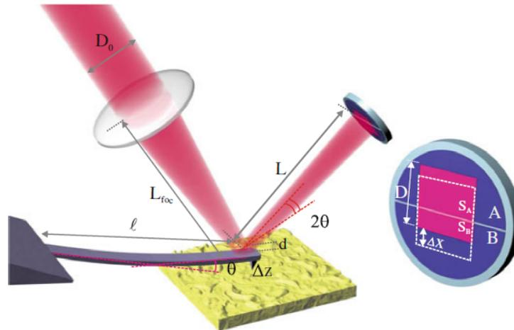
**Figure 3.10:** A schematic drawing from Voigtländer [134] exhibiting probe deflection characteristics for determining sensitivity during AFM measurements.<sup>6</sup>
