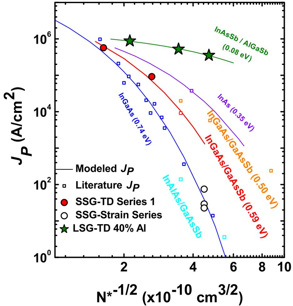
**Figure 5.11:** Figure of merit plot for the 40% Al LSG series samples with an exponential fit showing that a 10 MA/cm<sup>2</sup>  $J_P$  for this material system may not be possible.
