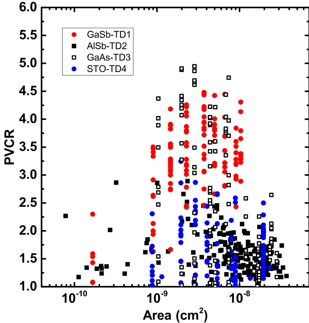
**Figure 8.6:** Devices are plotted by PVCR *vs.* area showing that PVCR tends to show maximum values prior to reaching the limits of the process control window. Both GaAs-TD3 and GaSb-TD1 show maximum PVCR around  $4 \times 10^{-9}$  cm<sup>2</sup>.
