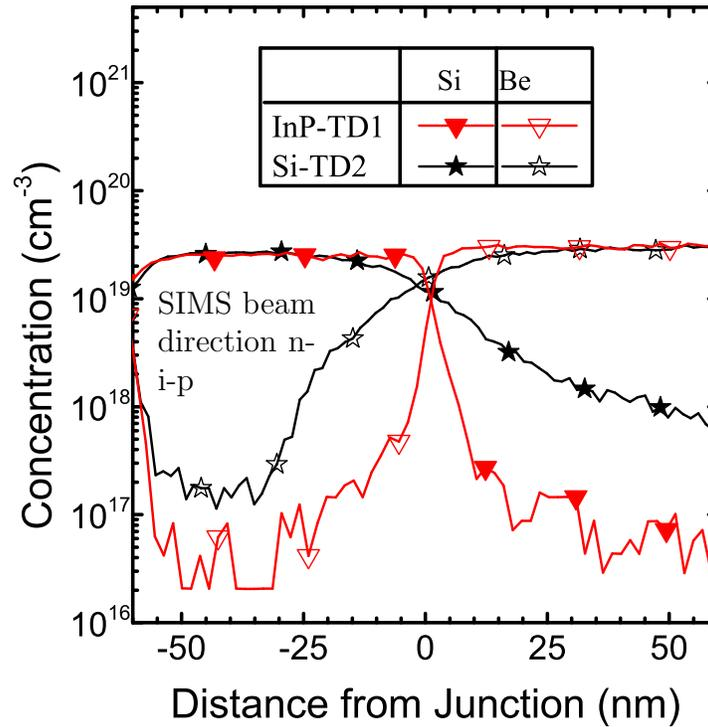
**Figure 7.4:** InP-TD1 and Si-TD2 appear to have similar doping levels. The broader slope of dopants for Si-TD2 are, presumptively, related to knock-on effects due to the roughness of the sample
