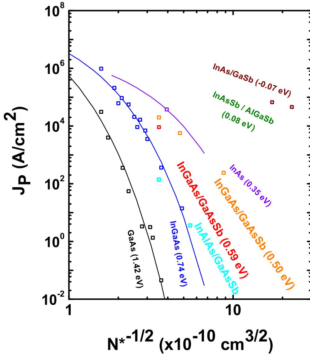
**Figure 1.3:** The state of the art prior to the work in this dissertation did not include many examples of broken or staggered gap tunnel diodes. Lack of electrical data compounds the difficulties in developing potential TFET systems.
