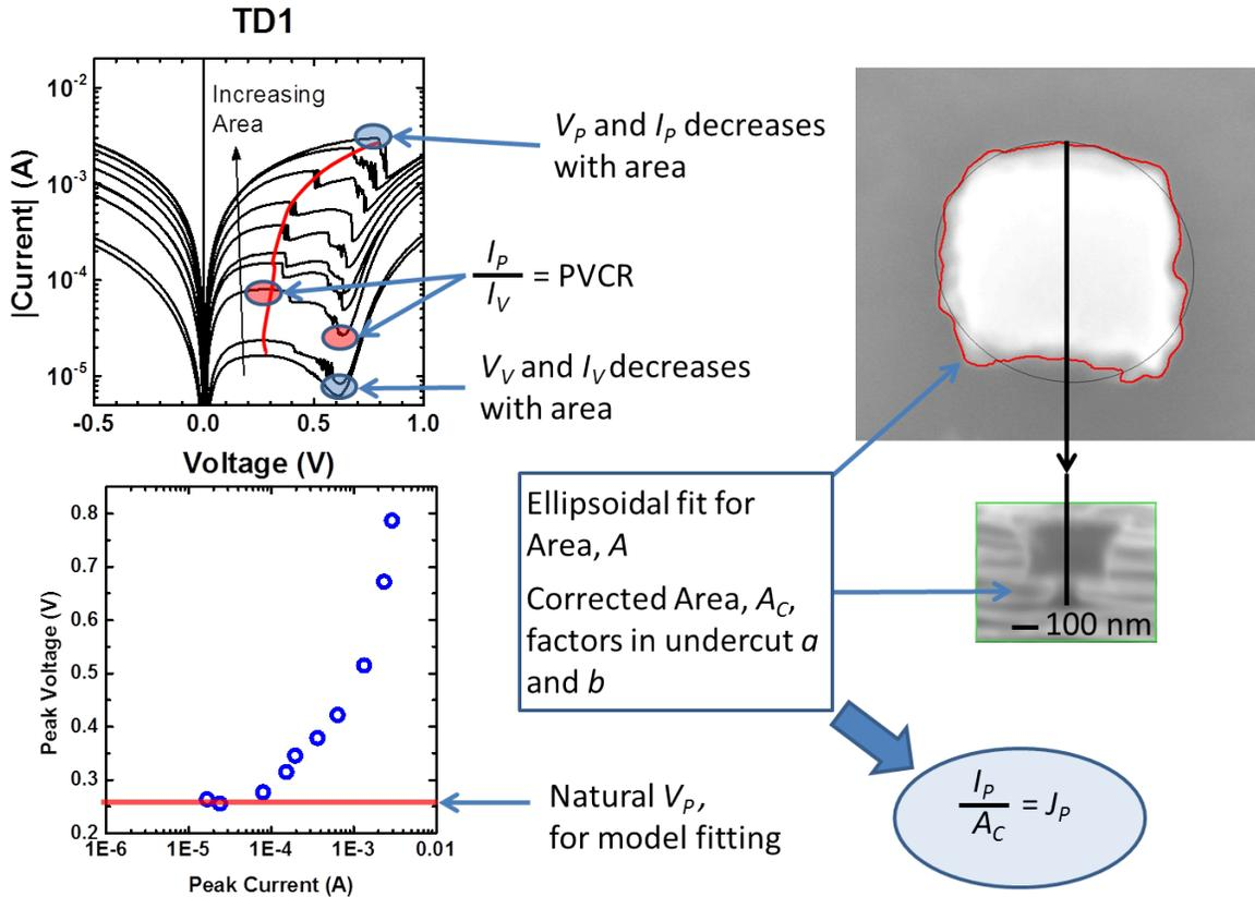
**Figure 3.12:** Utilizing sample SSG-TD1 an example, keys concepts for understanding Esaki diodes are shown above. a.  $I$ - $V$  characteristics for SSG-TD1 as devices are scaled down with area,  $I_P$ ,  $I_V$ ,  $V_P$ , and  $V_V$ , are all every apparent for each discrete device.  $R_S$  influence is reduced with area, and eventually  $V_P$  will reach a minimum value.  $J_P$  is calculated by dividing  $I_P$  by the corrected device area. PVCR is calculated from  $I_P$  and  $I_V$
