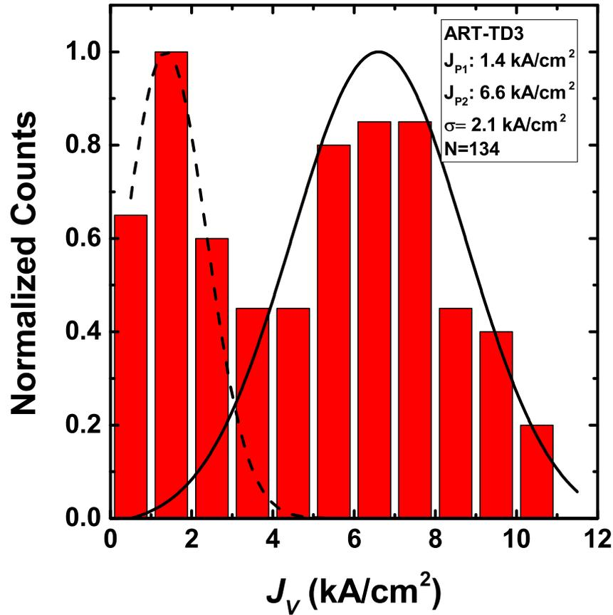
**Figure 7.16:** Histogram of  $J_V$  for ART-TD3, which shows a higher  $J_V$  value as compared to the control and buffer layer samples due to the higher defect density.
