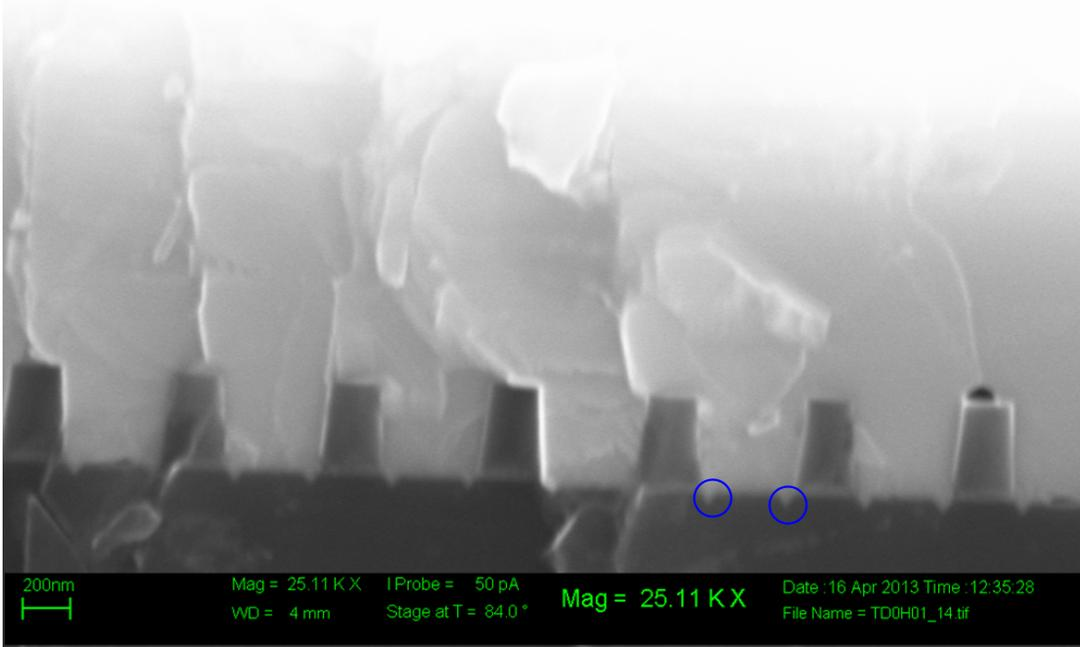
**Figure 7.12:** Sample ART-TD3 was cleaved to view the seed location in each trench. Normal samples should show a single V-groove due to the selective Si etch, these samples have a double groove indicating an incomplete groove etch which likely contributed to the epitaxy issues for the sample.
