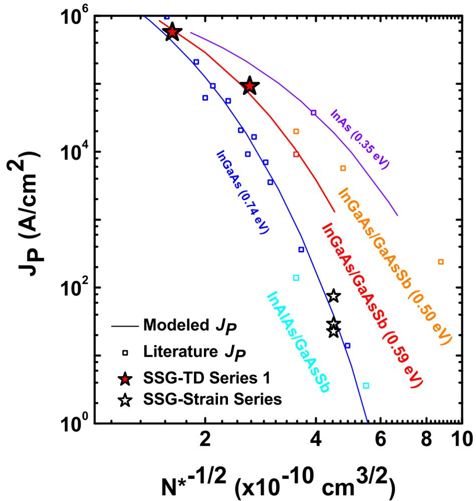
**Figure 4.17:** Figure of merit plot for the SSG series samples *vs.* other material systems [27, 54, 62] with an exponential fit showing that a 10 MA/cm<sup>2</sup>  $J_P$  for this material system may not be possible before dopant activation becomes a serious concern.
