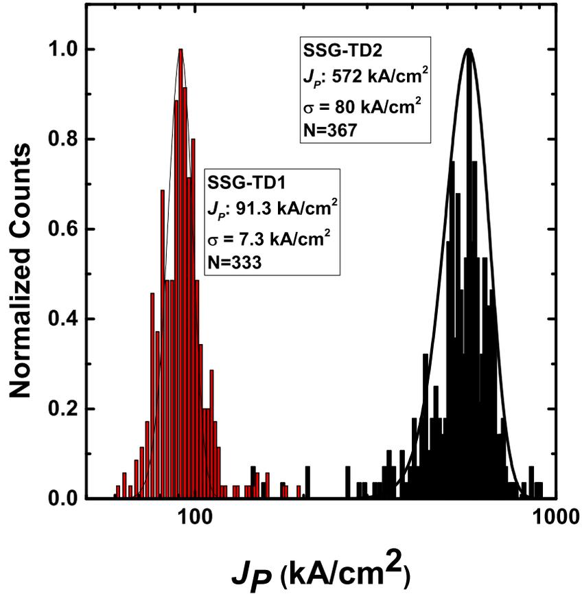
**Figure 4.5:**  $J_p$  histogram for SSG-TD1 and SSG-TD2 showing extracted values to be  $91.3 \text{ kA/cm}^2$  and  $572 \text{ kA/cm}^2$ , respectively.  $\sigma$  values are between 5% and 15%, indicating that area variation between devices is likely higher than the fitted value on SSG-TD2. Though doping levels may be pushed higher, it is unlikely that exceeding  $1 \times 10^{20} \text{ cm}^{-3}$  for both dopants could reach a  $10 \text{ MA/cm}^2$   $J_p$  target.
