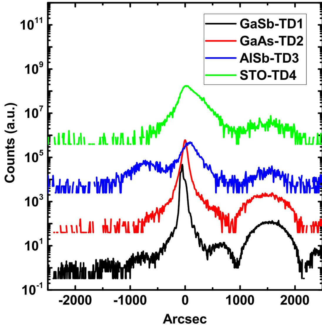
**Figure 8.2:** HRXRD of BG on Si series samples which have been aligned to the GaSb peak. Differences between the on buffer samples and control appear similar to those presented in Chapter 7, and will likely show decreased PVCr and  $J_P$  relative to the control.
