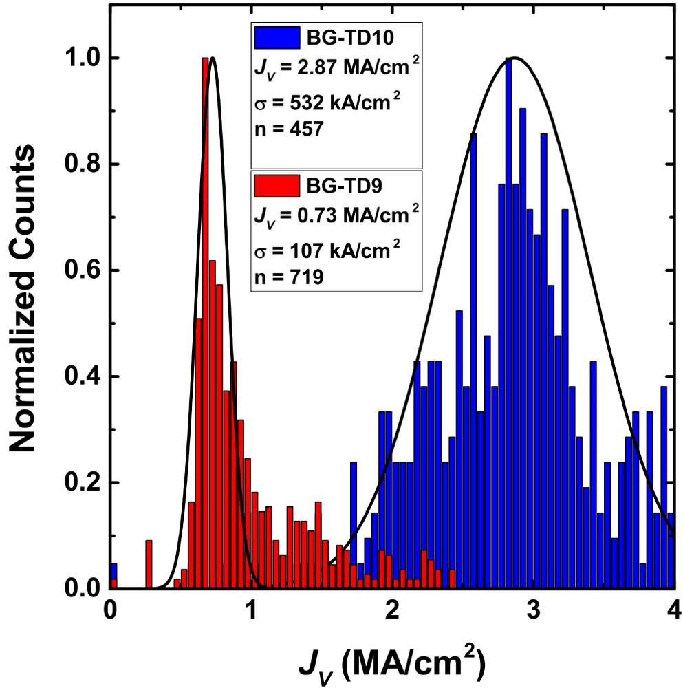
**Figure 6.35:** Normalized  $J_V$  histograms for series 2 study. BG-TD10 shows wider variation likely due to the additional processing requirements to etch into the GaSb layer.
