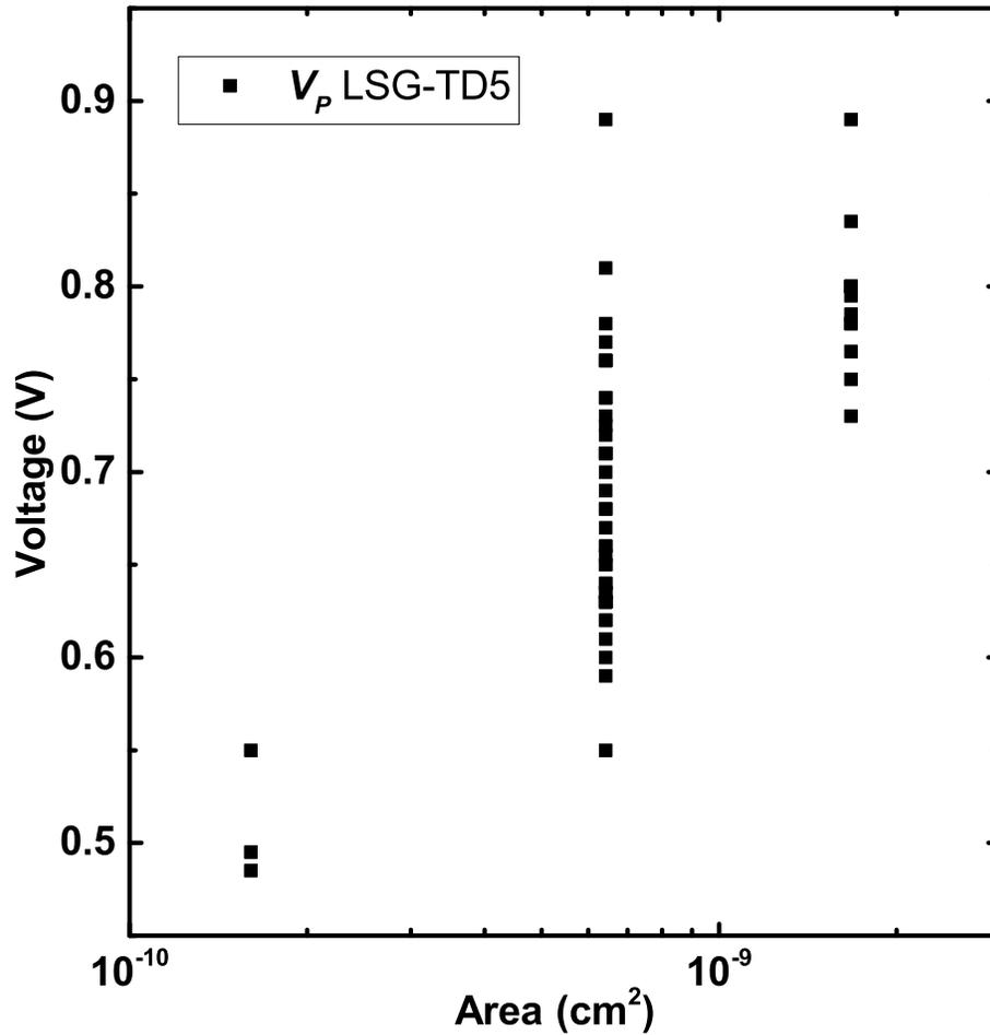
**Figure 5.15:** LSG-TD5  $V_P$  values are very large, indicating the presence of large resistance values *vs.* excess current being the source of the small PVCN values.
