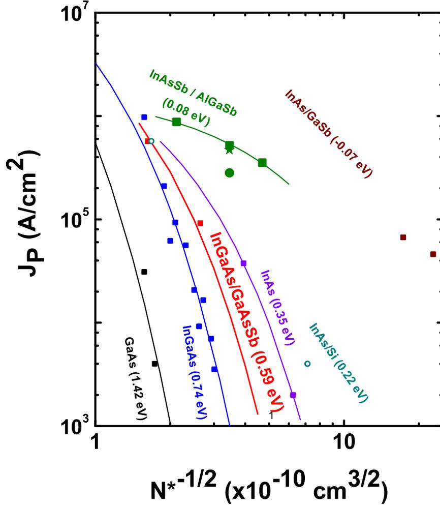
**Figure 5.19:** Figure of merit plot of the full LSG series. LSG series data exhibits a higher  $J_P$  than InAs for a given doping density which is further confirmation of the hypothesis that  $J_P$  can be increased through bandgap engineering. Notably, Al content also affected  $J_P$  indicating additional band gap engineering potential for this system.
