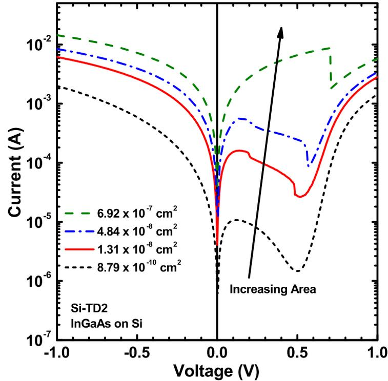
**Figure 7.7:** Representative  $I$ - $V$  characteristics for Si-TD2 device areas ranging from  $0.25 \mu\text{m}^2$  to  $100 \mu\text{m}^2$ . NDR was present at room temperature, indicating the presence of good tunnel junctions.
