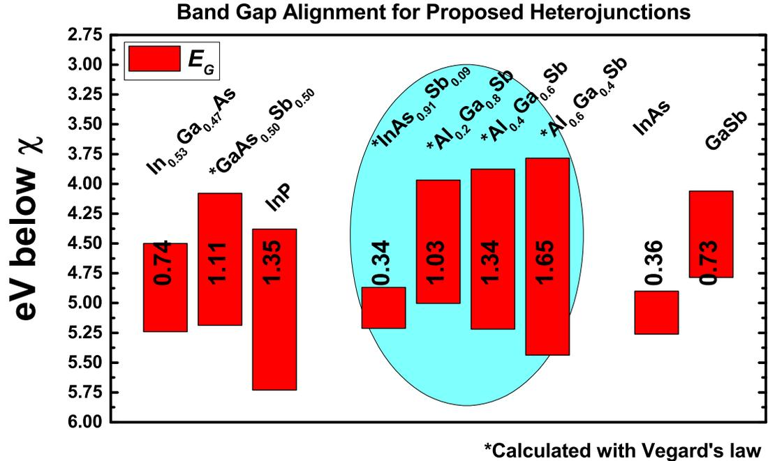
**Figure 5.1:** A relatively small decrease in the effective tunnel barrier for the SSG series resulted in significant gains in  $J_P$ , greater gains in  $J_P$  are expected for the LSG series which has a much smaller effective band gap.
