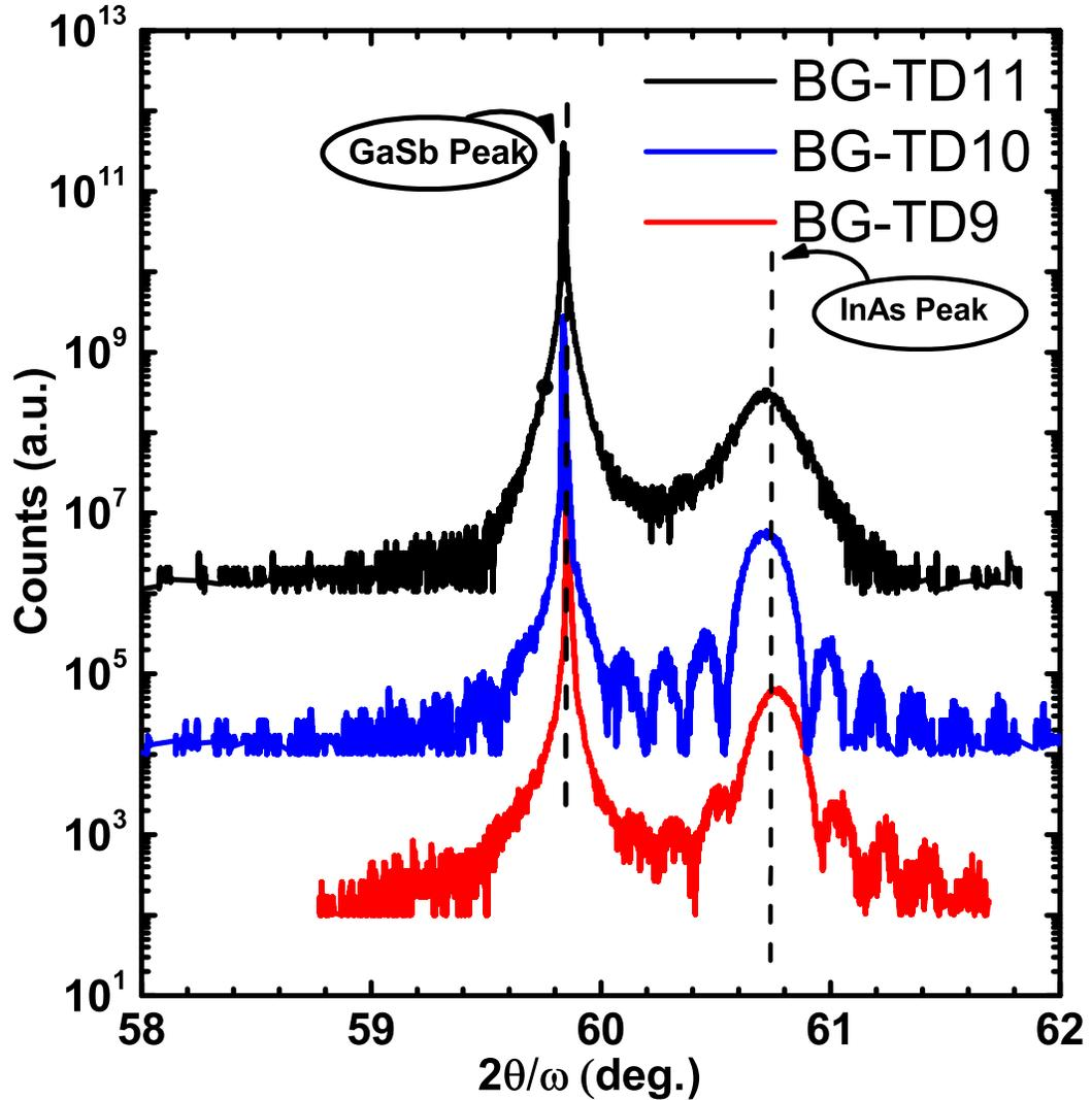
**Figure 6.29:** HRXRD information provided by the vendor show minimal relaxation for BG-TD9 and BGTD-10, while BG-TD11 appears to be fully relaxed. NDR should be expected to appear for samples BG-TD9 and BG-TD10, however the relaxation in BG-TD11 will be problematic for extracting tunneling characteristics. BG-TD11 will likely perform similarly to SSG-TD3, being highly conductive but failing to show NDR due to high defect density related excess current.
