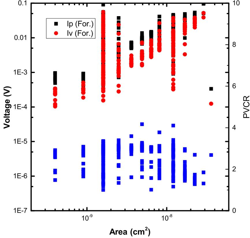
**Figure 6.8:**  $I_V$ ,  $I_P$ , and PVCR *vs.* Area for BG-TD1 shows current scaling with area and the relatively stable range for PVCR across device sizes.
