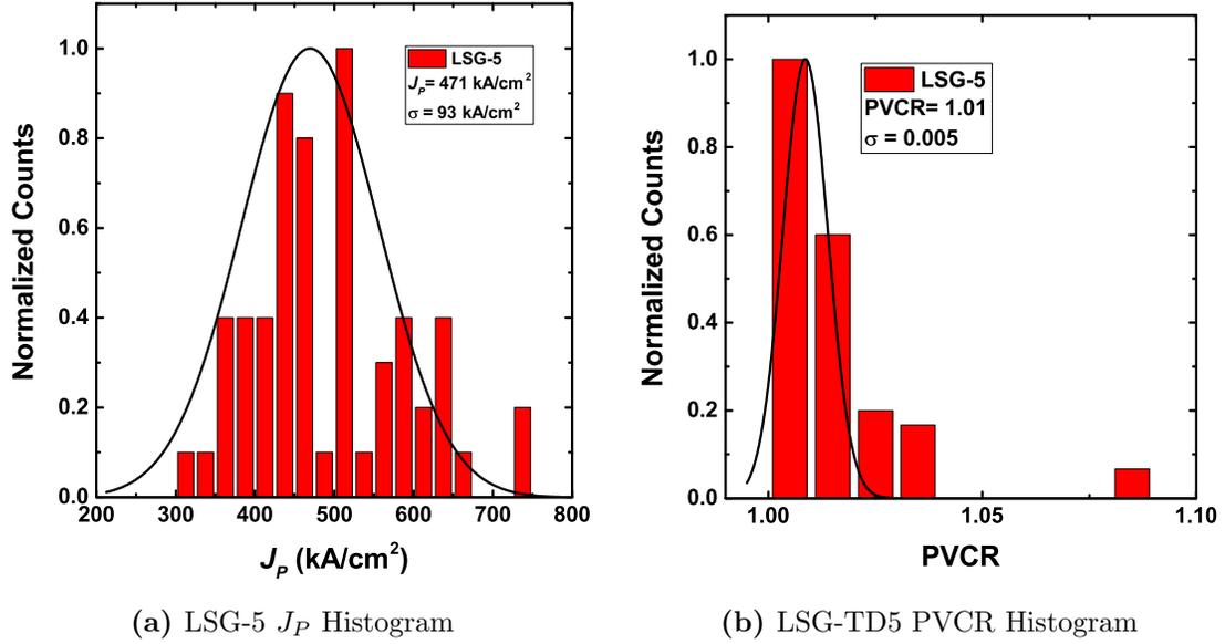
**Figure 5.16:** (a) A  $J_P$  of 471 kA/cm<sup>2</sup> was extracted from sample LSG-5, which is lower than anticipated and may be due to calibration differences between 20% and 40% Al content epitaxy at the grower. (b) A median PVCR of 1.01 was extracted from sample LSG-5, indicating significant excess currents.
