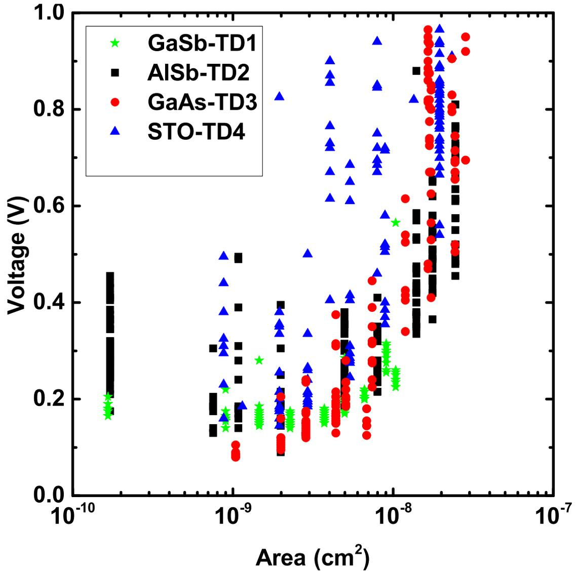
**Figure 8.8:** Typical minimum  $V_P$  values for the BG on Si devices appear to fall between 0.2 V and 0.3 V, indicating minimal influence from  $R_S$ . STO-TD4 appears to have higher  $V_P$ , likely due to variations in etch back of BCB affecting device measurements.
