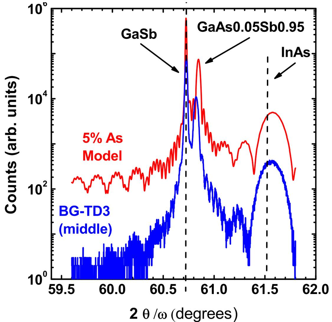
**Figure 6.4:** Assuming a 5% As incorporation into the GaSb film, LEPTOS was used to predict a  $\omega/2\theta$  curve. Interestingly, the same peak appears in simulation as was exhibited by each sample. Implying that there was As incorporated into the film.
