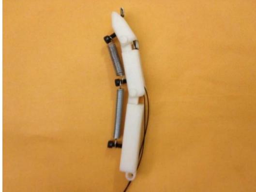
Figure 35: Finger assembly with springs and actuating tendons
