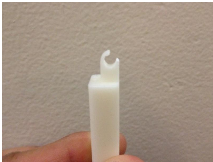
Figure 36: Fractured cross-sectional area at the joint
