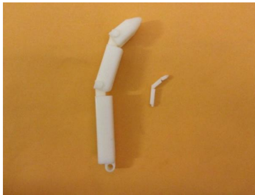
Figure 34: Rapid prototyping of finger assembly (full and \frac{1}{4} size)
