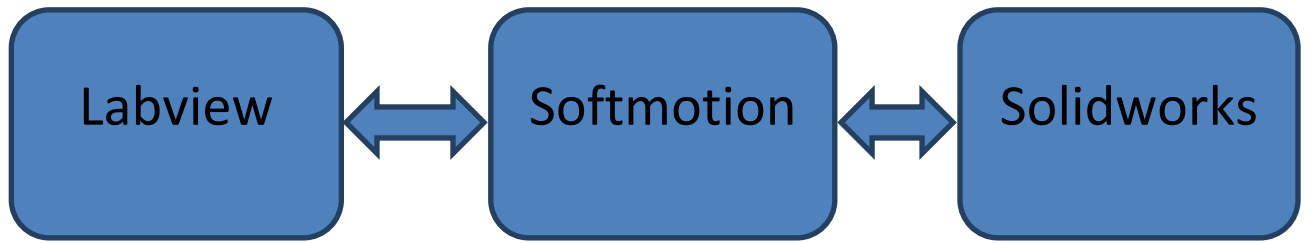
Figure 48: LabView code and Solidworks interfaced through Softmotion
