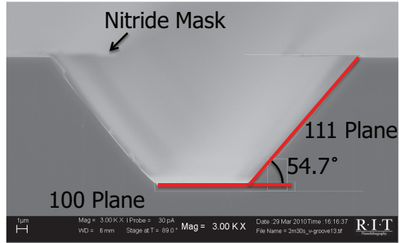
Figure 4.3: SEM image of an etched v-groove , demonstrating the crystallographic etch performed with a nitride hard mask
