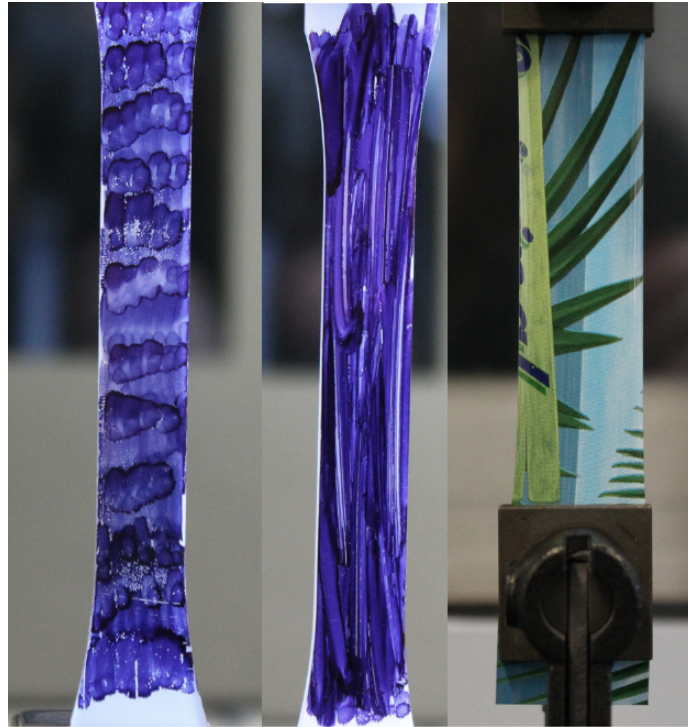
Figure 3.11: Clear speckle patterns on the specimen
