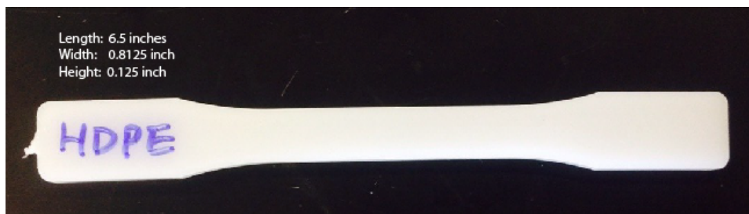
Figure 3.2: HDPE dog-bone shape specimen
