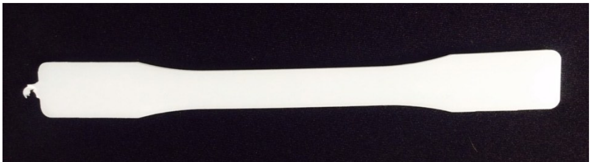
Figure 3.1 Example of Dog-Bone shaped specimen
