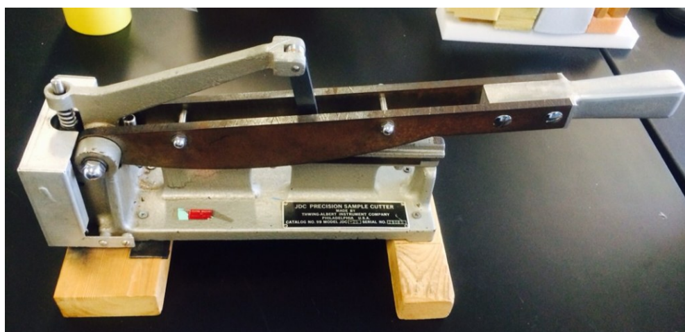
Figure 3.5: JDC Precision sample cutter
