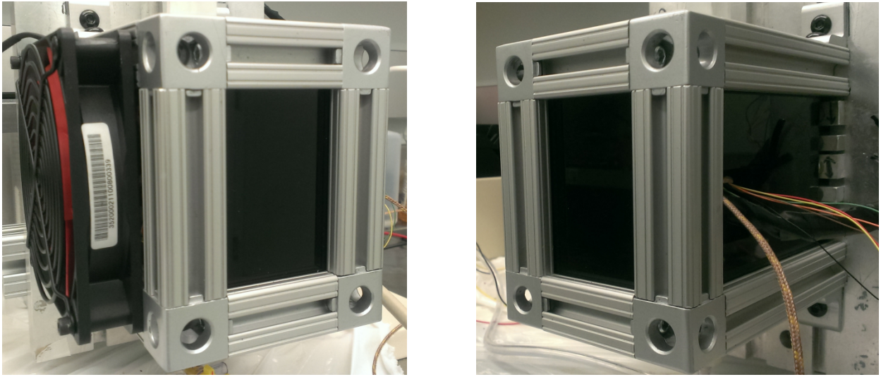
Figure 18 : Protective outer case for the shearing device
