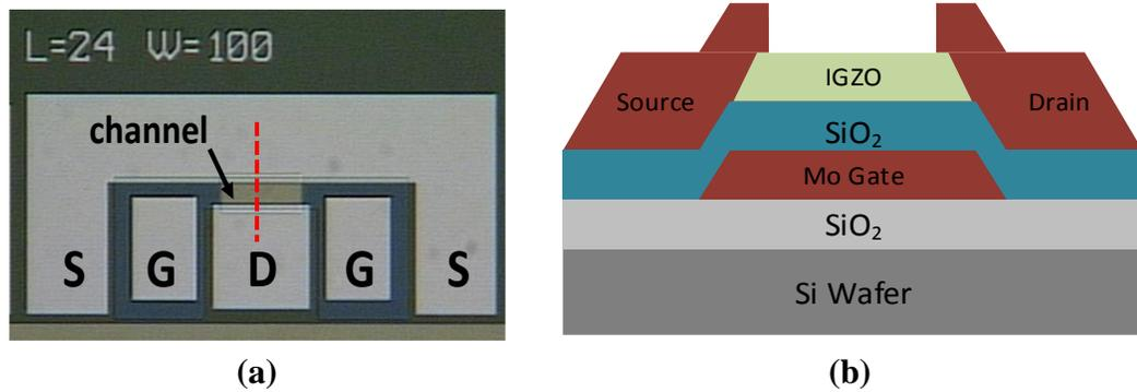
**Figure 4: (a) Micrograph of a bottom-gate IGZO TFT with source (S), gate (G), drain (D), and channel labeled with cross section along the dotted line shown in (b). The source and drain are either Mo or Al, and the channel length is 24  $\mu\text{m}$  and the channel width is 100  $\mu\text{m}$ .**
