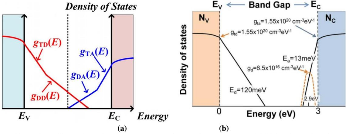
**Figure 2: (a) General density of the deep and tail states in the bandgap of IGZO [13]. (b) Density of states in the bandgap utilized in Silvaco Atlas™ simulation with a mean energy of the oxygen vacancies at 2.9 eV.**
