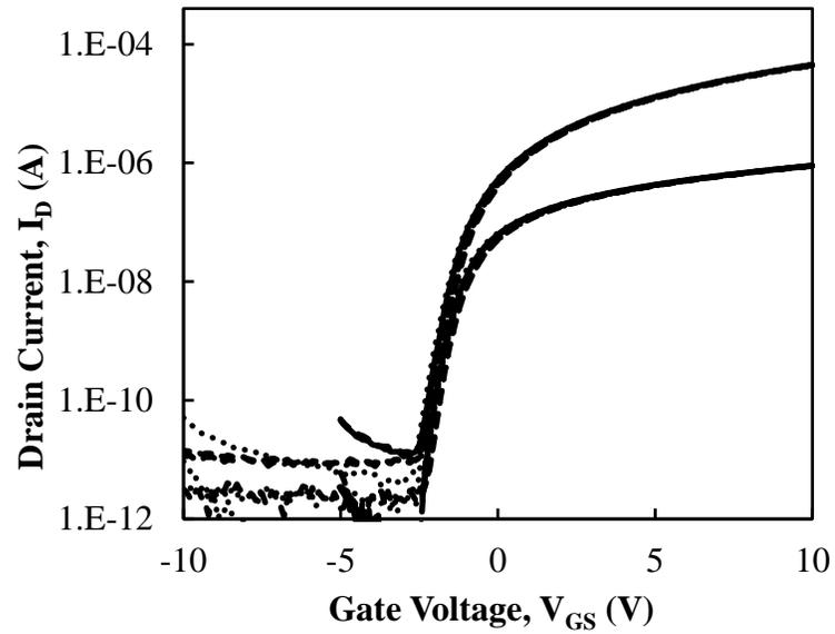
**Figure 14: Overlay transfer characteristic of a BCB passivated IGZO TFT of multiple up/down  $V_G$  sweeps with suppressed hysteresis. The dimensions are  $L = 24 \mu\text{m}$  and  $W = 100 \mu\text{m}$ .**
