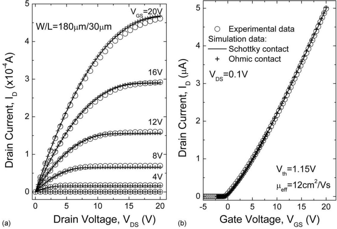
Figure 3: Overlay of the  $I_D V_G$  (a) and  $I_D V_D$  (b) characteristics of IGZO TFTs and Silvaco Atlas™ simulation with parameters defined in Table 1 [14].
