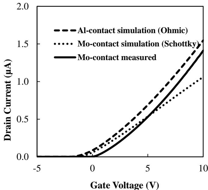
Figure 6: Overlay of a measured linear-mode ( $V_{DS} = 0.1$  V) transfer characteristic from the device shown in Figure 8 (solid line), along with simulated characteristics consistent with M-S contact conditions for Al (dashed line) and Mo (dotted line) shown in Figure 5. The TFT channel dimensions were  $L = 24$   $\mu\text{m}$  &  $W = 100$   $\mu\text{m}$ .
