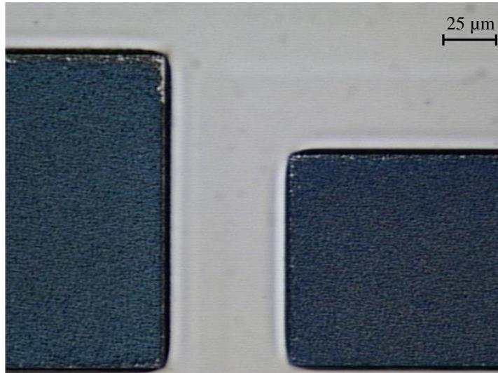
**Figure 16: Al contacts after alumina etch in 10:1 BOE**
