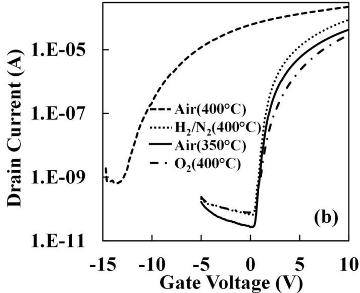
**Figure 8: Overlay of saturation-mode transfer characteristics for Mo-contact post-metal anneal treatments: Air at 350 °C for 1 h; air at 400 °C for 30 min; O<sub>2</sub> at 400 °C for 30 min; H<sub>2</sub>/N<sub>2</sub> at 400 °C for 30 min. Ramp-down conditions were in air ambient for each. The TFT channel dimensions are L =12 μm & W = 100 μm.**
