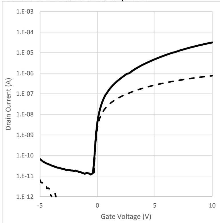
**Figure 11:**  $I_D$ - $V_G$  transfer characteristic overlays of 10 nm thick IGZO with an anneal at 400 °C for 1 hr in  $N_2$  with an  $O_2$  ramp down.
