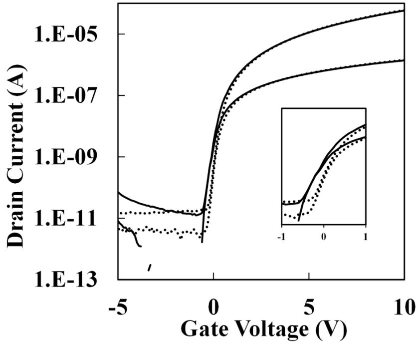
Figure 9:  $I_D$ - $V_G$  transfer characteristic overlays of Mo-contact device with a post-metal  $N_2$  anneal and air ramp-down. The inset shows up/down  $V_G$  sweep hysteresis. The TFT dimensions are  $L = 12 \mu m$  &  $W = 100 \mu m$ .
