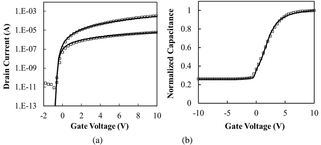
**Figure 20:** (a) Measured (markers) and simulated  $I_D$ - $V_G$  transfer characteristics of a “best-case” TFT without the application of a back-channel passivation material. The TFT channel dimensions were  $L=6\ \mu\text{m}$  &  $W=100\ \mu\text{m}$ . Model parameters and extracted properties are listed in Table I. (b) Measured (markers) and simulated C-V characteristics of an IDC with the same material model. Minor adjustments were made for structural calibration,
