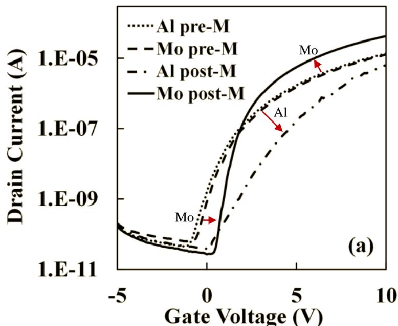
**Figure 7: Overlay of transfer characteristic for Mo-contact and Al-contact devices that either had pre-metal or post-metal air anneal at 350 °C for 1 hr. The TFT channel dimensions are  $L = 12 \mu\text{m}$  &  $W = 100 \mu\text{m}$ .**
