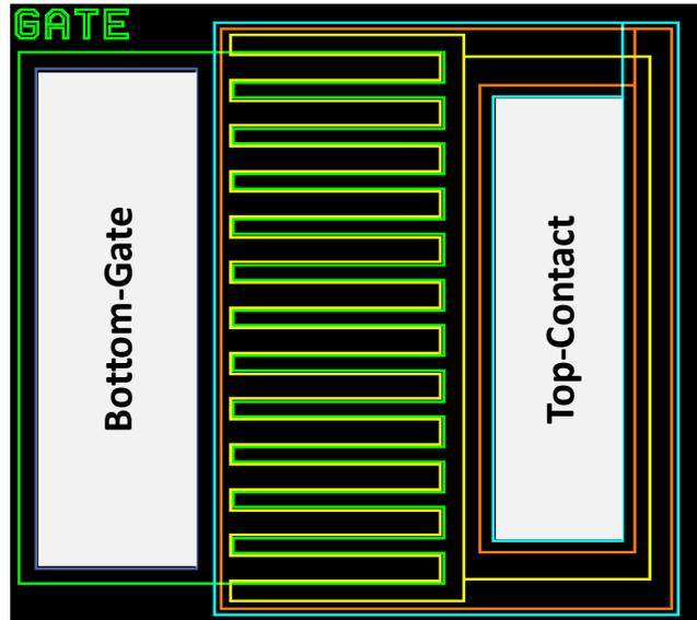
**Figure 15:** ICD layout, with twelve interdigitated fingers extending across the IGZO mesa. Each gated region has a width of  $44\ \mu\text{m}$ , and  $5\ \mu\text{m}$  side overlaps between the top-contact metal and the bottom-gate metal. The total gated area is  $\sim 0.002\ \text{cm}^2$ .
