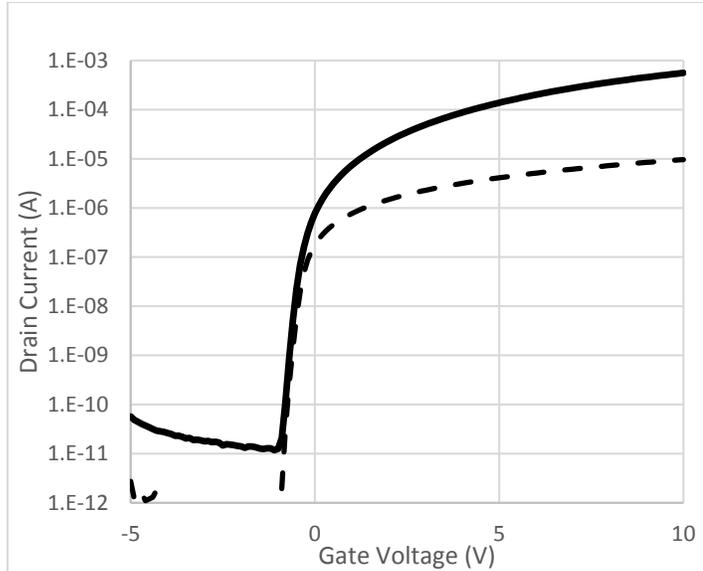
**Figure 12:  $I_D$ - $V_G$  transfer characteristic overlays of 30 nm thick IGZO with an anneal at 400 °C for 1 hr in  $N_2$  with an  $O_2$  ramp down.**
