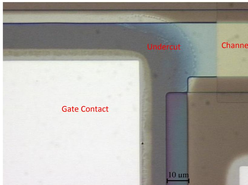
Figure 18: Undercut of the gate contacts during  $\text{Al}_2\text{O}_3$  etch.
