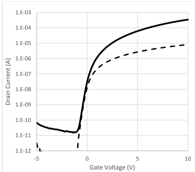
**Figure 10:**  $I_D$ - $V_G$  transfer characteristic overlays of 5 nm thick IGZO with an anneal at 400 °C for 1 hr in  $N_2$  with an  $O_2$  ramp down.
