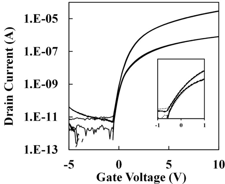
**Figure 13: Mo-contact device with alumina back-channel passivation exhibiting suppressed hysteresis over multiple up/down sweeps**
