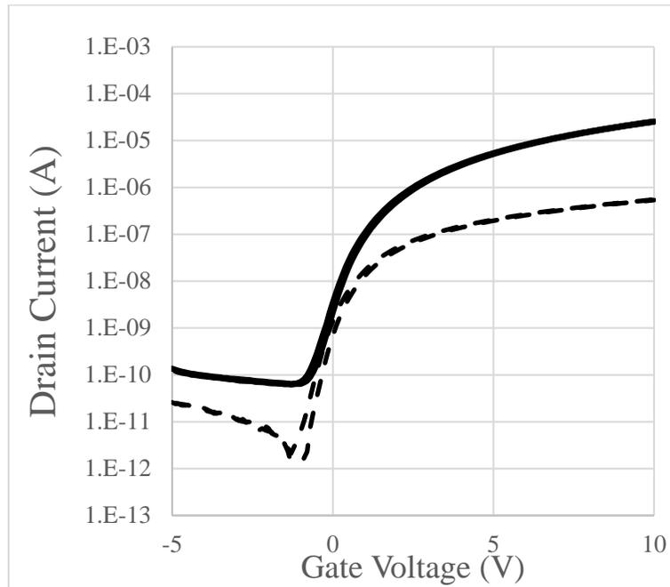
Figure 17: Overlay  $I_D$ - $V_G$  transfer characteristic of an unpassivated IGZO TFT swept up and down with hysteresis. The dimensions are  $L = 24 \mu\text{m}$  and  $W = 100 \mu\text{m}$ .
