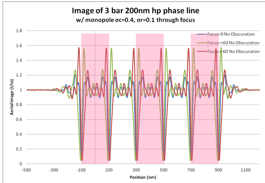
Figure 104: Aerial image of a phase shifted three bar structure with 200 nm half pitch, six \pi phase edges, imaged with a monopole with \sigma_c=0.4 , and \sigma_r=0.1 through focus
