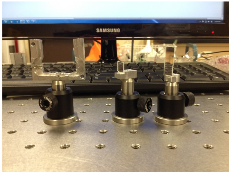
Figure 2.7 – Mirror mount 1 which held the mirror between two pieces of aluminum, Mirror mount 2 which cut and mounted mirror onto an optical post with epoxy, Mirror mount 3 which used a larger mirror and reduced the space between mirror and sample holder.
