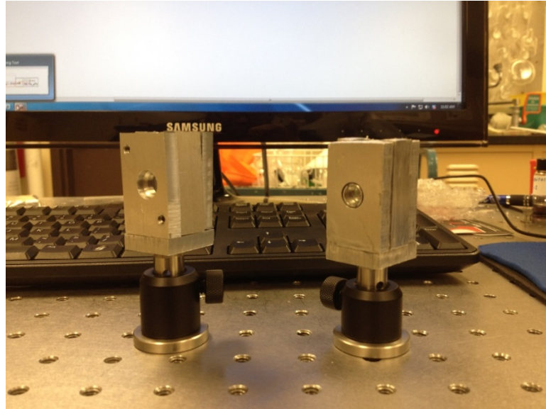
Figure 2.6 – On the right is sample holder 1 which was constructed with the ability to be broken down and connected by screws and on the left is sample holder 2 is a permanent holder that is constructed with epoxy.
