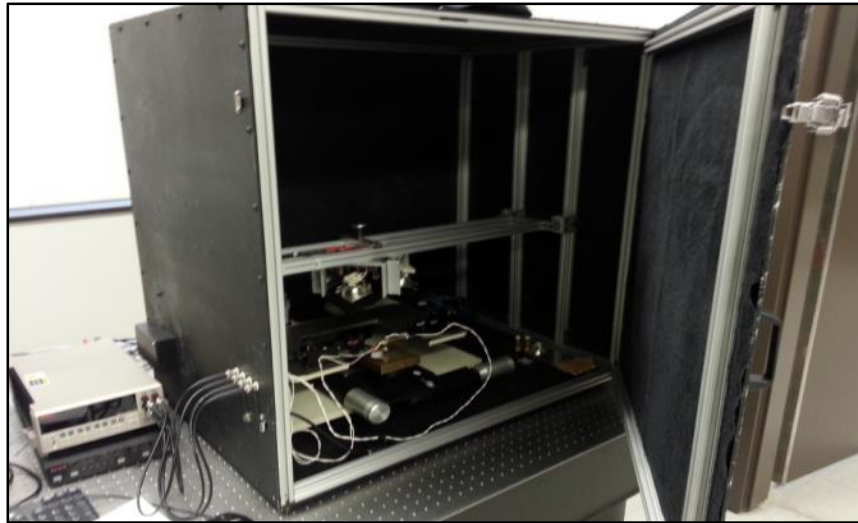
Figure 23: Setup to extract Dark I - V and I_{sc} - V_{oc}
