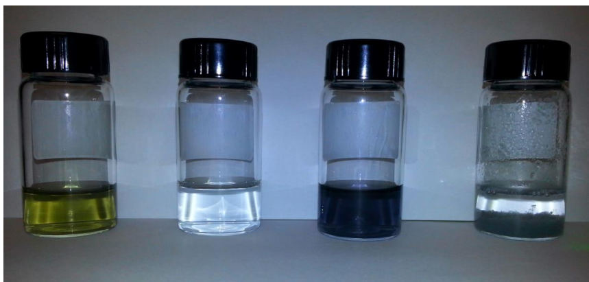
Figure 2.13 Separated metallic “yellow” and semiconducting fractions with different salts. LiCl (transparent), NaCl (purple) and KCl (grey aggregates).
