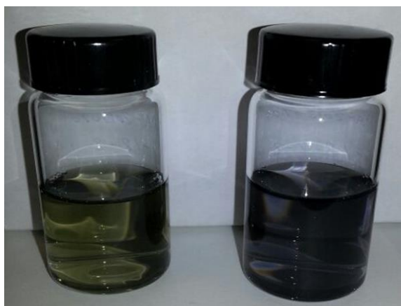
Figure 2.5 Separated metallic SWCNTs, “yellow fraction,” and semiconducting SWCNTs, “purple fraction.”
