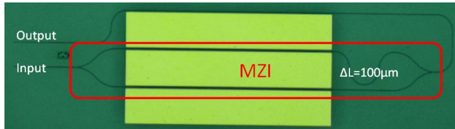
Fig. 4.9 (a). Microscope image of the hybrid Si-LiNbO 3 modulator integrated into a Mach-Zehnder interferometer. The total size of the device is only 1mm.
