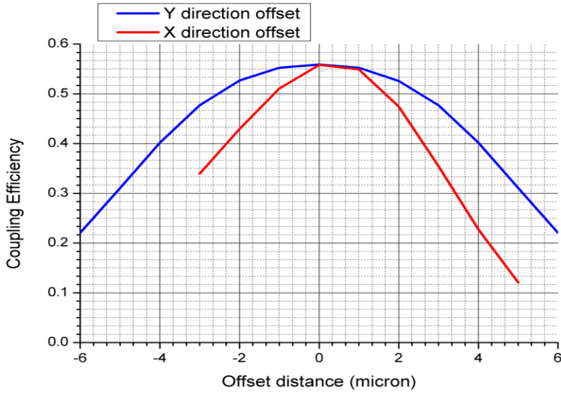
Fig. 3.36. Alignment tolerance study of focusing grating coupler
