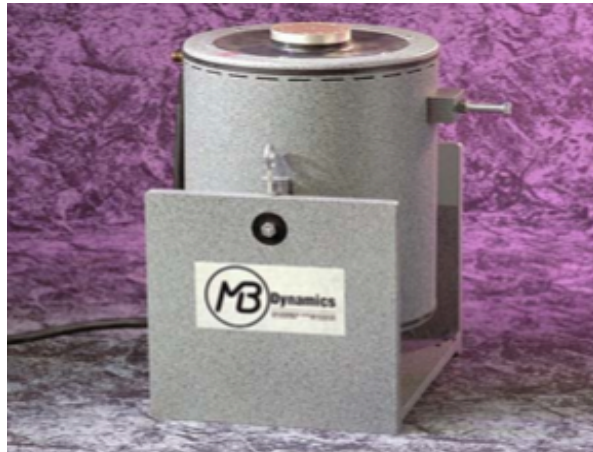
Figure 49 – Permanent Magnet Shaker
