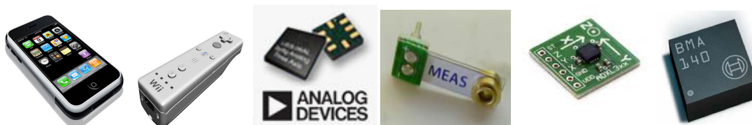
Figure 45 - Tested Accelerometer, listed from left to right, ADXL30 in the iPhone, LIS331DL in the Wiimote, ADXL278, Minisense 100, ADXL330, and BMA 140.
