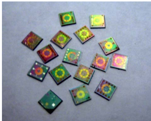
Figure 6.2: Different 4 x 4 mm 2 diced devices.
