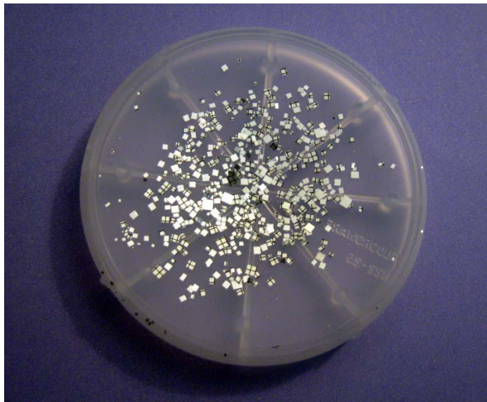
Figure 6.4: Different size aluminum coated micromirrors in a plastic dish.
