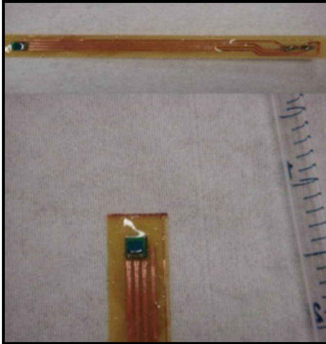
Figure 4.2: ISFET device glued on a dedicated PCB.
