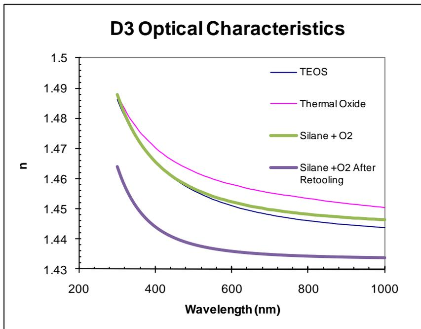
Figure 8.4: Index of refraction for dielectric formed by the silane and oxygen reaction.
