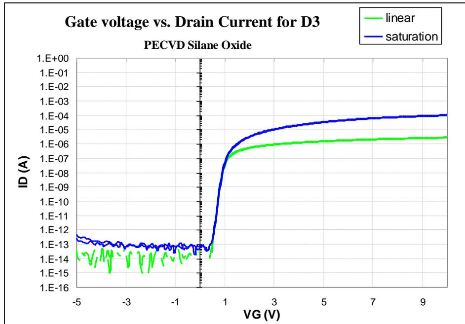
**Figure 7.17:** The current voltage relationship of D3 in both saturation ( $V_D = 5$  V) and linear ( $V_D = 0.1$  V).
