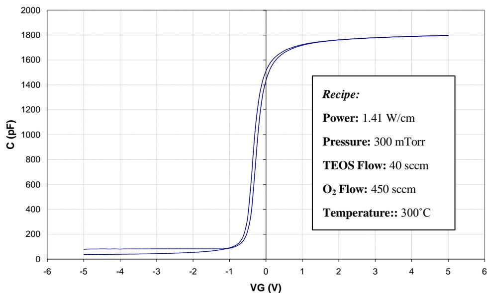
**Figure 6.14:** C-V plot of a sample that was deposited using a ratio of TEOS to O<sub>2</sub> of 1:11.25 and pressure of 1 Torr. The device used aluminum gate metal and a 0.002 cm<sup>2</sup> area capacitor.
