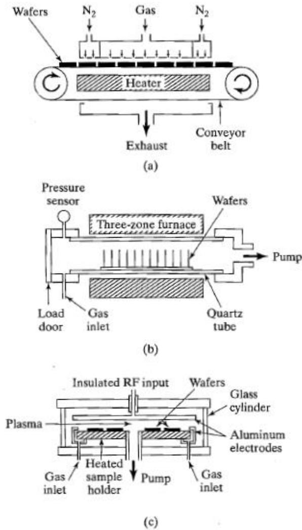
**Figure 2.1:** Three types of chemical vapor deposition (CVD) systems. (a) Atmospheric-pressure reactor; (b) hot-wall LPCVD system using a three-zone furnace tube; (c) parallel-plate plasma-enhanced CVD system [3].
