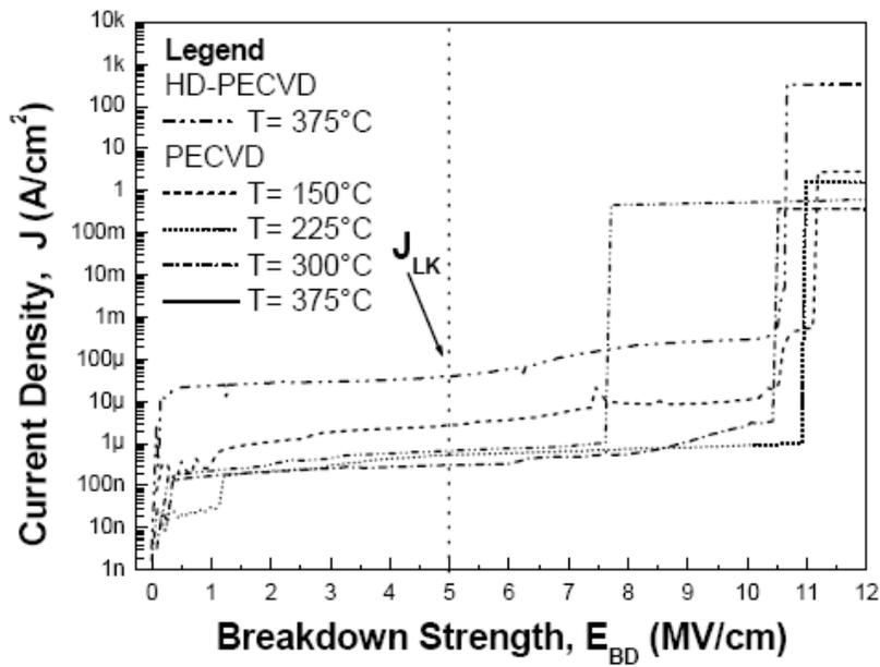
Figure 5.4: Electrical breakdown of different PECVD film [8].
