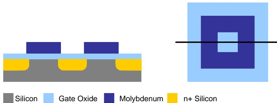
**Figure 7.6:** Cross-section of the NFET transistor after S/D implants.
