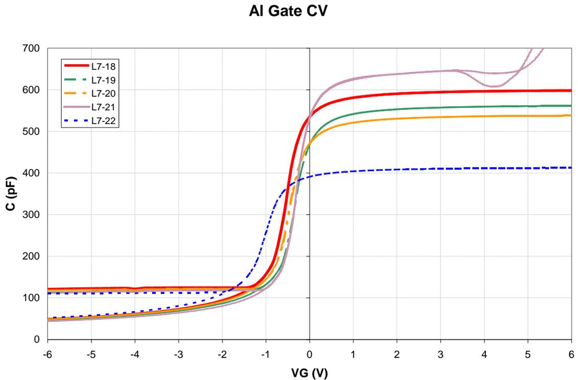
**Figure 6.21:** Overlay of C-V curves on samples with an Al gate and Al during sinter. The devices used an aluminum gate metal and a 0.002 cm<sup>2</sup> area capacitor.
