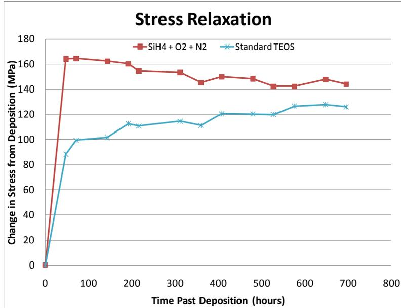
**Figure 8.8:** Stress relaxation (compressive shift) data for the dielectric that was formed by a silane, oxygen and nitrogen reaction, also used in wafer D2.
