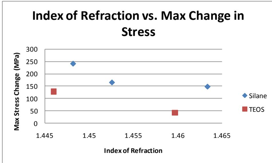
**Figure 8.11:** Index of refraction (@800 nm) vs. max change in stress for silane based oxides.
