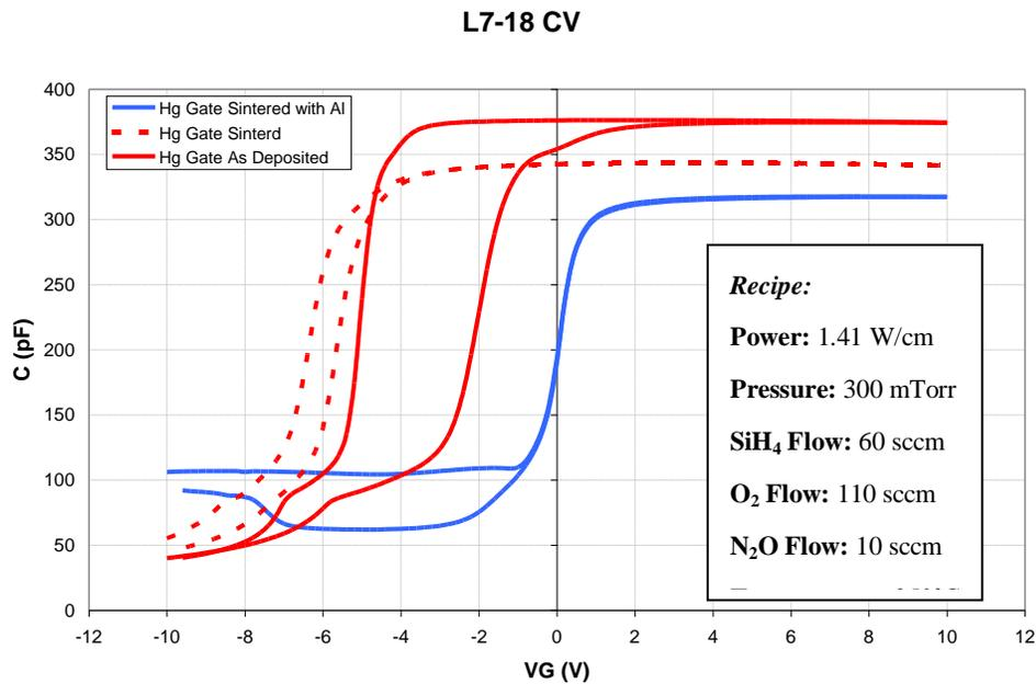
**Figure 6.16:** Overlay of L7-18 with different post gate oxide deposition annealing processes, showing elimination of hysteresis with the addition of an Al capping layer with use of a Hg gate during testing.
