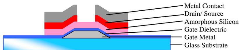
**Figure 1.1:** Bottom gate LCD TFT cross-section.
