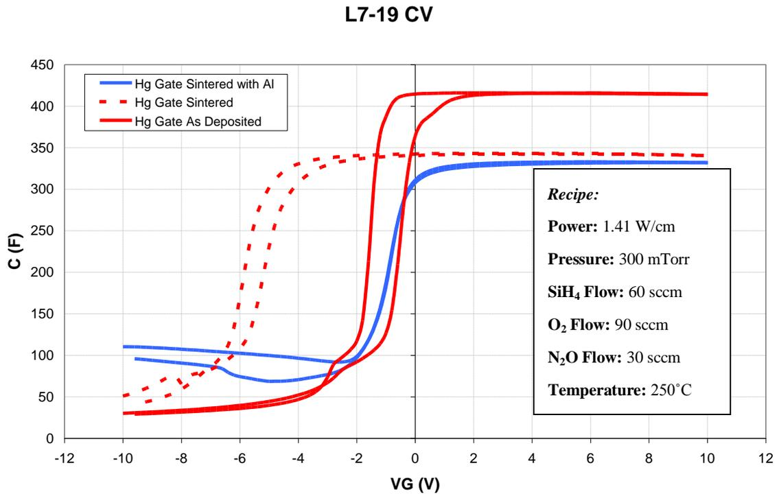
**Figure 6.17:** Overlay of L7-19 with different post gate oxide deposition annealing processes, showing elimination of hysteresis with the addition of an Al capping layer.
