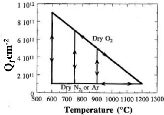
**Figure 3.2:** “Deal triangle” showing the reversibility of heat treatment effects on  $Q_f$  for a (111) oriented silicon wafer [10].
