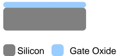
**Figure 6.3:** Cross-section of a MOS structure after gate oxide deposition.
