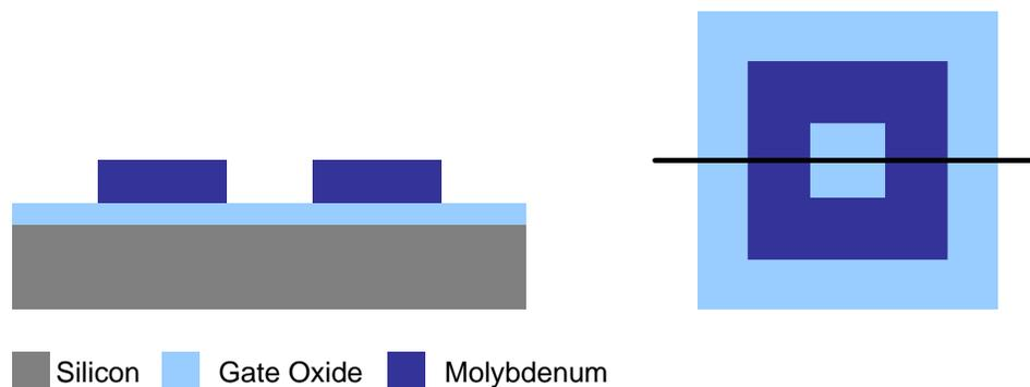
**Figure 7.5:** Cross-section of the NFET transistor after gate metal etch.
