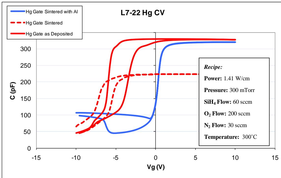
**Figure 6.20:** Overlay of L7-22 with different post gate oxide deposition annealing processes, showing elimination of hysteresis with the addition of an Al capping layer.
