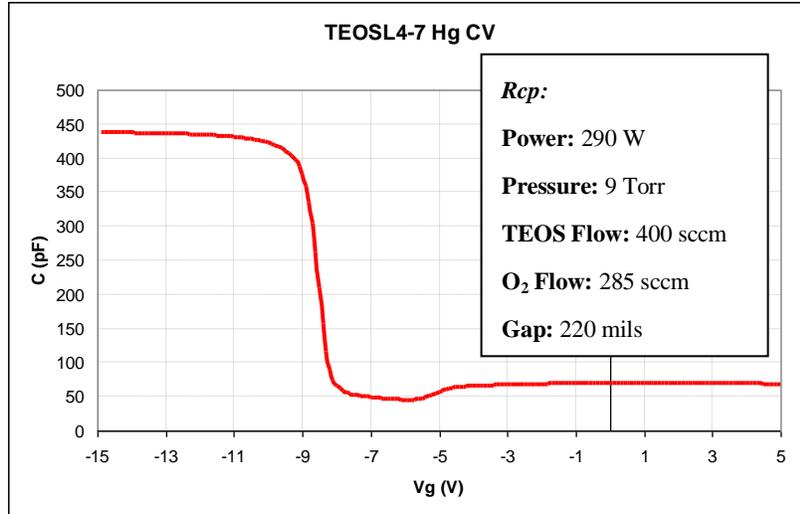
**Figure 6.12:** C-V measurement of the standard PECVD TEOS recipe used in the SMFL using an aluminum gate and a 0.002 cm<sup>2</sup> area capacitor.
