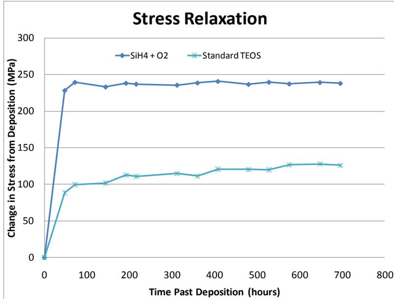
**Figure 8.9:** Stress relaxation (compressive shift) data from the dielectric that was formed by a reaction of silane and oxygen, used in device wafer D3.
