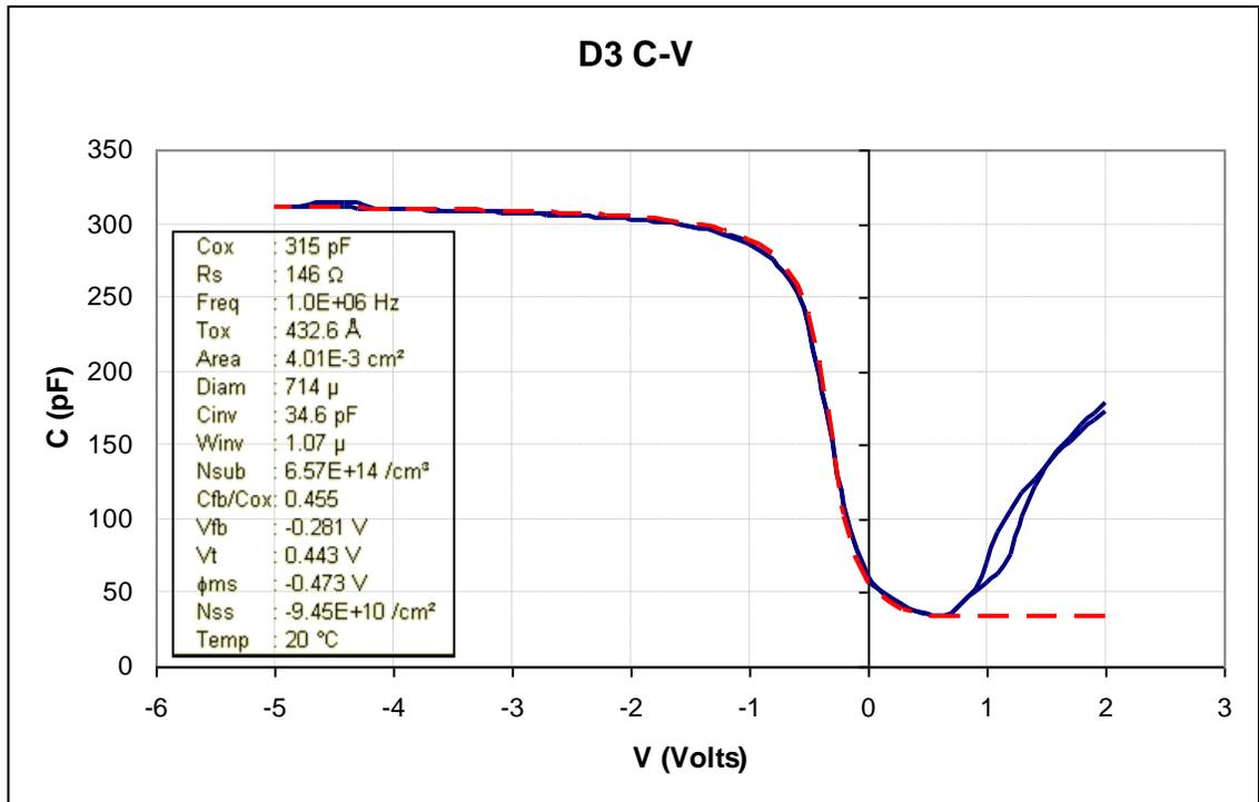
**Figure 6.26:** C-V curve for the device wafer D3, which had a SiH<sub>4</sub> based PECVD oxide for a gate dielectric in the NMOS process. The red dashed line shows the C-V curve that corresponds to the shown extracted parameters.
