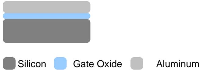
**Figure 6.7:** Aluminum deposited on gate oxide as gate metal.
