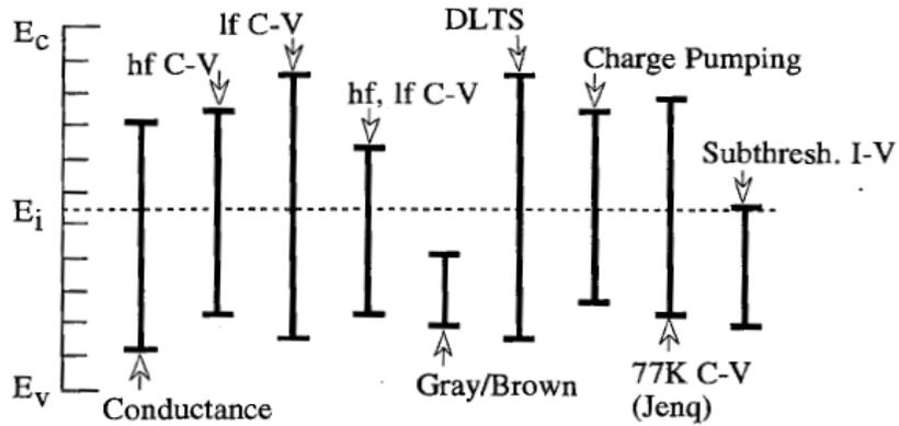
**Figure 3.4:** Ranges of energy in the band gap of a silicon p-type substrate over which interface trap charges are determined by various characterization techniques [12].
