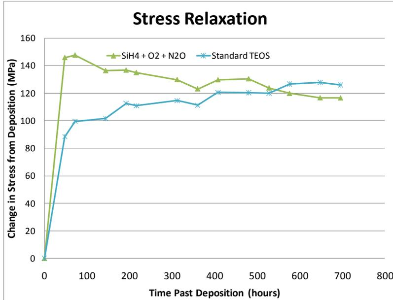
**Figure 8.10:** Stress relaxation (compressive shift) data from the dielectric that was formed by the reaction of silane, oxygen, and nitrous oxide, used in device wafer D4.
