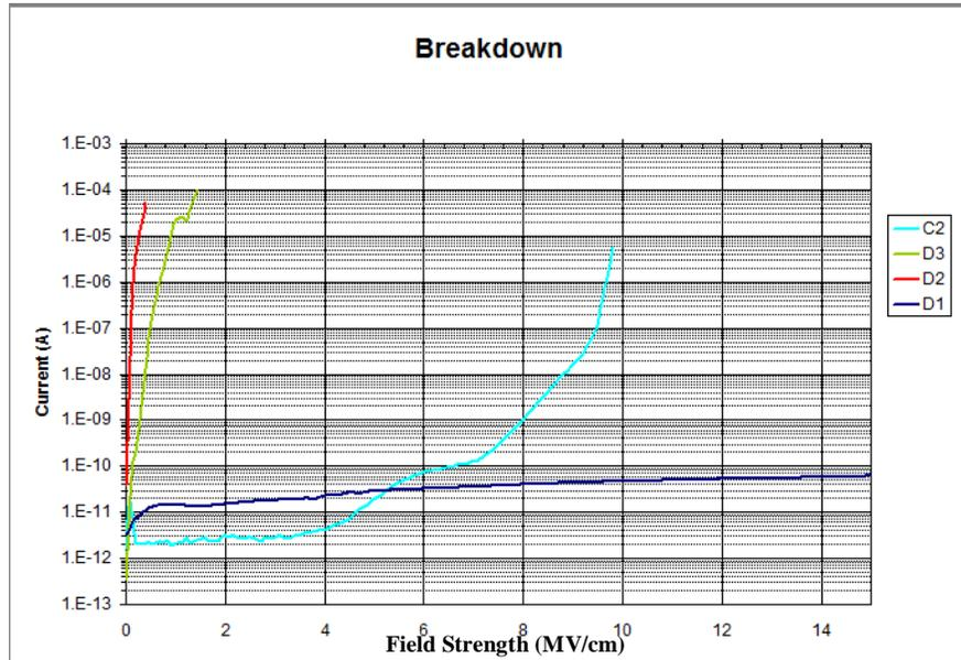
**Figure 6.27:** Breakdown of D1-D3 and C2, with D1 showing a less leakage and higher breakdown strength than the SiH<sub>4</sub> oxide.
