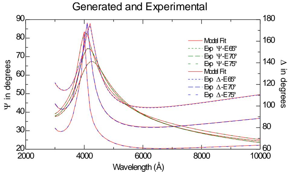
**Figure 8.1:** Representative fit of  $\Psi$  and  $\Delta$  using a Cauchy model.
