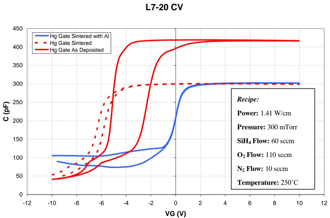
**Figure 6.18:** Overlay of L7-20 with different post gate oxide deposition annealing processes, showing elimination of hysteresis with the addition of an Al capping layer.
