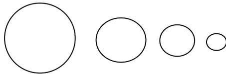
**Figure 6.10:** Diagram of fabricated circular capacitors ranging in diameter from 0.0357 to 0.1596 cm.
