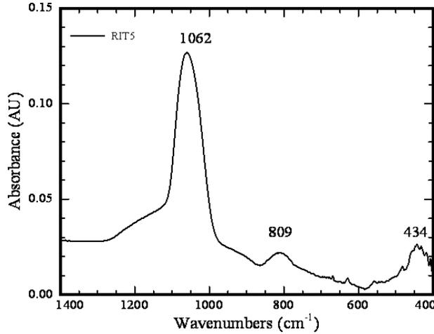
**Figure 4.3:** FTIR absorbance spectrum for a TEOS sample prepared at RIT.
