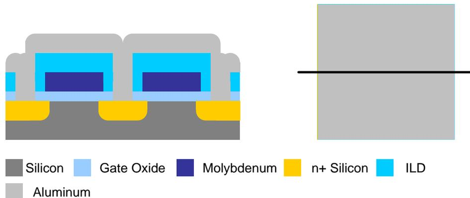
**Figure 7.10:** Cross-section of the NFET after aluminum deposition
