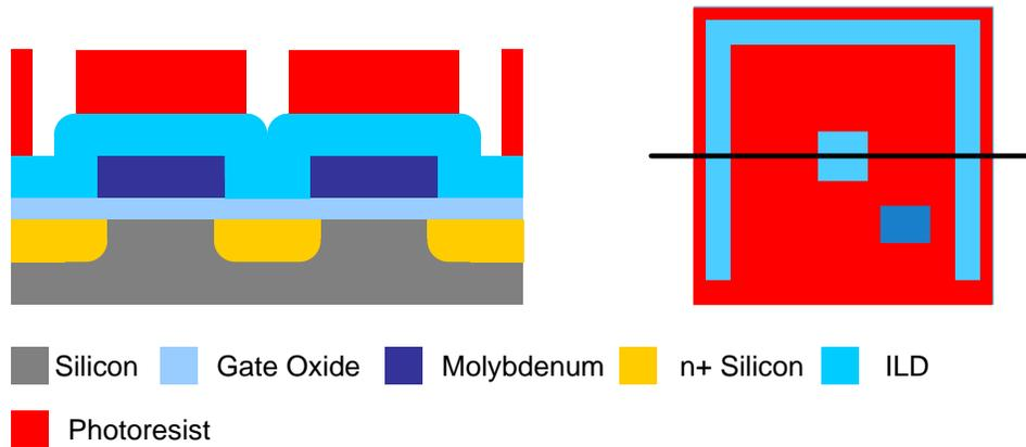
**Figure 7.8:** Cross-section of the NFET transistor after contact lithography.
