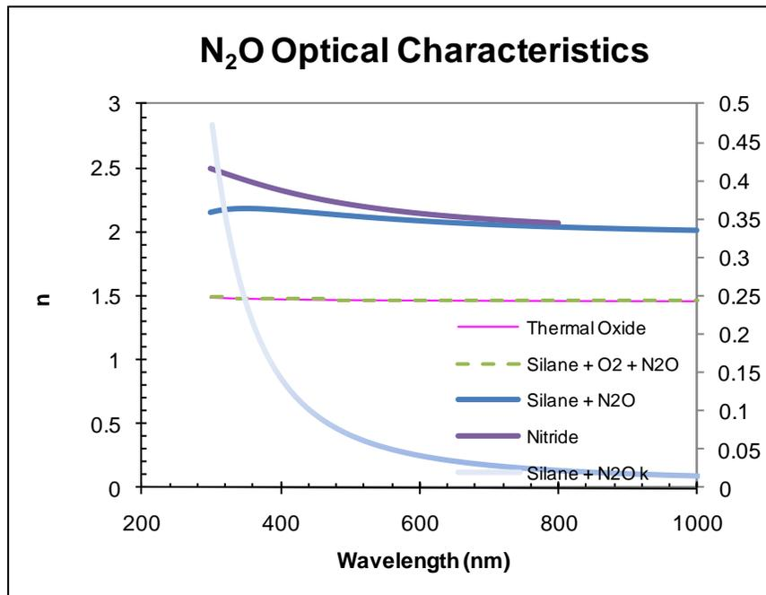
**Figure 8.6:** The index of refraction of various dielectric deposited with varying amounts of nitrous oxide and oxygen. Also plotted is thermal oxide and silicon nitride.
