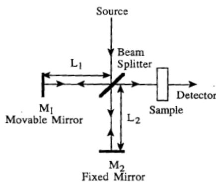
**Figure 4.2:** Schematic of a typical FTIR system [12].
