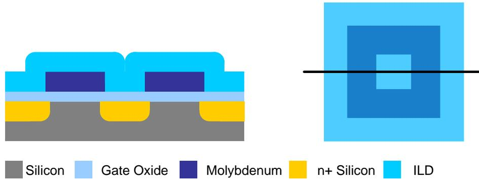
**Figure 7.7:** Cross-section of the NFET transistor after the ILD has been deposited.
