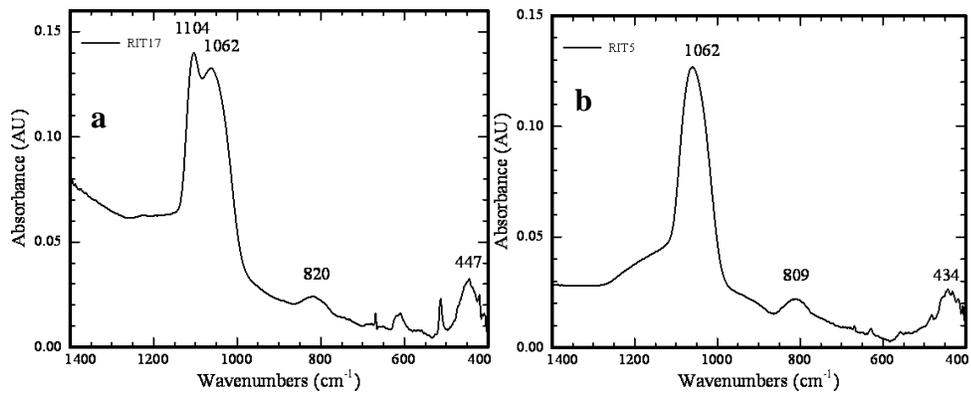
**Figure 6.13:** FTIR spectrum of PECVD TEOS taken on 100mm samples (a) and 150 mm samples (b).
