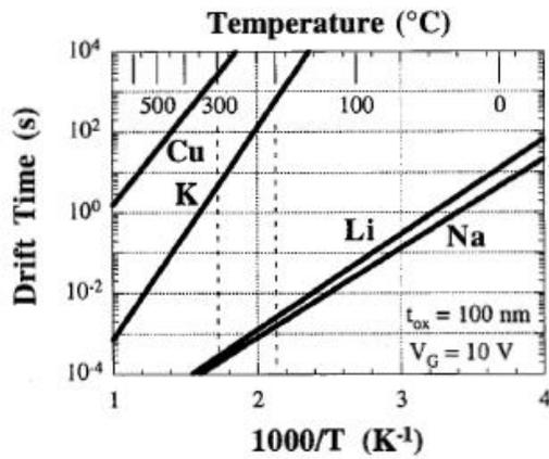
**Figure 3.3:** Drift time for Na, Li, K, and Cu for an oxide electric field of  $10^6 \text{ V/cm}$  and  $t_{\text{ox}}=100 \text{ nm}$  [12].
