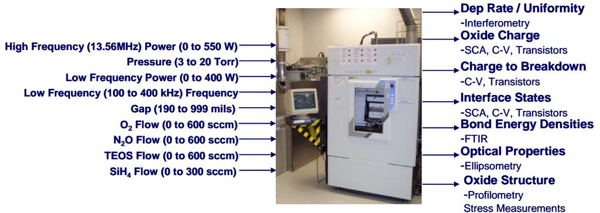
**Figure 6.1:** Picture of the Applied Materials P-5000 and input and output parameters.
