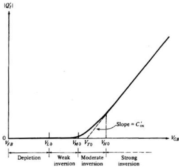
**Figure 5.2:** Magnitude of inversion charge per unit area vs. gate-substrate bias voltage [19].
