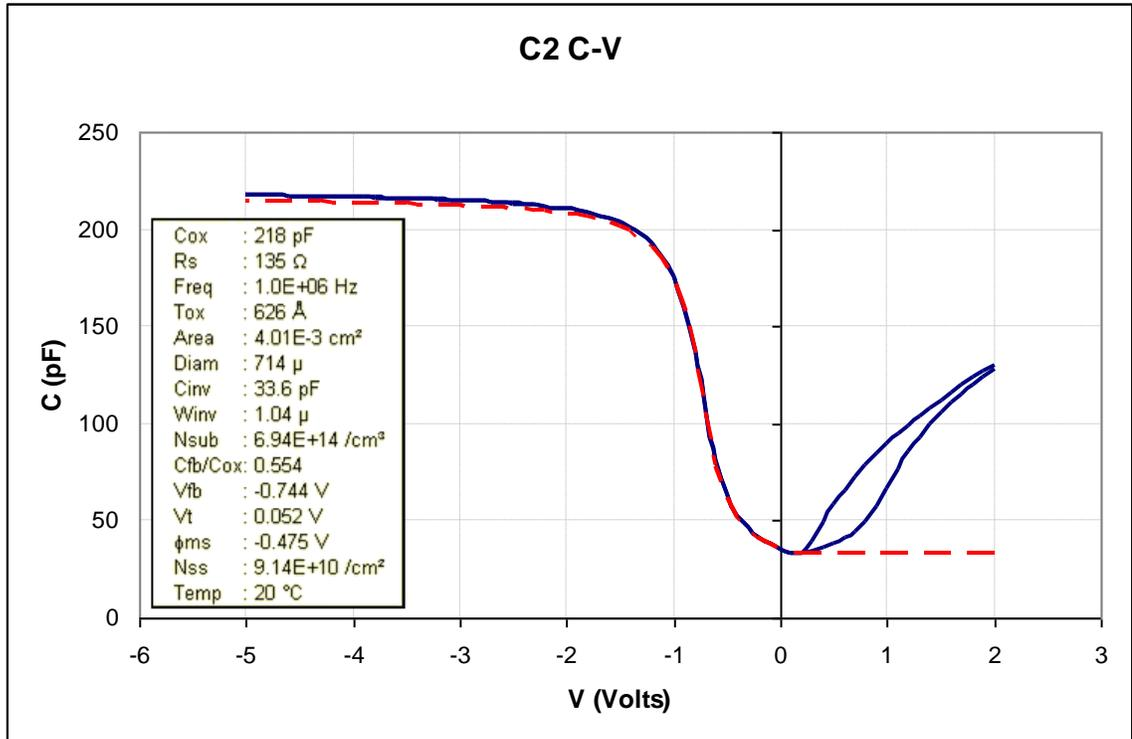
**Figure 6.23:** C-V curve for the control C2, which had an LTO LPCVD oxide for a gate dielectric and molybdenum for the gate metal in the NMOS process. The red dashed line shows the C-V curve that corresponds to the shown extracted parameters.
