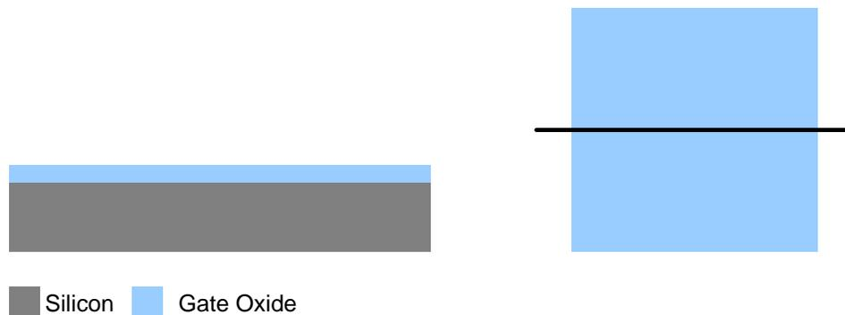
**Figure 7.2:** Cross-section and top down view after gate oxide deposition.
