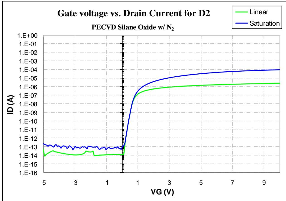
**Figure 7.16:** The current voltage relationship of a representative D2 transistor in both saturation ( $V_D = 5$  V) and linear ( $V_D = 0.1$  V).
