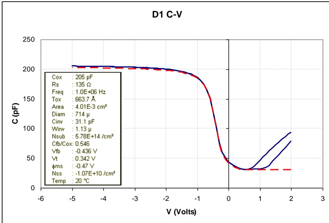
**Figure 6.24:** C-V curve for the device wafer D1, which had a TEOS based PECVD oxide for a gate dielectric in the NMOS process. The red dashed line shows the C-V curve that corresponds to the shown extracted parameters.
