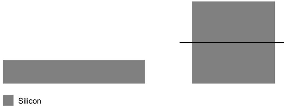
**Figure 7.1:** Starting (100) p-type silicon substrate.
