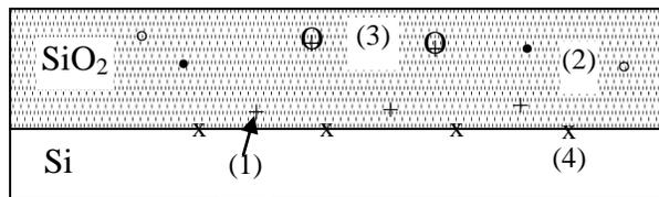
**Figure 3.1:** Charges and their location for thermally oxidized silicon. (1)-Fixed Oxide Charge, (2) - Oxide Trapped Charge, (3) - Mobile Oxide Charge, (4) – Interface Trapped [9].
