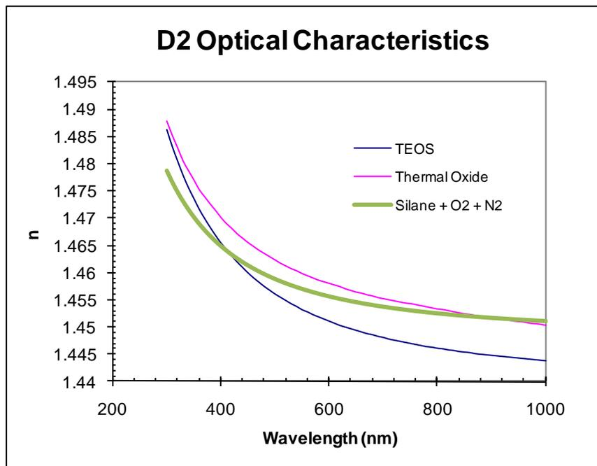
**Figure 8.3:** Index of refraction of the dielectric formed by the silane, oxygen, and nitrogen reaction.
