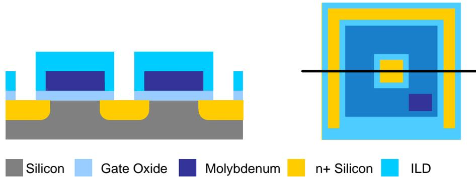
**Figure 7.9:** Cross-section of the NFET transistor after contact cut etch.
