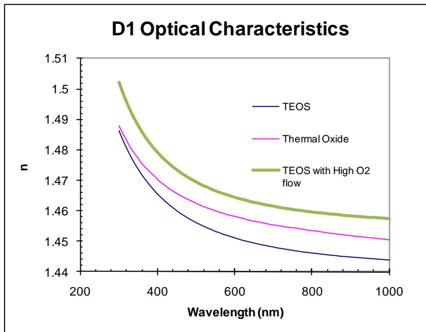
**Figure 8.2:** Index of refraction of the modified TEOS dielectric, D1, as well as a thermal oxide and the standard TEOS recipe.
