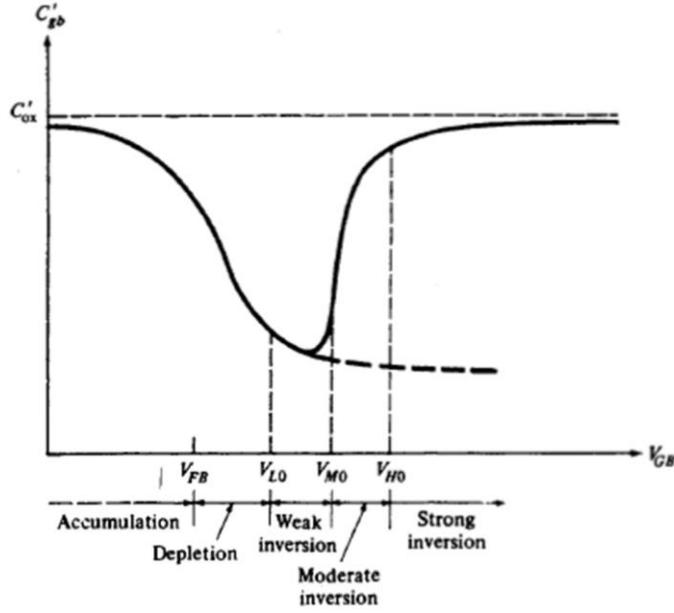
**Figure 5.3:** Diagram of a C-V curve showing the different regions of operation [19].
