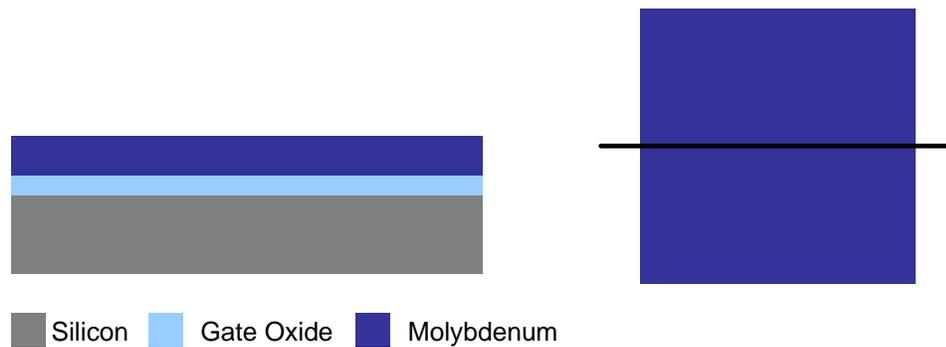
**Figure 7.3:** Cross section and top down view of the NFET after molybdenum gate metal deposition.
