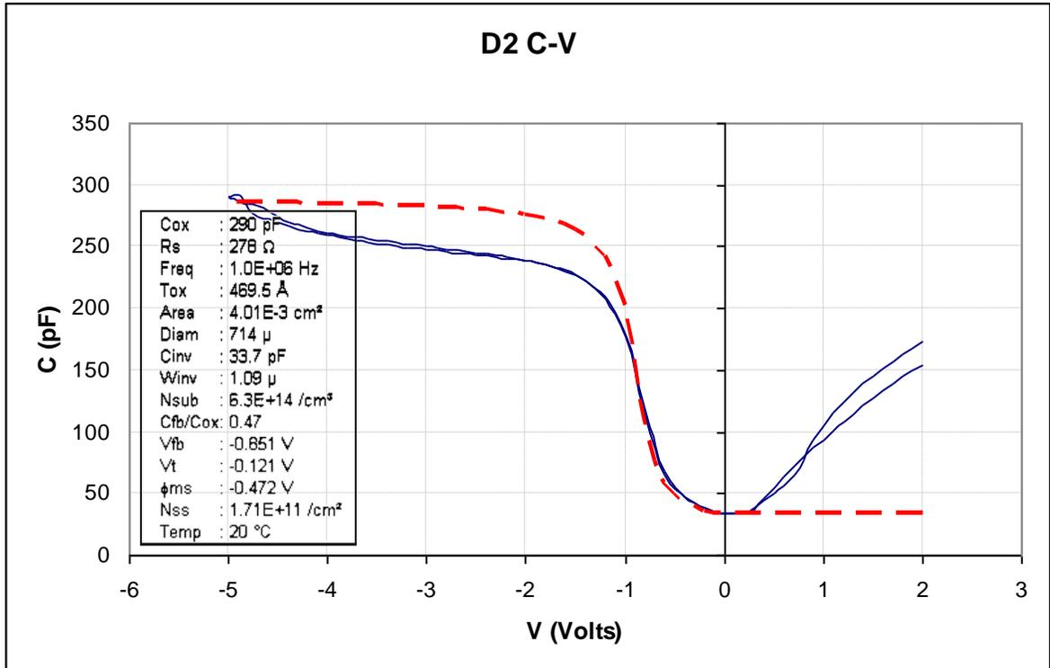
**Figure 6.25:** C-V curve for the device wafer D2, which had a SiH<sub>4</sub> based PECVD oxide with the addition of N<sub>2</sub> for a gate dielectric in the NMOS process. The red dashed line shows the C-V curve that corresponds to the shown extracted parameters.
