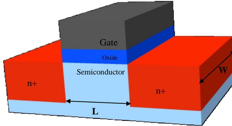
**Figure 5.5:** Cross-section of an n-MOSFET.
