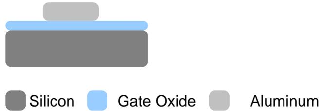
**Figure 6.9:** Aluminum after being etched.
