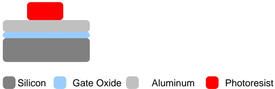
**Figure 6.8:** Photolithograph of aluminum.
