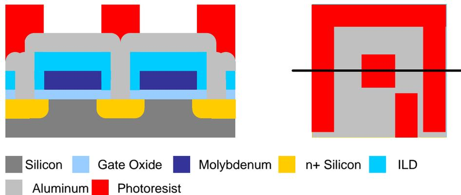
**Figure 7.11:** Cross-section of the NFET transistor after metal lithography.
