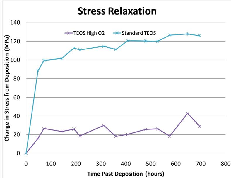
**Figure 8.7:** Stress relaxation (compressive shift) measurements for the dielectric that was formed by a modified TEOS sample, also used in device D1.
