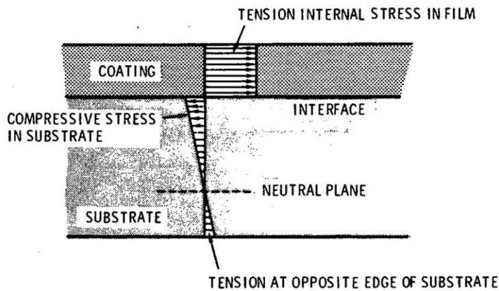
**Figure 4.6:** Schematic of the stress state of a thin film and substrate [17].
