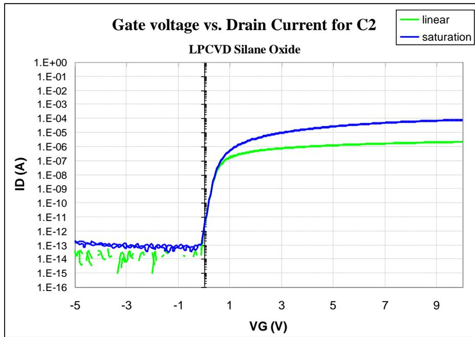
**Figure 7.14:** The current voltage relationship of representative C2 transistors in both saturation ( $V_D = 5$  V) and linear ( $V_D = 0.1$  V).
