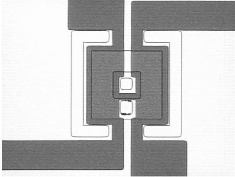
**Figure 7.13:** Optical picture at 50x showing a completed NMOS transistor with  $L=16\ \mu\text{m}$  and  $W\sim 160\ \mu\text{m}$ .
