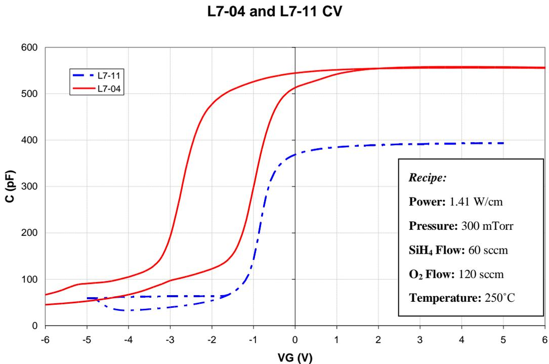
**Figure 6.15:** Overlay of L7-04 and L7-11 showing elimination of hysteresis with the use of an Al capping layer during sintering. The device used aluminum gate metal and a 0.002 cm<sup>2</sup> area capacitor.
