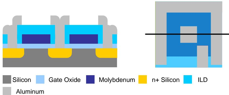
**Figure 7.12:** Cross-section of the NFET transistor after metal etch.
