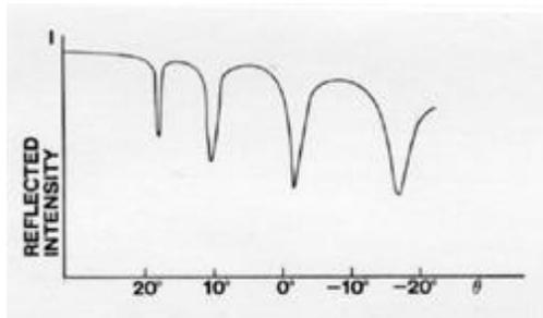
**Figure 4.5:** Intensity readout of a prism coupler showing the  $m=0, 1, 2, 3$  order minima's [16].
