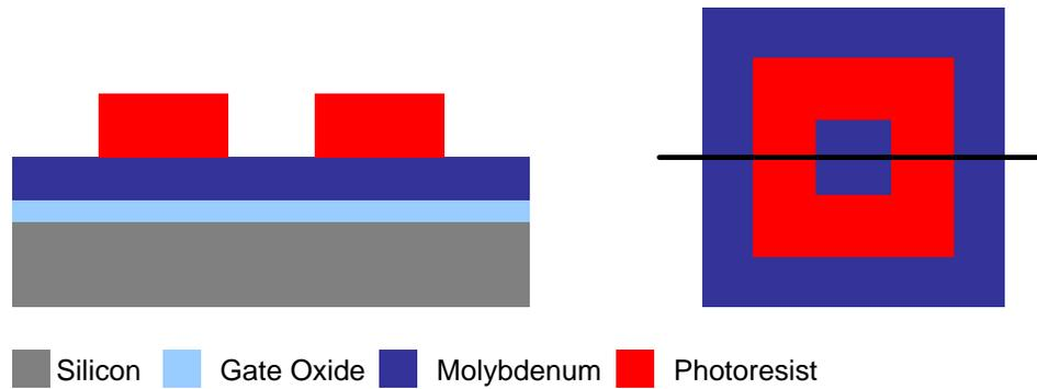
**Figure 7.4:** Cross-section of the patterned resist for the gate layer and top down view.
