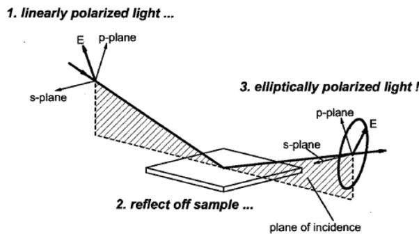
**Figure 4.1:** Geometry of an ellipsometry experiment, showing the p- and s-directions [13].
