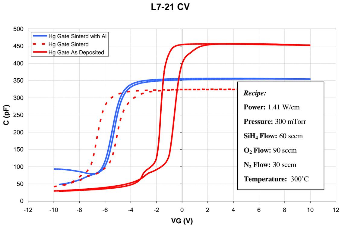
**Figure 6.19:** Overlay of L7-21 with different post gate oxide deposition annealing processes, showing reduction of hysteresis with the addition of an Al capping layer.
