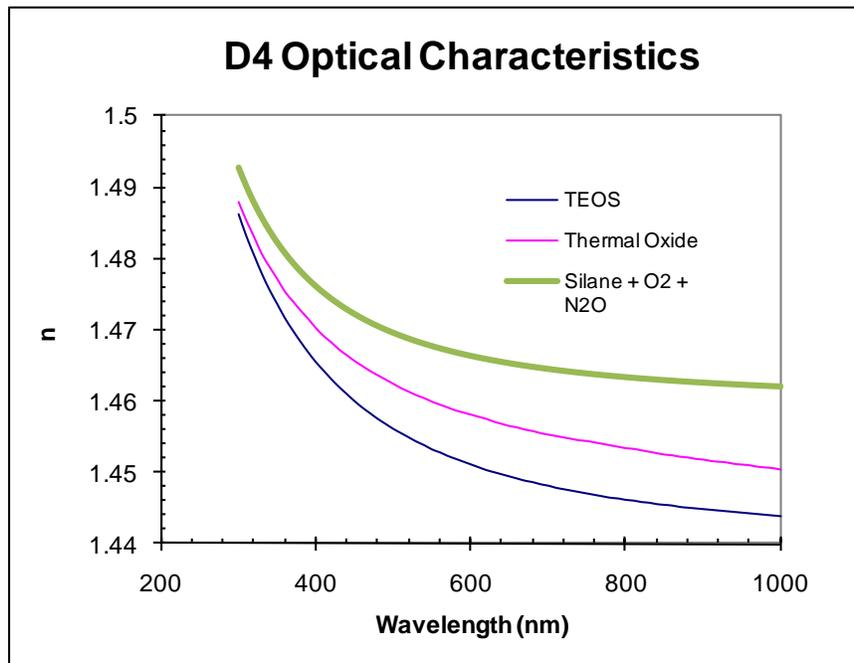
**Figure 8.5:** Index of refraction for the dielectric formed by the reaction of silane, oxygen and nitrous oxide.
