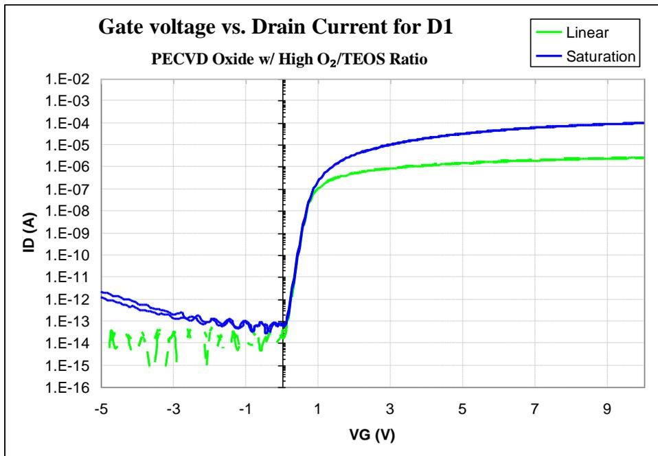
**Figure 9.2:** Gate voltage vs. drain current for a transistor fabricated with a molybdenum gate and PECVD TEOS gate oxide. Repeat of Figure 7.15.
