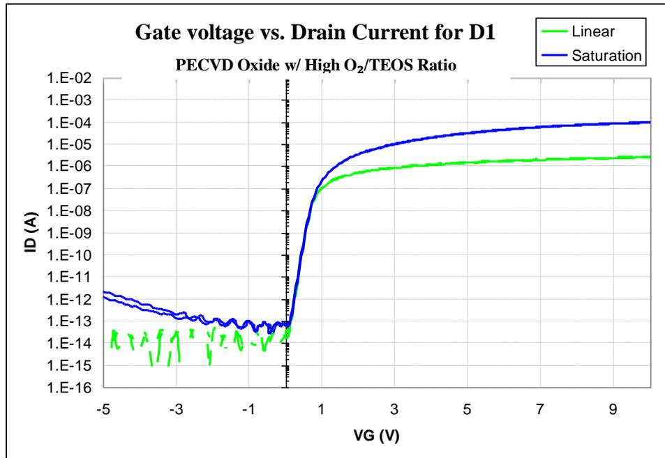
**Figure 7.15:** The current voltage relationship of representative D1 transistors in both saturation ( $V_D=5$  V) and linear ( $V_D=0.1$  V).
