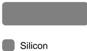
**Figure 6.2:** Starting substrate is (100) silicon.
