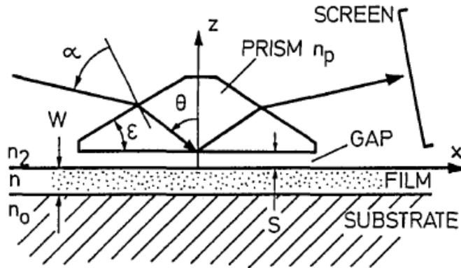
**Figure 4.4:** Schematic cross section of a prism coupler used in determining film thickness and refractive index [15].
