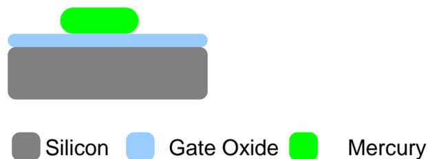
**Figure 6.4:** Cross section of the MOS device using mercury as the gate metal.
