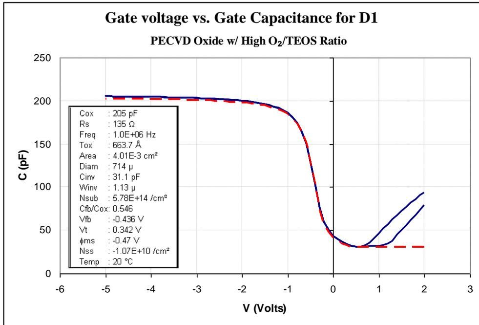
**Figure 9.1:** Gate voltage vs. gate capacitance for an integrated capacitor with a molybdenum gate and a PECVD TEOS oxide showing low charge levels. Repeat of Figure 6.24.
