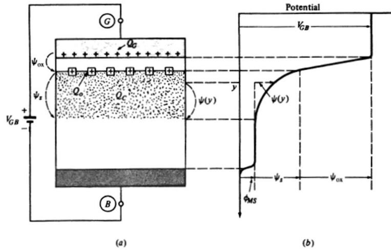
**Figure 5.1:** (a) A p-type substrate two-terminal MOS structure under general gate bias. (b) Potential distribution assuming the gate, substrate cap, and external wires are all made of the same material (assuming  $\psi_s > 0$ ) [19].
