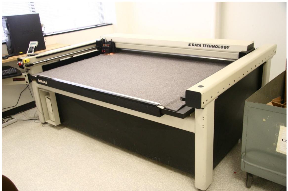
(Figure 10) Sample cutting table
