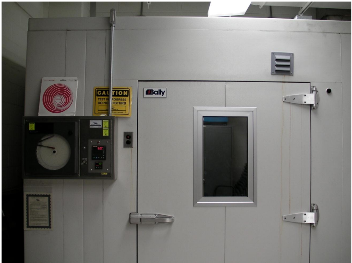
(Figure 12) Environmental chamber
