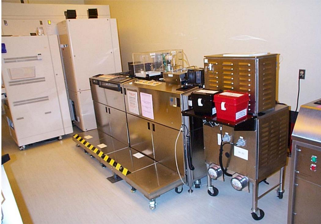
**Fig. 4.9: SSI coat and develop track at RIT SMFL**
