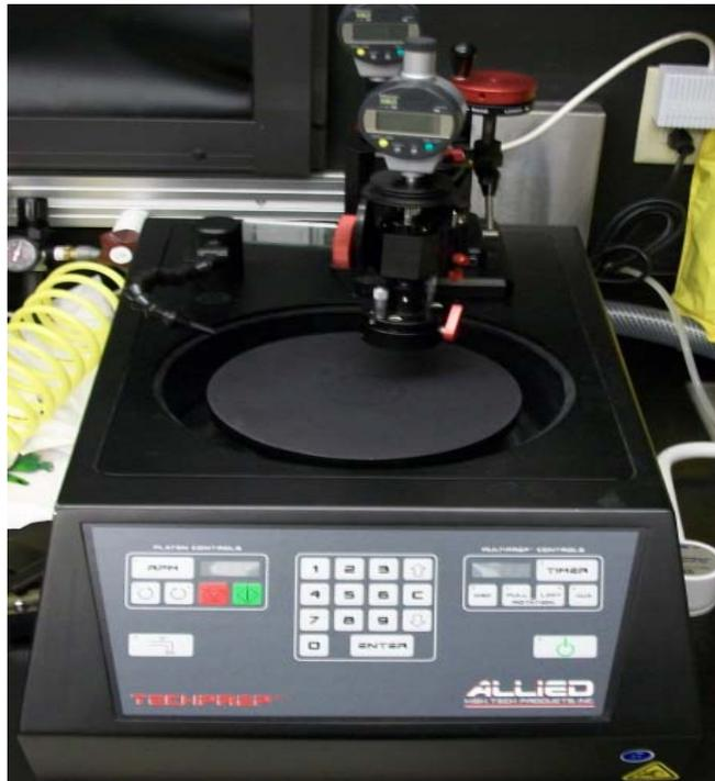
**Fig. 5.1: Allied Techprep grinding and polishing system**
