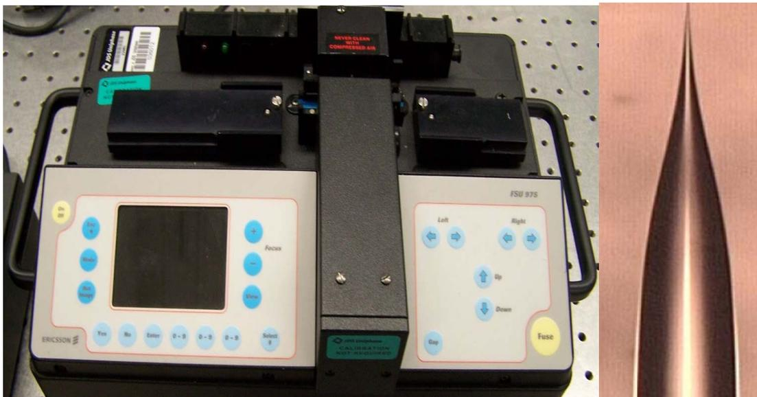
**Fig. 5.6: a) FSU975 fuser, b) Tapered optical fiber tip**
