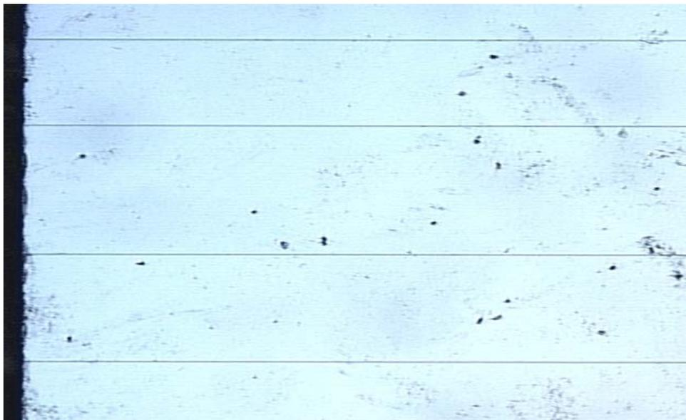
**Fig. 4.19b: Further microscopy showing resist smudges post dicing**
