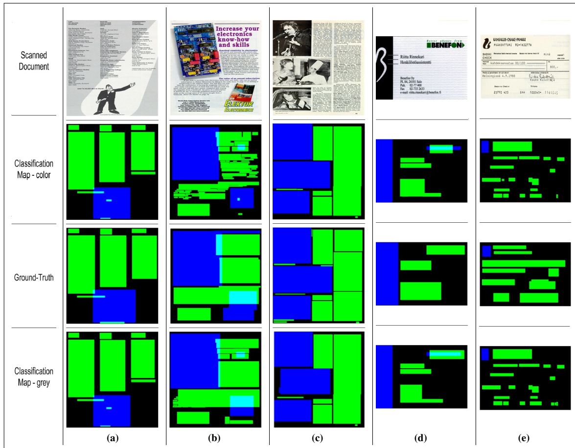
Fig. 4.3: Final classifications map for:(a) ADDRESS-LIST, (b) ADVERTISEMENT, (c) ARTICLE, (d) BUSINESS-CARD and (e) CHECK scanned document.
