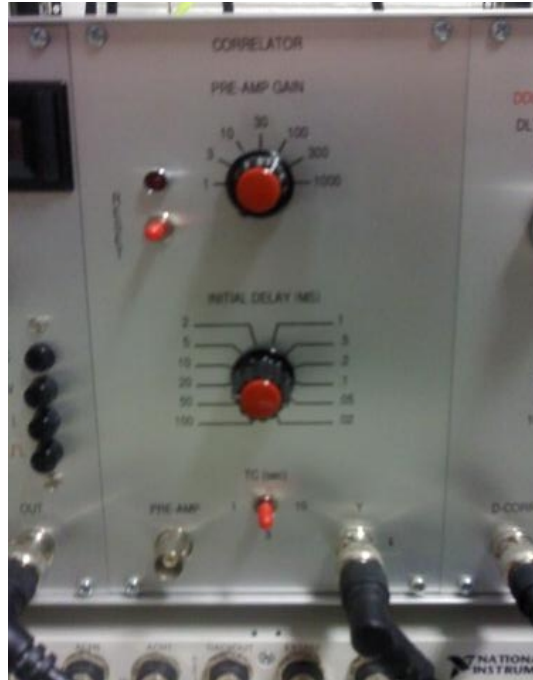
Figure 37: Correlator module on the DLTS system. The initial delay defines the size of t_{window} in milliseconds. The pre-amp gain knob is not relevant to the DLTS set-up here.
