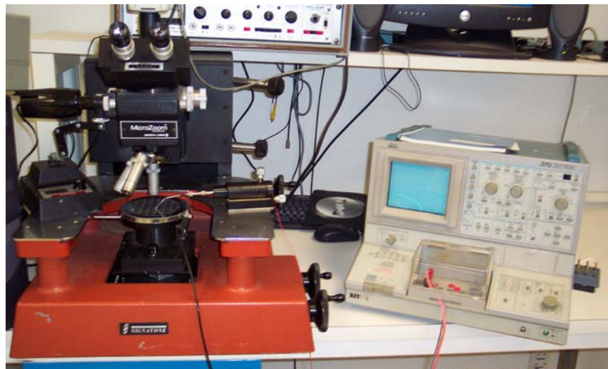
Figure 3.2: High-field charge injection setup located at RIT.
