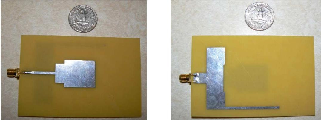
Figure 43: Manufactured UWB antenna on FR4.
