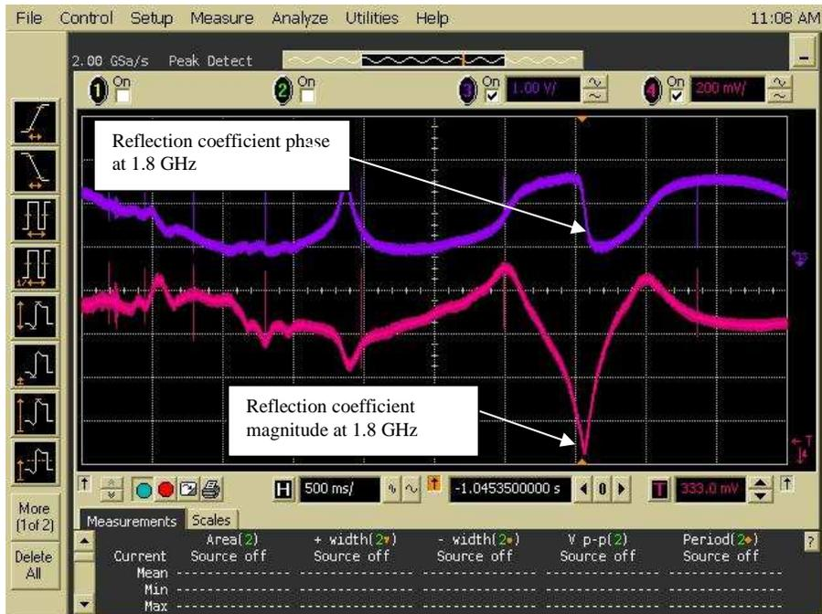
Figure 50: Output voltages of AD8302.
