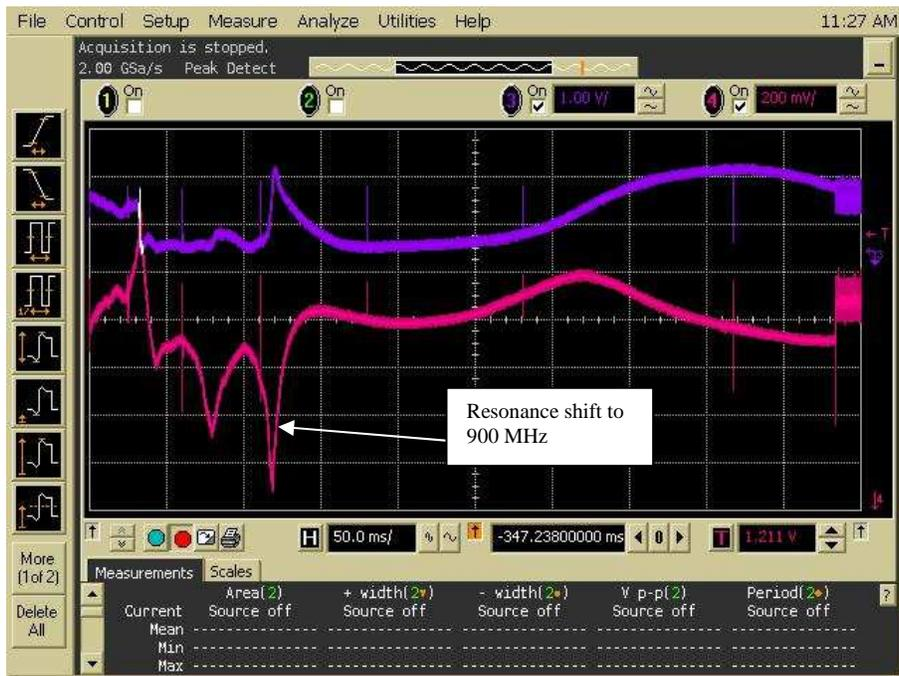
Figure 51: Output voltages of AD8302 with arm present.
