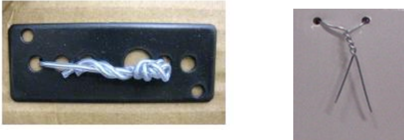
Figure 9. Previous wire-tie method with ends twisted several times.
