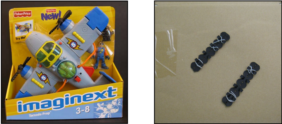
Figure 8. Wire-tie package sample: Front of package (left); back of package - exposing wire-tie fasteners (right).
