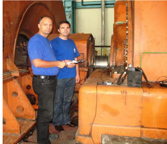
Fig. 11b: Collecting vibration data with VIBSCANNER
