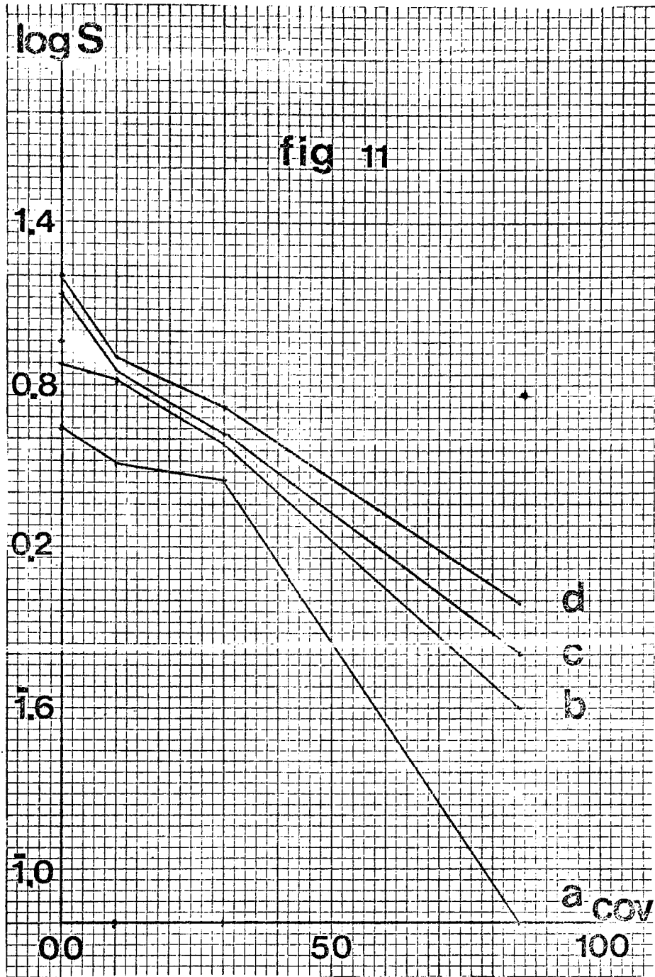
Figure 11. Log sensitivity vs. % of monolayer coverage (cov) for blue light exposures and the positive emulsion. Chemical development times: a. 1\frac{1}{2} min, b. 3 min, c. 4\frac{1}{2} min, d. 6 min, at 20^{\circ}\text{C} . Retardation of development is clearly indicated above 30% coverage.
