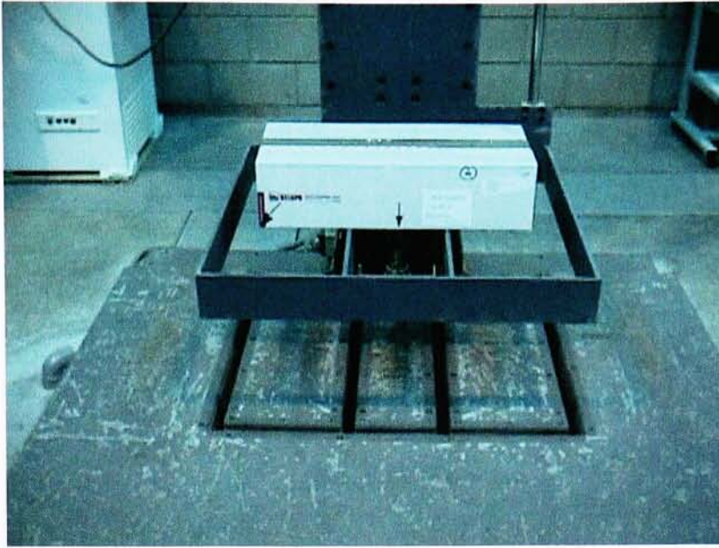
Fig. 6 Box Ref. Lupo in the drop tester
