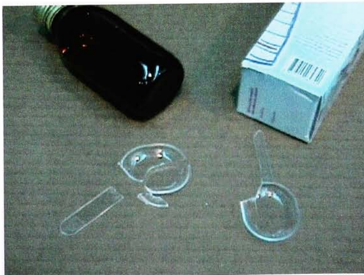
Fig. 11 Broken spoon after test
