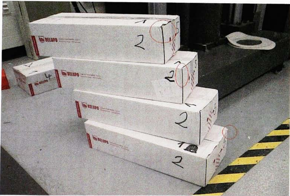
Fig. 14 Box corner damage after test.
