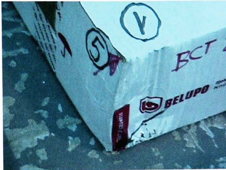
Fig. 10 Lateral edge of a box damage after test
