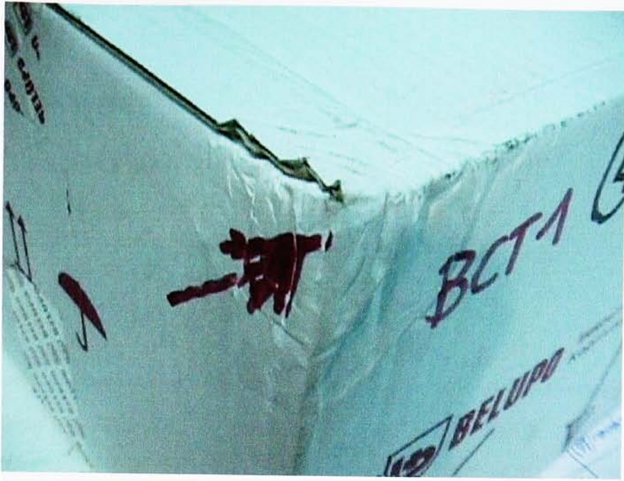
Fig. 20 Box corner damage after test
