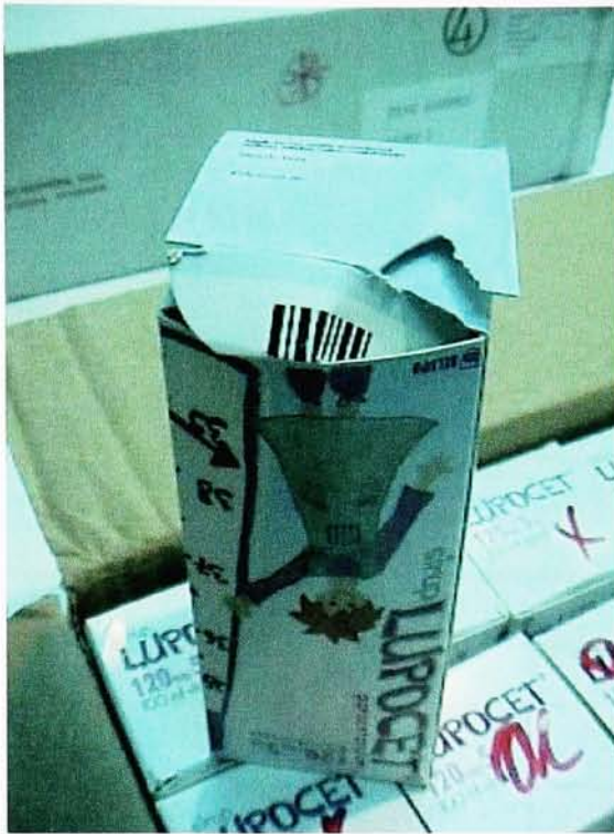
Fig. 12 Interior box damaged after test
