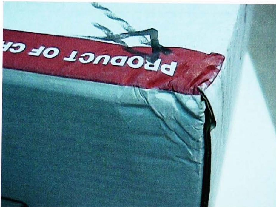
Fig. 18 Box corner damaged after test
