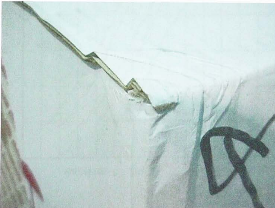
Fig. 23 Box corner damage
