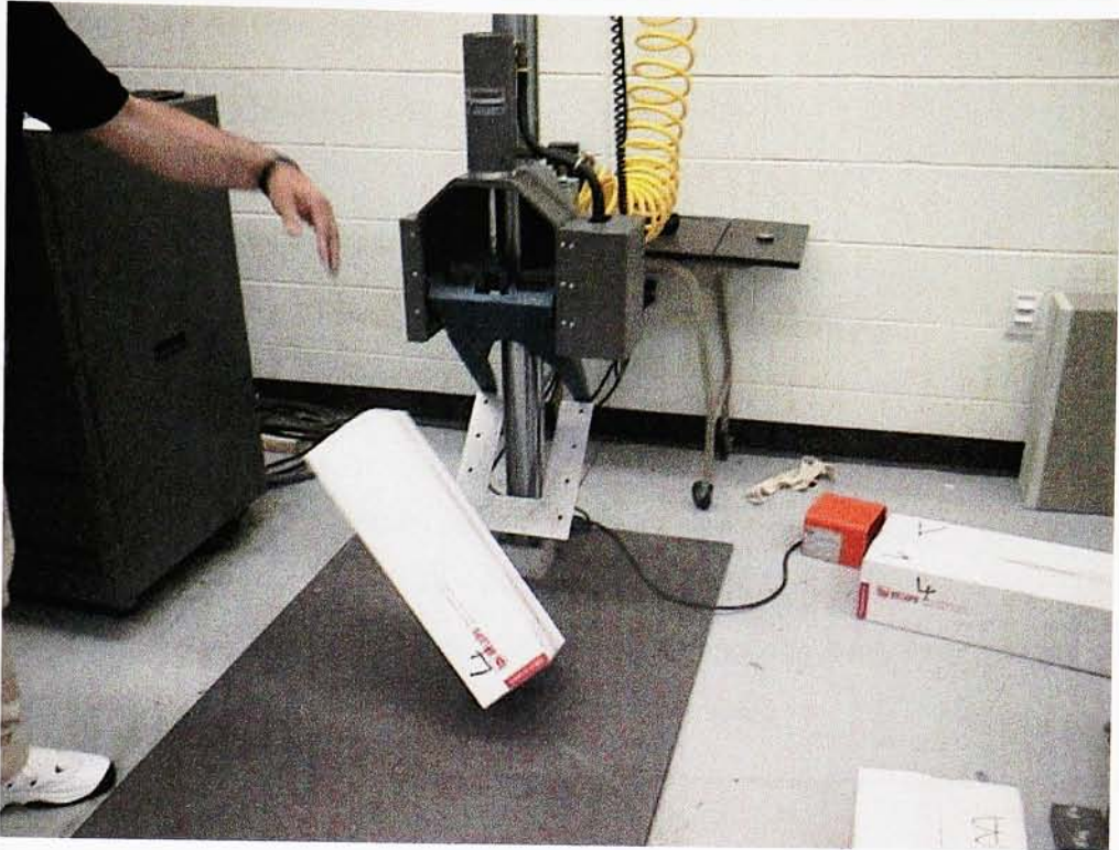
Fig. 13 Box Ref. Belos in the drop tester
