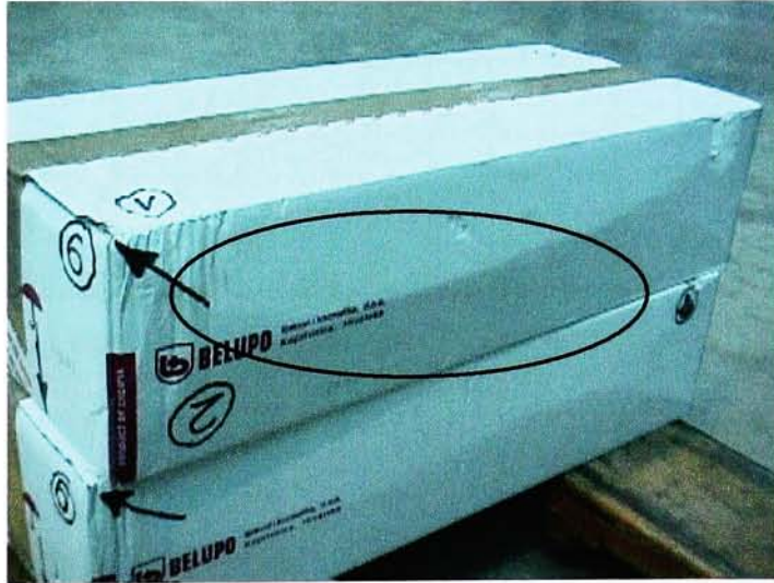
Fig. 8 Lateral face of a box damaged after test
