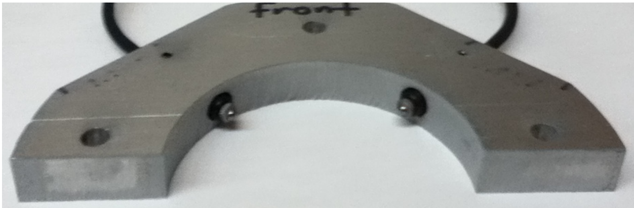
Figure 5.4: Machined sensor bracket with LVDTs installed
