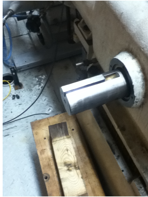
(b) LVDT bracket removed from compressor
