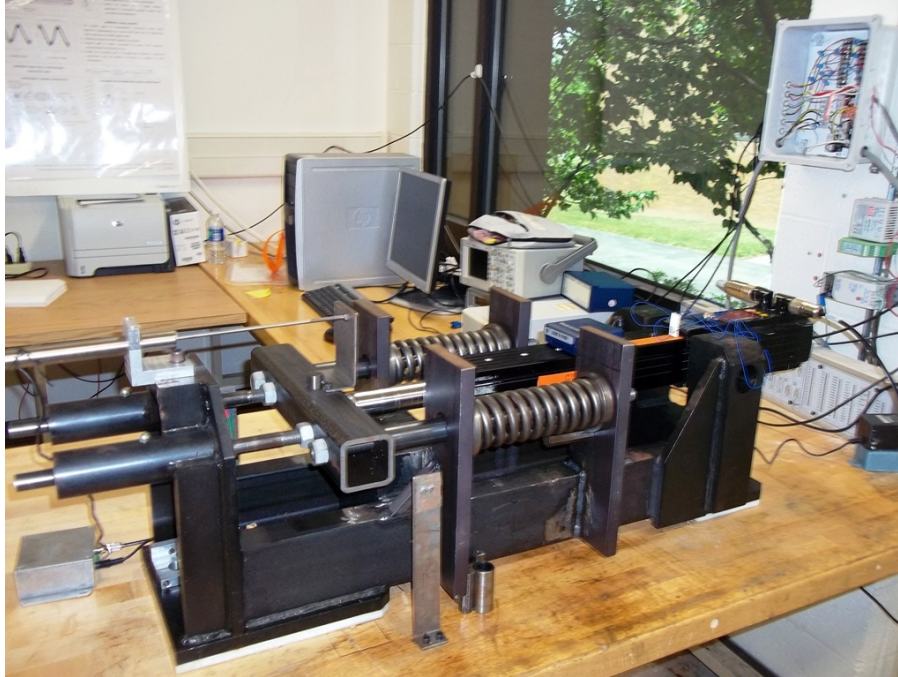
Figure 5.33: RIT Test Rig for Moog MaxForce EMA
