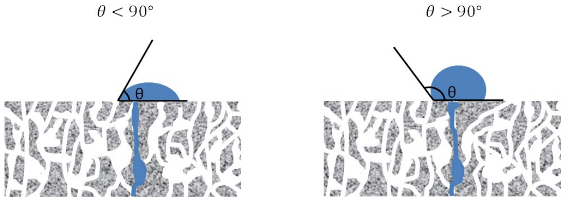
Figure 4: Water emergence from a GDL with a hydrophobic surface (right) and a hydrophilic surface (left) (Reproduced from [3]).
