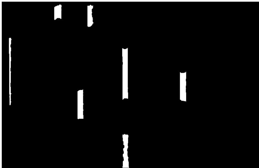
**Figure 4.15 - Closing of Figure 4.14 using disk structuring element.**
