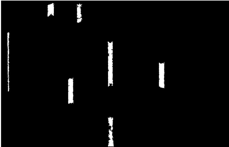
**Figure 4.13 - Area opening of thresholded image. Remaining connected components represent liquid water in the channels.**
