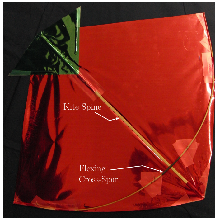
Fig. 1.11: Top of kite, showing flexing crossbar and spine structure.
