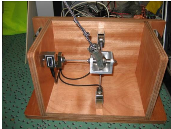
Fig. 4.1: Fixed tether length load cell used by Lansdorp et al. Image taken from [14].
