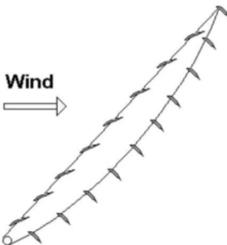
Fig. 1.6: The original laddermill power generation system design. Image taken from [17].
