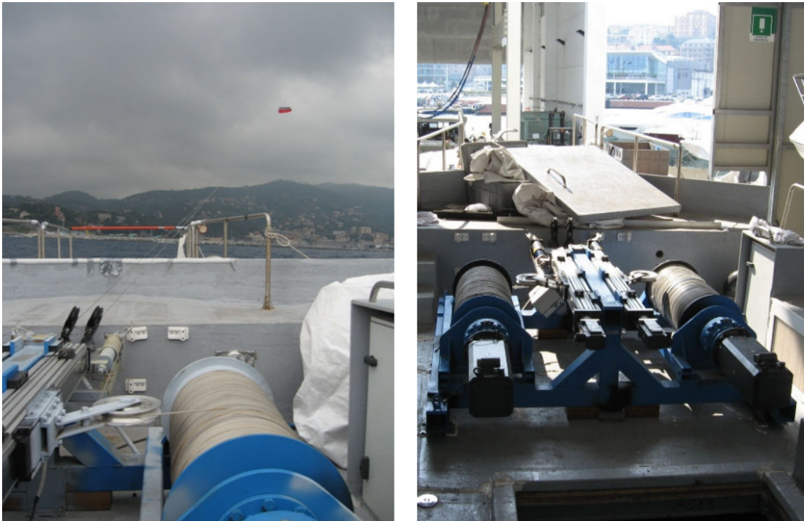
Fig. 1.4: Experimental flight tests of a manually operated kite system used for ship steering and propulsion. Kite is controlled by adjusting relative lengths of the two tethers. Image taken from [10].
