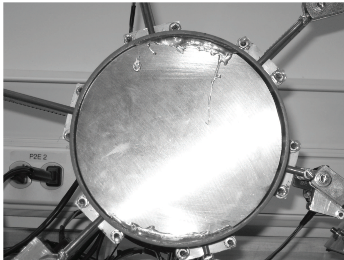
Figure 8.22: Counterweight mounted on core
