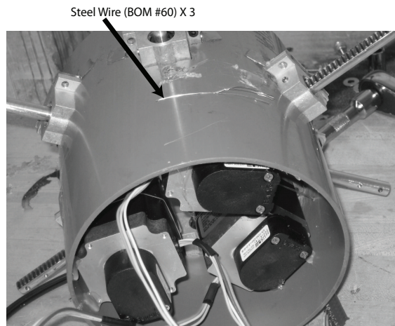
Figure 8.18: Securing and adjusting the motors
