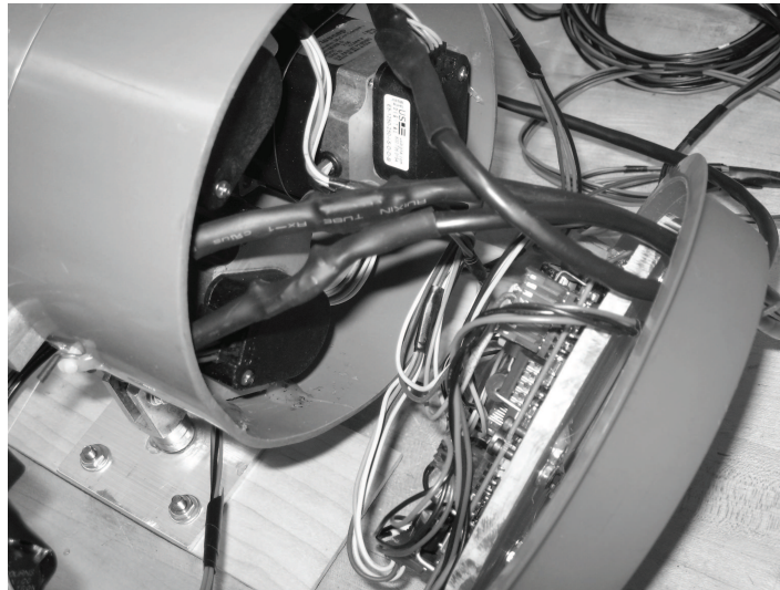
Figure 8.24: Electronics Assembly mounted on core
