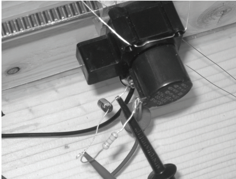
Figure 8.32: Analog Filter for potentiometer
