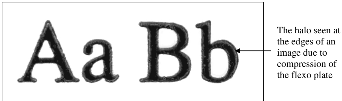
Figure 4: Illustration of the Halo Effect in Flexography (Brian Brollier, International Paper)
