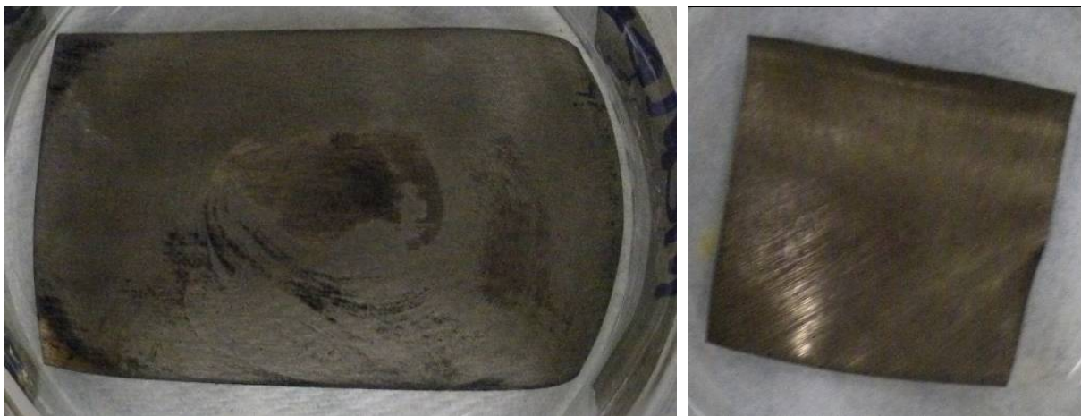
Figure 26. Photograph of the completed plated membranes. Shown on the left is the first sample, and on the right is the second sample.
