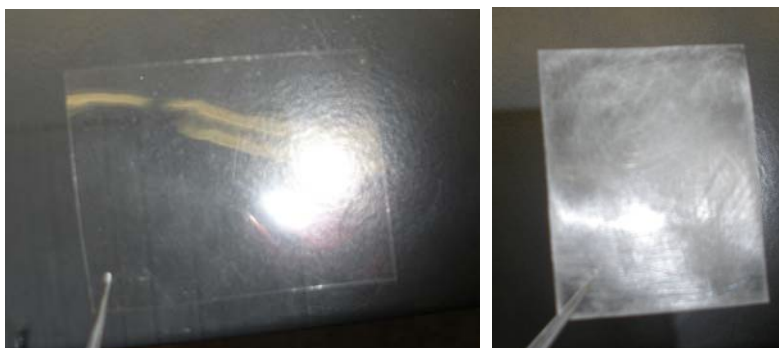
Figure 20. Photographs of the Nafion 117 membrane prior to surface roughening (left) and after surface roughening (right).
