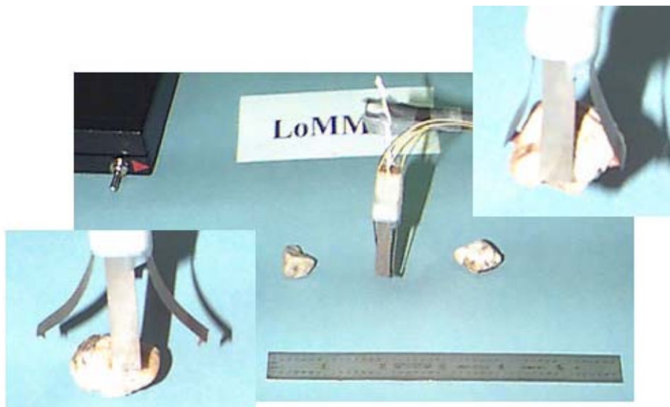
Figure 5. Microgripper made from an Ionic Polymer Metal composite actuators [29].
