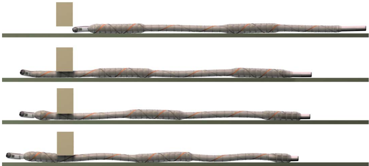
Figure 11. The Softworm using peristalsis to generate motion [24].
