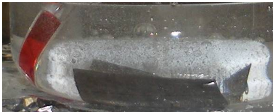
Figure 24. Close-up photograph of the hydrogen formation during reduction process.
