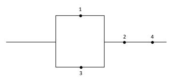
What may help at first is to identify which components must be working in order for the system to function. We see that either component 1 can work or component 3 can work, but that components 2 and 4 must work in order for the system to function. Notice that we have a combination here of parallel and series systems. We can write the structure function as follows:
