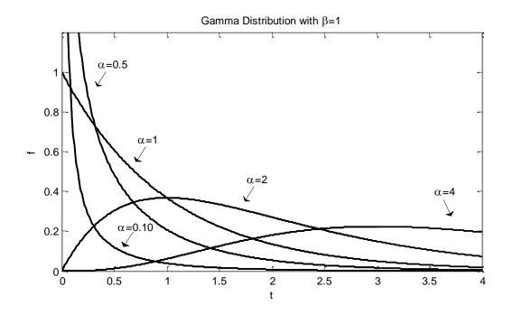
It can be easily proven that when  $\alpha < 1$ , the function has a DFR distribution, when  $\alpha > 1$ , the function has an IFR distribution, and when  $\alpha = 1$ , we are simply looking at the exponential distribution.
