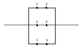
Notice that at least 2 out of the 3 components must be functioning in order to have a system that is functioning.
