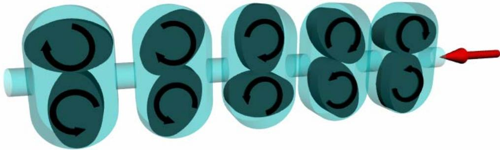
**Figure 1.2:** Oval gear positive displacement flowmeter.
