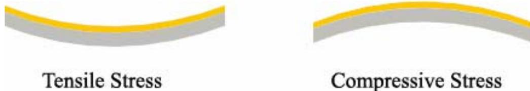
**Figure 5.2:** Tensile and compressive wafer bending after deposition of silicon nitride.
