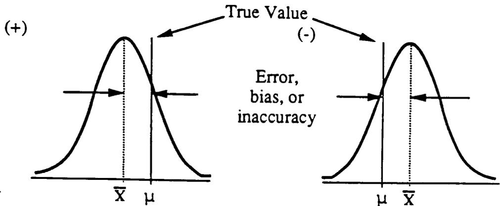
A measuring instrument is considered accurate if the error is less than the tolerance for that grade of instrument. In some test equipment the tolerance is about 2% of the measurement. The measurement equipment should have the ability to measure to 1/10 of the total product tolerance range.
