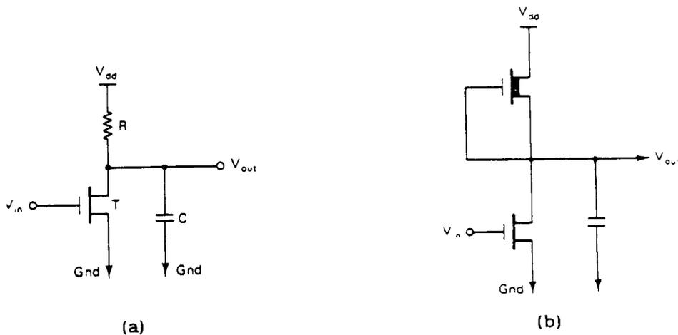
As can be seen above, the input voltage  $V_{in}$  is applied to the gate of  $T$ , which provides a very high input impedance via the gate capacitance  $C_g$ . This, in turn, will drive a similar output capacitance  $C$ . If  $V_{in}$  is less
