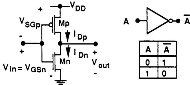
In order to derive the DC transfer characteristics for the inverter, one must first consider the regions of operation for the devices that make it up. These are shown below.
