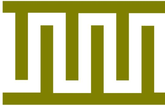
Fig. 1.5 A basic IDT structure.
