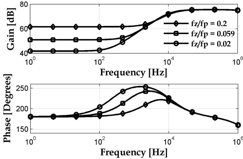
**Figure 4.10:** Bode Plot for Lead Compensator Circuit with  $R_O = 6\text{ k}\Omega$ ,  $C_1 = 30\text{ pF}$ ,  $C_C = 10\text{ pF}$ ,  $g_m = -1\text{ S}$ ,  $R_B = 500\text{ k}\Omega$ , and  $R_T$  swept with values of  $2\text{ M}\Omega$ ,  $8\text{ M}\Omega$ , and  $24\text{ M}\Omega$ .
