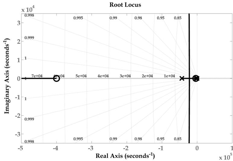
Figure 5.15: DCM Boost Converter with PI Control Root Locus
