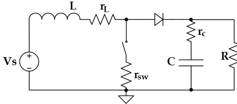
**Figure 2.3:** Non-Ideal Boost Converter Circuit
