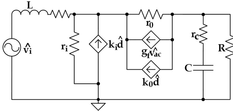
**Figure 3.18:** Equivalent Small-Signal Non-Ideal Boost Circuit in DCM
