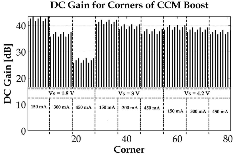
**Figure 5.10:** CCM Boost Converter DC Gain Over Parameter Corners.  $V_S = [1.8\text{ V}, 3\text{ V}, 4.2\text{ V}]$ ,  $I_O = [150\text{ mA}, 300\text{ mA}, 450\text{ mA}]$ ,  $L = [170\text{ }\mu\text{H}, 200\text{ }\mu\text{H}, 230\text{ }\mu\text{H}]$ ,  $g_m = [0.93\text{ }\mu\text{S}, 1.03\text{ }\mu\text{S}, 1.13\text{ }\mu\text{S}]$ .
