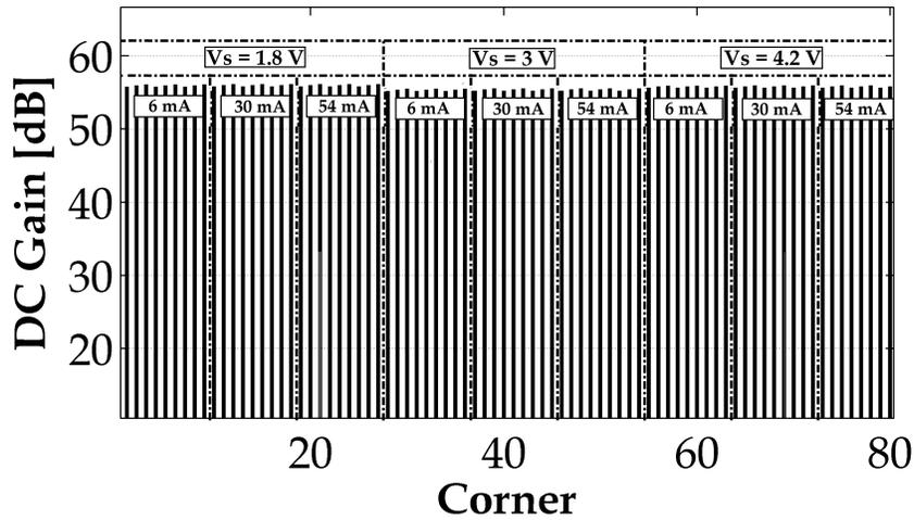
**Figure 5.20:** DCM Boost Converter DC Gain Over Parameter Corners.  $V_S = [1.8V, 3V, 4.2V]$ ,  $I_O = [6mA, 30mA, 54mA]$ ,  $L = [15\mu H, 20\mu H, 25\mu H]$ ,  $g_m = [8mS, 10mS, 12mS]$ .
