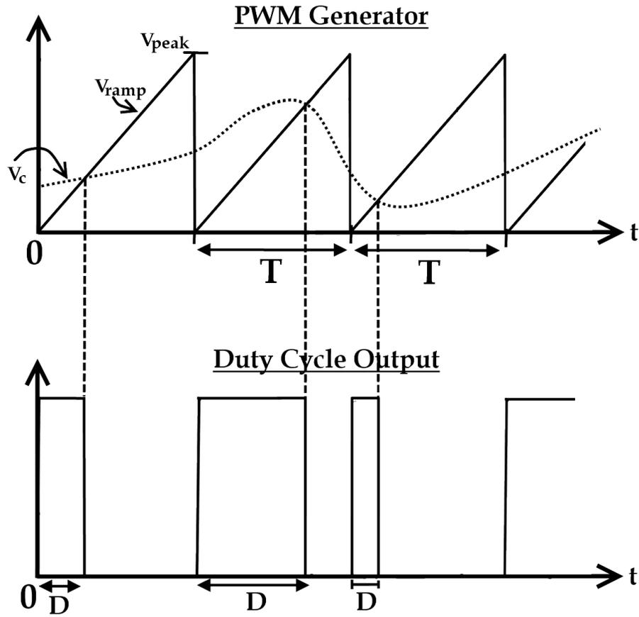
Figure 3.3: PWM Generation Circuit Waveforms
