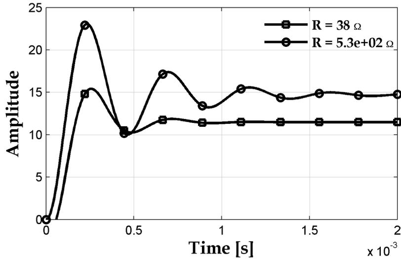
**Figure 3.16:** Step Response for Non-Ideal Boost in CCM with  $L = 180 \mu H$ ,  $C = 4.7 \mu F$ ,  $F_S = 350 kHz$ ,  $\frac{V_O}{V_S} = 2.5$ ,  $r_L = 0.8 \Omega$ , and  $r_C = 0.1 \Omega$ .
