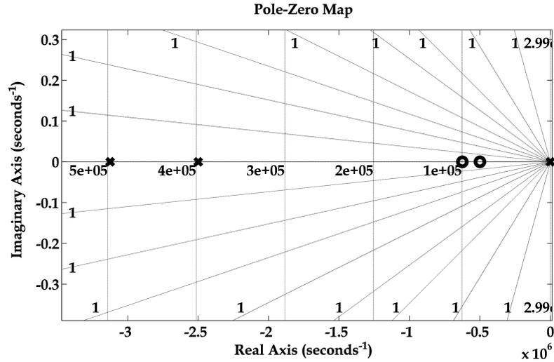
**Figure 4.13:** Pole-Zero Plot for Lag-Lead Compensator Circuit with  $C_1 = 0.8\text{ pF}$ ,  $C_C = 2\text{ nF}$ ,  $g_m = -10\text{ }\mu\text{S}$ ,  $R_B = 500\text{ k}\Omega$ ,  $R_T = 2\text{ M}\Omega$ ,  $C_Z = 300\text{ nF}$ , and  $R_Z$  swept with values of  $100\text{ }\Omega$ ,  $500\text{ }\Omega$ , and  $1\text{ k}\Omega$ .
