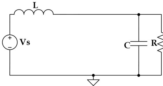
**Figure 3.5:** Ideal Boost Converter with Switch Open
