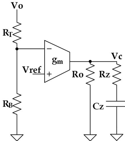
**Figure 4.3:** Lag Compensator Circuit
