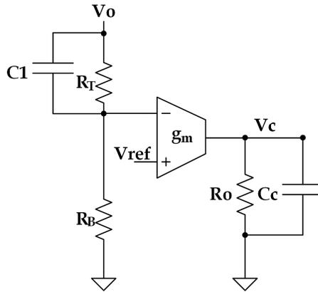
**Figure 4.9:** Lead Compensator Circuit
