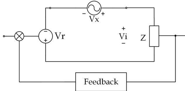
**Figure 6.4:** Voltage Injection via Middlebrook's Method.
