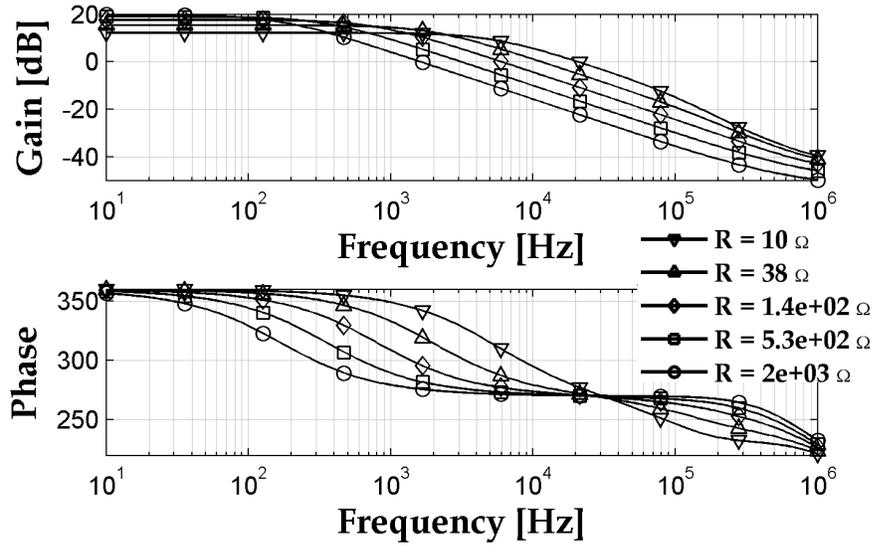
**Figure 3.20:** Bode Plot for Non-Ideal Boost in DCM with  $L = 18 \mu H$ ,  $C = 4.7 \mu F$ ,  $F_S = 350 kHz$ ,  $\frac{V_O}{V_S} = 1.6$ ,  $r_L = 0.8 \Omega$ , and  $r_C = 0.1 \Omega$ .
