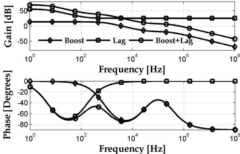
**Figure 4.14:** Bode Plot for Lag Compensator with DCM Boost with  $G_{d0} = 5$ ,  $C_O = 10\ \mu\text{F}$ ,  $R_{ESR} = 0.5\ \Omega$ ,  $Q = 0.05$ ,  $\omega_0 = 16\text{ kHz}$ ,  $R_O = 3\text{ k}\Omega$ ,  $R_Z = 100\ \Omega$ ,  $C_Z = 10\ \mu\text{F}$ ,  $g_m = -1\text{ S}$ ,  $R_T = 2\text{ M}\Omega$ , and  $R_B = 500\text{ k}\Omega$
