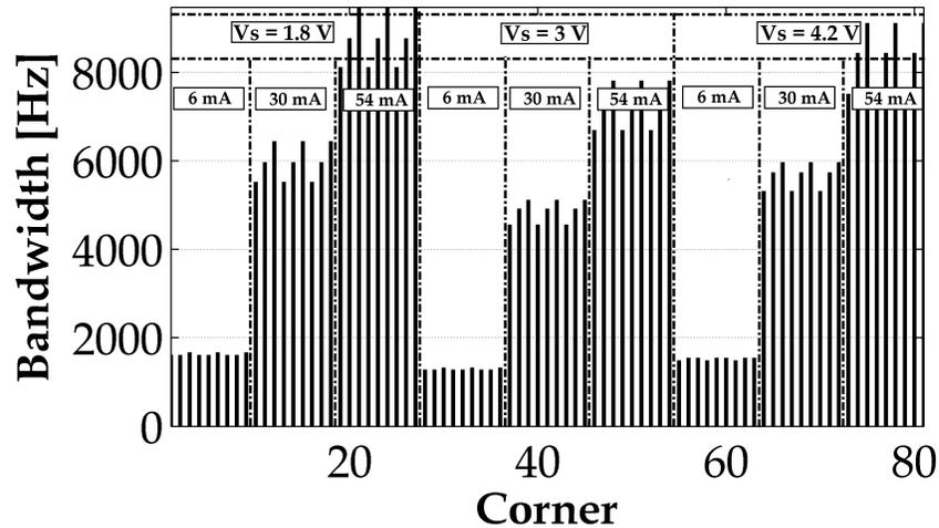
**Figure 5.18:** DCM Boost Converter Bandwidth Over Parameter Corners.  $V_S = [1.8 V, 3 V, 4.2 V]$ ,  $I_O = [6 mA, 30 mA, 54 mA]$ ,  $L = [15 \mu H, 20 \mu H, 25 \mu H]$ ,  $g_m = [8 mS, 10 mS, 12 mS]$ .
