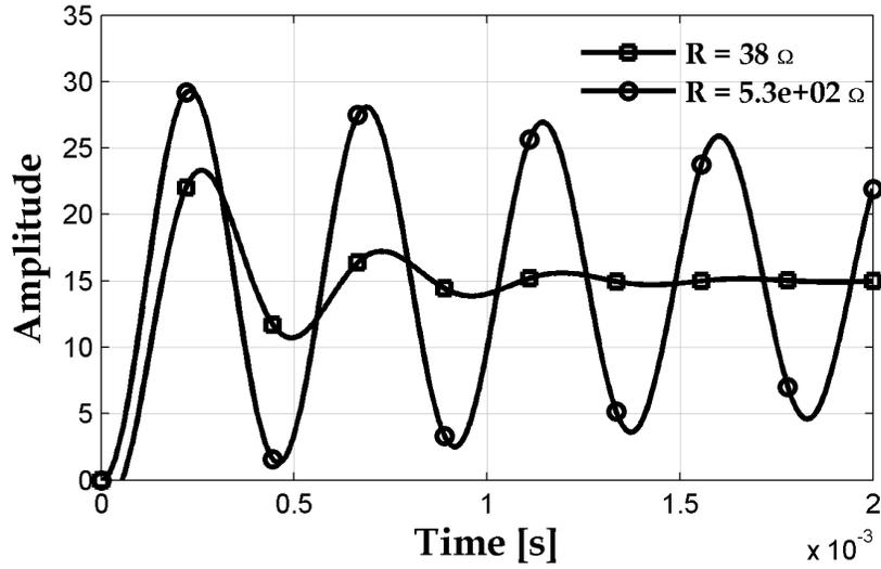
**Figure 3.15:** Step Response for Ideal Boost in CCM with  $L = 180 \mu H$ ,  $C = 4.7 \mu F$ ,  $F_S = 350 kHz$ , and  $\frac{V_O}{V_S} = 2.5$ .
