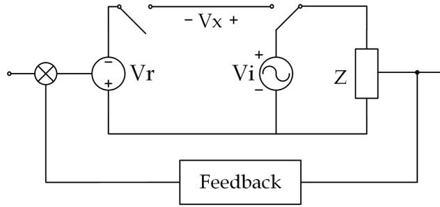
**Figure 6.3:** Voltage Injection via Opening the Loop (Adapted from [32]).
