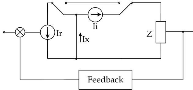
**Figure 6.5:** Current Injection via Opening the Loop (Adapted from [32]).
