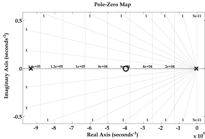
Figure 5.13: DCM Boost Converter Pole-Zero Plot (RHPZ Not Shown)
