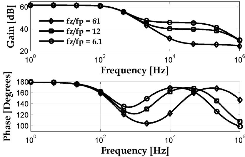
**Figure 4.6:** Bode Plot for Lag Compensator Circuit Plus Pole with  $R_O = 6\text{ k}\Omega$ ,  $C_Z = 100\text{ nF}$ ,  $C_C = 1\text{ nF}$ ,  $g_m = -1\text{ S}$ ,  $R_T = 2\text{ M}\Omega$ ,  $R_B = 500\text{ k}\Omega$  and  $R_Z$  swept with values of  $100\text{ }\Omega$ ,  $500\text{ }\Omega$ , and  $1\text{ k}\Omega$ .
