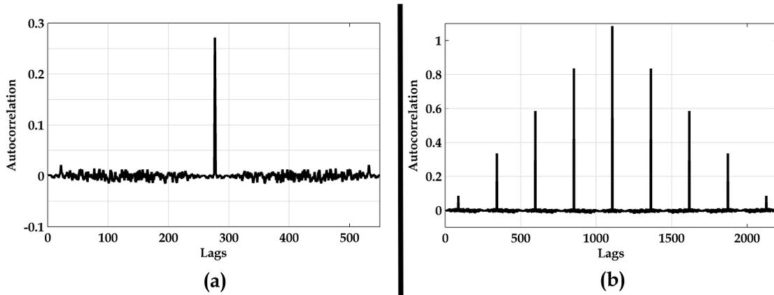
**Figure 6.10:** Autocorrelation of (a) Single-Period 8-bit PRBS, and (b) Four-Period 8-bit PRBS.
