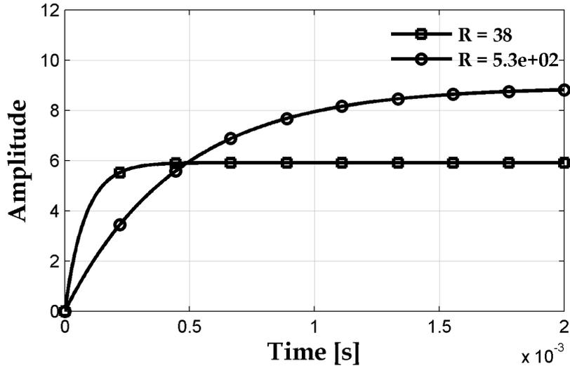
**Figure 3.22:** Step Response for Non-Ideal Boost in DCM with  $L = 18 \mu H$ ,  $C = 4.7 \mu F$ ,  $F_S = 350 kHz$ ,  $\frac{V_O}{V_S} = 1.6$ ,  $r_L = 0.8 \Omega$ , and  $r_C = 0.1 \Omega$ .
