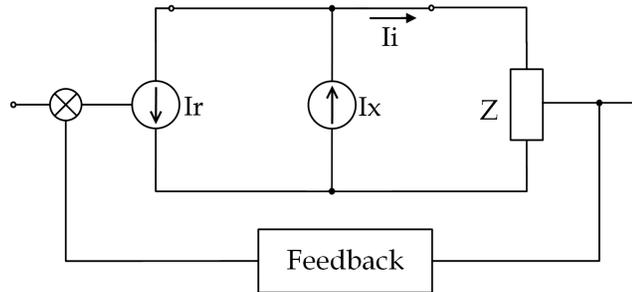
**Figure 6.6:** Current Injection via Middlebrook's Method.
