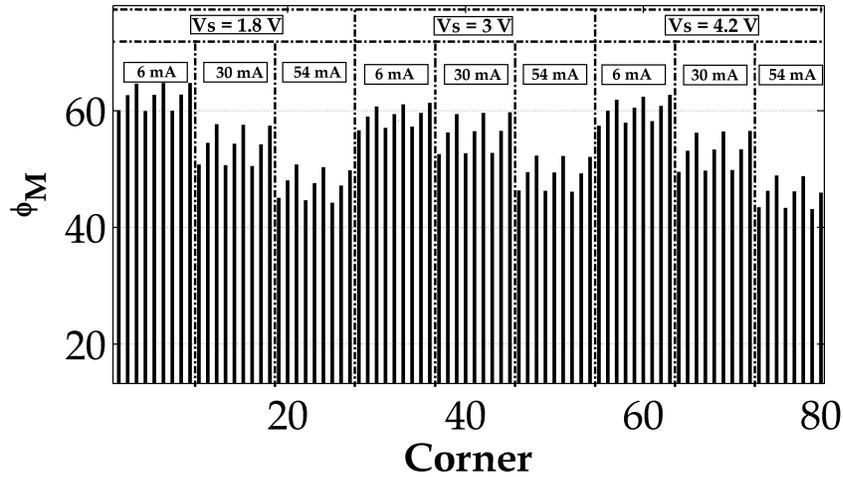
**Figure 5.17:** DCM Boost Converter Phase Margin Over Parameter Corners.  $V_S = [1.8 V, 3 V, 4.2 V]$ ,  $I_O = [6 mA, 30 mA, 54 mA]$ ,  $L = [15 \mu H, 20 \mu H, 25 \mu H]$ ,  $g_m = [8 mS, 10 mS, 12 mS]$ .
