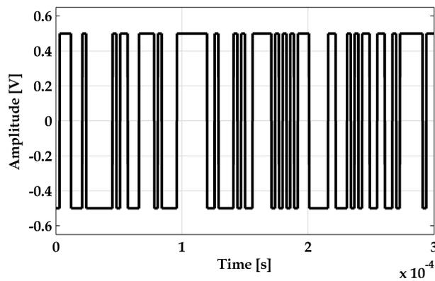
**Figure 6.9:** 8-bit PRBS Signal.
