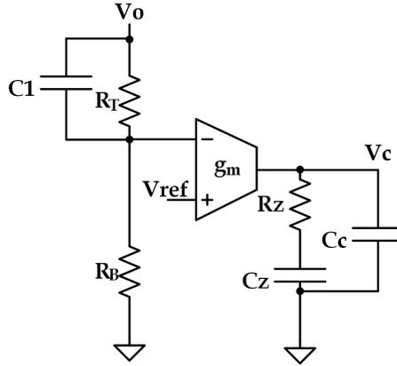
Figure 4.11: Lag-Lead Compensator Circuit
