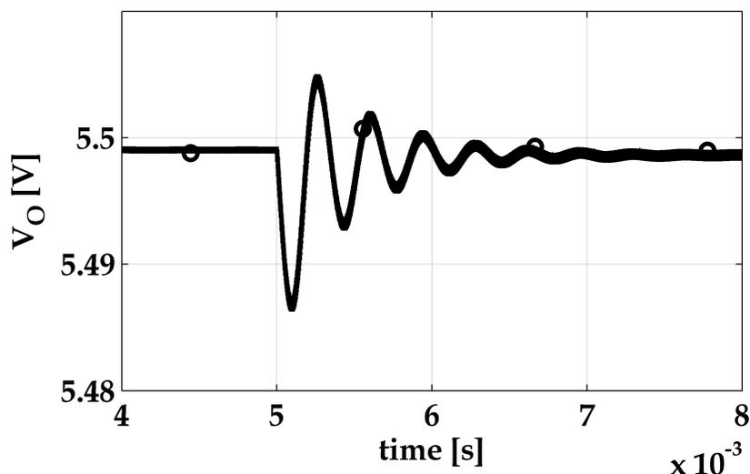
**Figure 6.1:** DCM Boost Converter Load Step from 10 mA to 20 mA with an Underdamped Step Response
