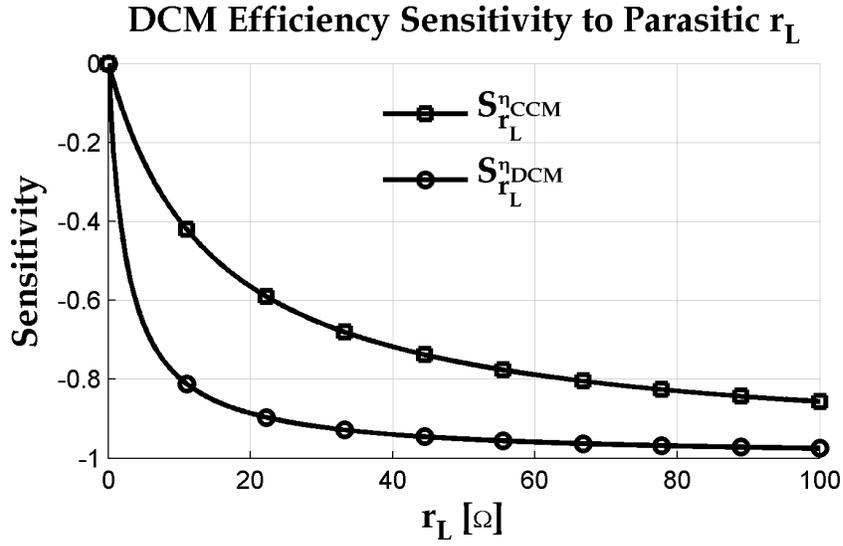
**Figure 2.8:** Sensitivity of Efficiency to Changing  $r_L$  for CCM and DCM
