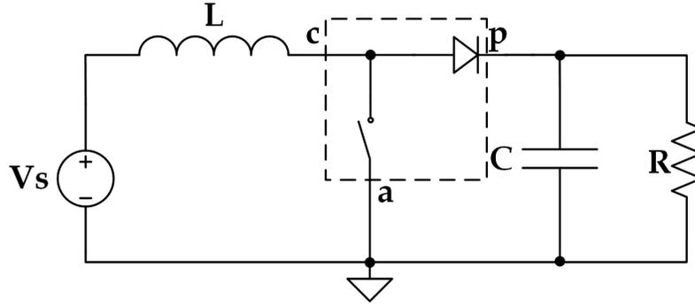
**Figure 3.7:** Ideal Boost Converter with Common-Active PWM Switch
