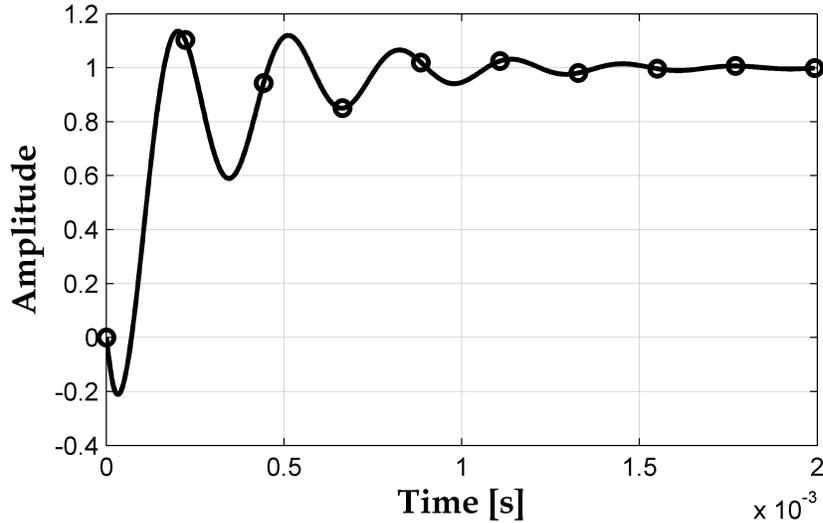
**Figure 5.6:** CCM Boost Converter Step-Response with PID Control
