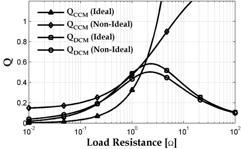
**Figure 3.27:** Quality Factor Comparison for Varying Load Resistances with  $L = 18 \mu H$ ,  $C = 4.7 \mu F$ ,  $F_S = 350 kHz$ , and  $M = 1.6$ .
