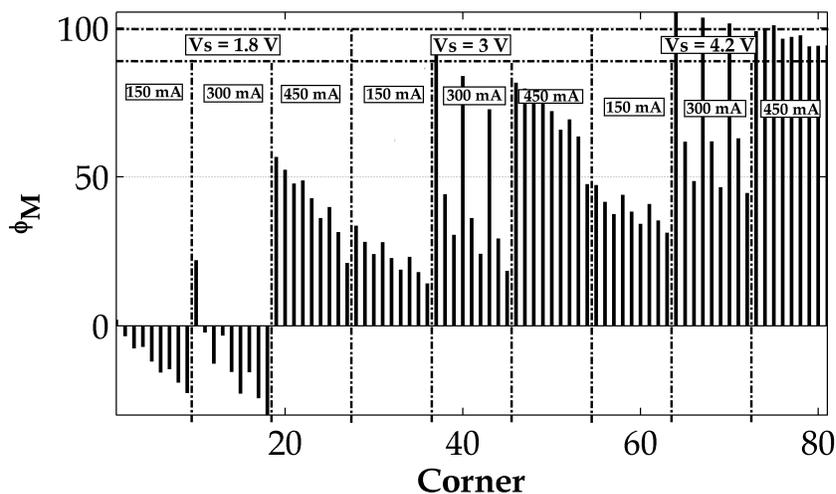
**Figure 5.7:** CCM Boost Converter Phase Margin Over Parameter Corners.  $V_S = [1.8\text{ V}, 3\text{ V}, 4.2\text{ V}]$ ,  $I_O = [150\text{ mA}, 300\text{ mA}, 450\text{ mA}]$ ,  $L = [170\text{ }\mu\text{H}, 200\text{ }\mu\text{H}, 230\text{ }\mu\text{H}]$ ,  $g_m = [0.93\text{ }\mu\text{S}, 1.03\text{ }\mu\text{S}, 1.13\text{ }\mu\text{S}]$ .
