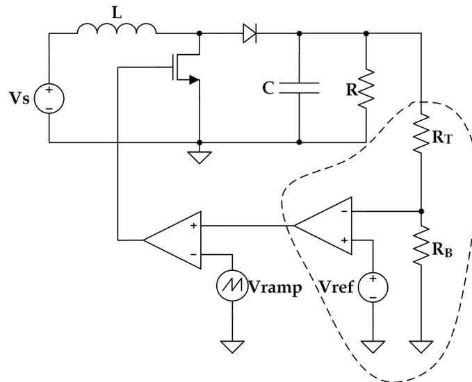
**Figure 4.2:** Circuit Implementation of a Voltage-Mode Controlled Boost Converter
