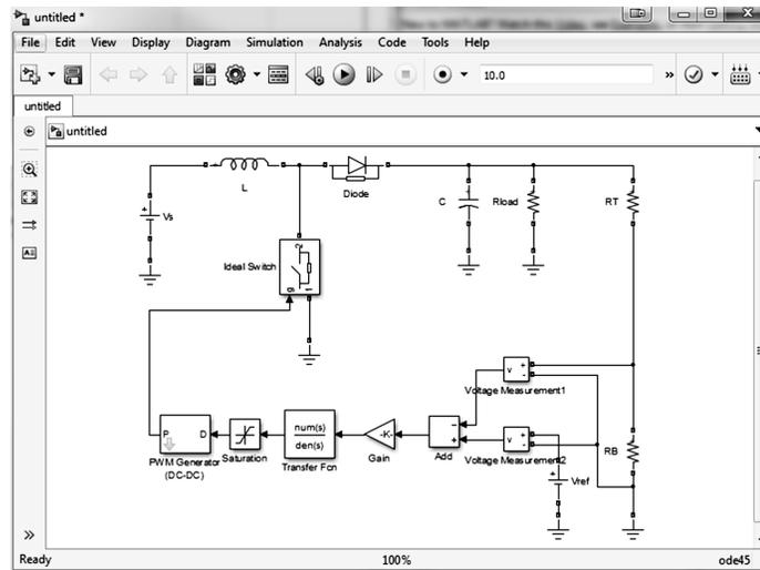
**Figure B.5:** Boost Converter in Powerlib
