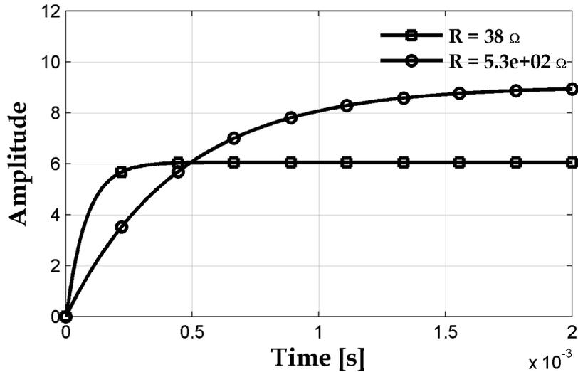
**Figure 3.21:** Step Response for Ideal Boost in DCM with  $L = 18 \mu H$ ,  $C = 4.7 \mu F$ ,  $F_S = 350 kHz$ , and  $\frac{V_O}{V_S} = 1.6$ .
