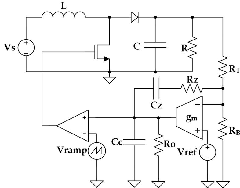
**Figure 5.11:** Boost Converter with PI Control
