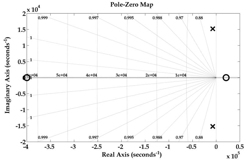
Figure 5.3: CCM Boost Converter Pole-Zero Plot
