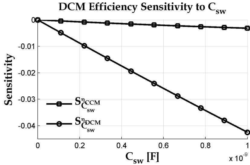
**Figure 2.9:** Sensitivity of Efficiency to Changing  $C_{sw}$  for CCM and DCM
