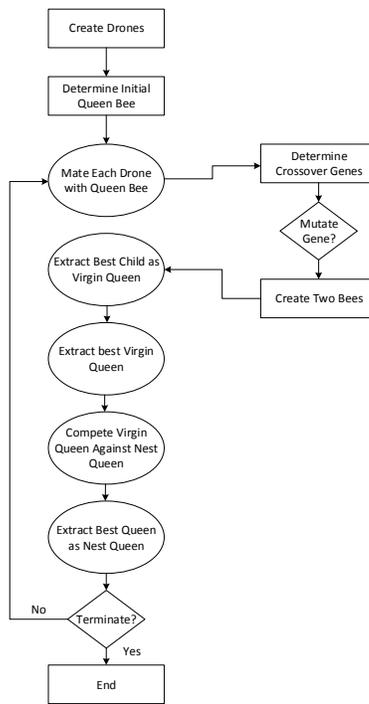
**Figure A.1:** Block Diagram for a Queen-Bee Genetic Algorithm for Optimization of Switched-Converter Controller Transfer Function.
