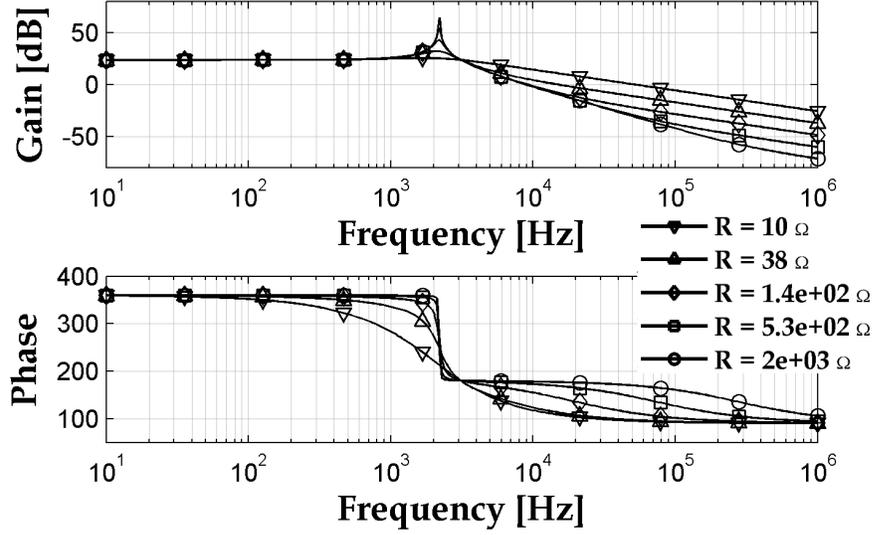
**Figure 3.13:** Bode Plot for Ideal Boost in CCM with  $L = 180 \mu H$ ,  $C = 4.7 \mu F$ ,  $F_S = 350 kHz$ , and  $\frac{V_O}{V_S} = 2.5$ .
