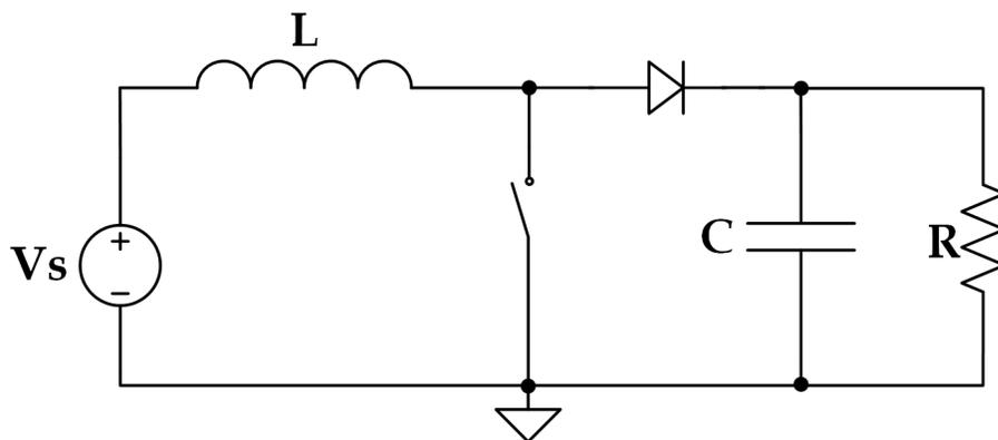
**Figure 2.1:** Ideal Boost Converter Circuit
