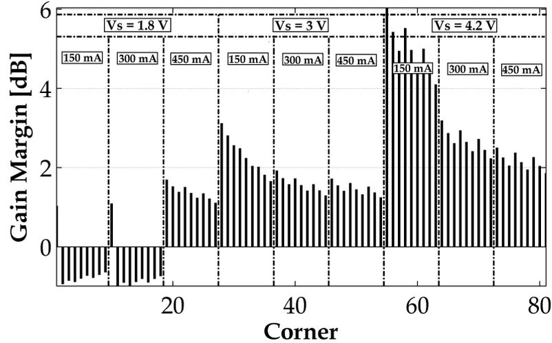
**Figure 5.9:** CCM Boost Converter Gain Margin Over Parameter Corners.  $V_S = [1.8 V, 3 V, 4.2 V]$ ,  $I_O = [150 mA, 300 mA, 450 mA]$ ,  $L = [170 \mu H, 200 \mu H, 230 \mu H]$ ,  $g_m = [0.93 \mu S, 1.03 \mu S, 1.13 \mu S]$ .
