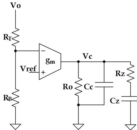
Figure 4.5: Lag Compensator Circuit
