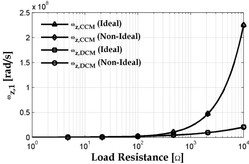
Figure 3.29: RHP Zero Comparison for Varying Load Resistances with  $L = 18 \mu H$ ,  $C = 4.7 \mu F$ ,  $F_S = 350 kHz$ , and  $M = 1.6$ .
