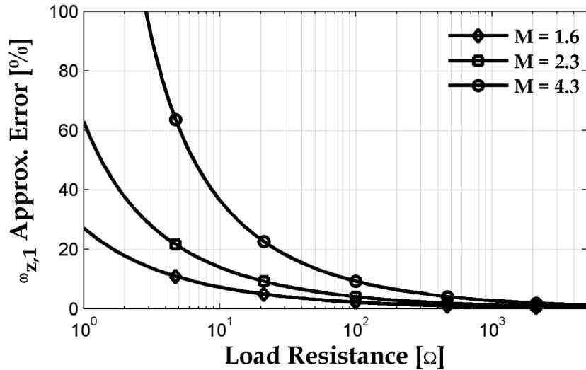
Figure 3.30: RHP Zero DCM Approximation Error
