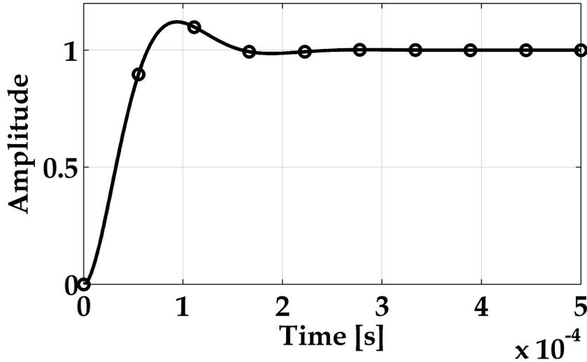
Figure 5.16: DCM Boost Converter with PI Control Step Response
