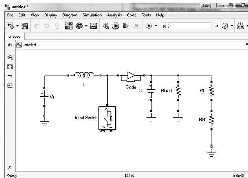
**Figure B.4:** Boost Converter in Powerlib (no Controller)
