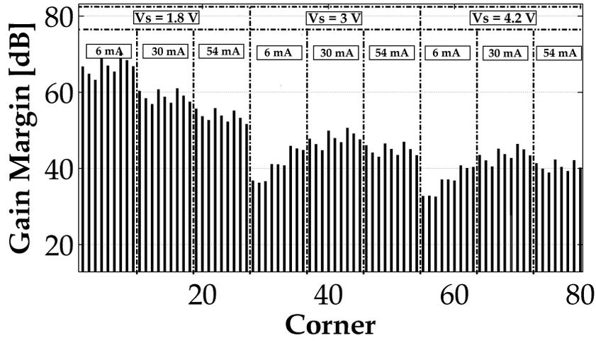
**Figure 5.19:** DCM Boost Converter Gain Margin Over Parameter Corners.  $V_S = [1.8V, 3V, 4.2V]$ ,  $I_O = [6mA, 30mA, 54mA]$ ,  $L = [15\mu H, 20\mu H, 25\mu H]$ ,  $g_m = [8mS, 10mS, 12mS]$ .
