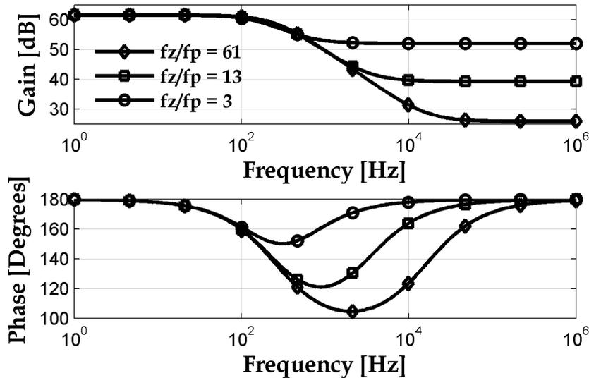
**Figure 4.4:** Bode Plot for Lag Compensator Circuit with  $R_O = 6 \text{ k}\Omega$ ,  $C_Z = 100 \text{ nF}$ ,  $g_m = -1 \text{ S}$ ,  $R_T = 2 \text{ M}\Omega$ ,  $R_B = 500 \text{ k}\Omega$  and  $R_Z$  swept with values of  $100 \text{ }\Omega$ ,  $500 \text{ }\Omega$ , and  $3 \text{ k}\Omega$ .
