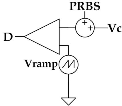
**Figure 6.11:** Injection Point for PRBS in a Switched DC-DC Converter
