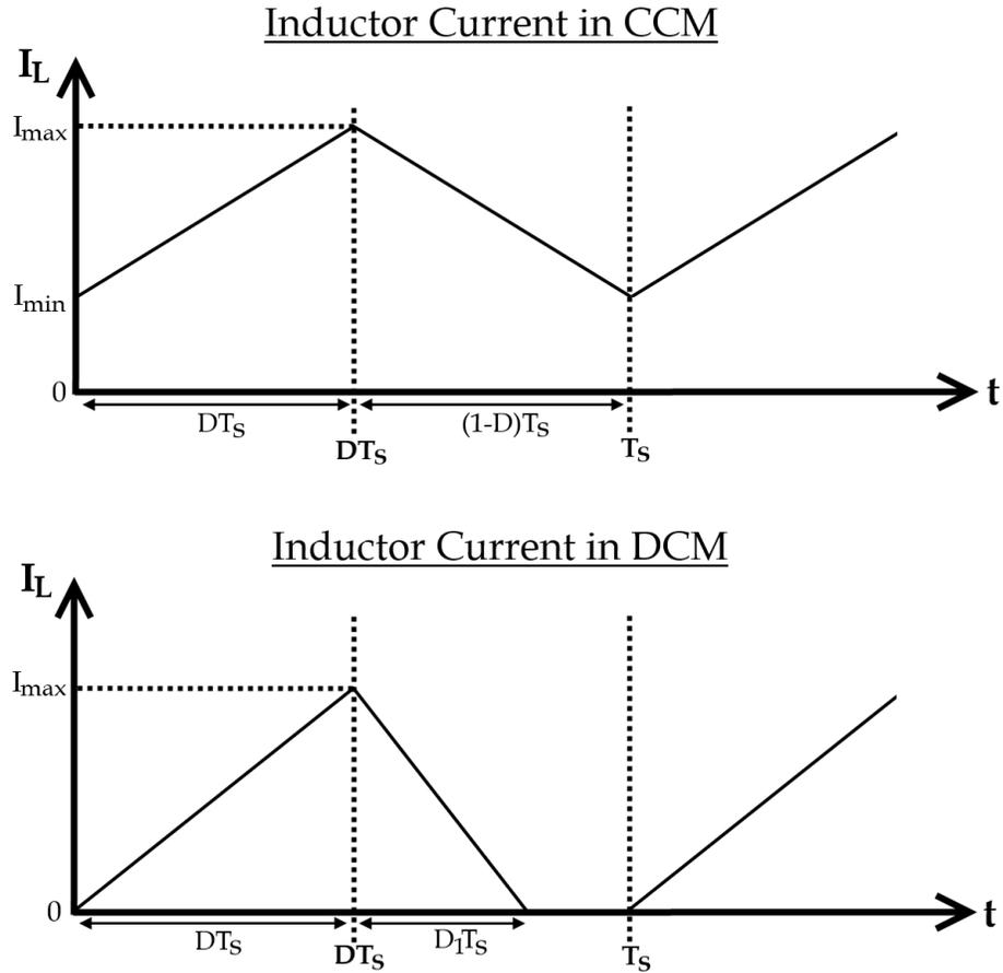
**Figure 2.2:** Inductor Current in Boost Converter for CCM and DCM
