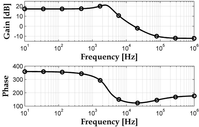
Figure 5.2: CCM Boost Converter Bode Plot
