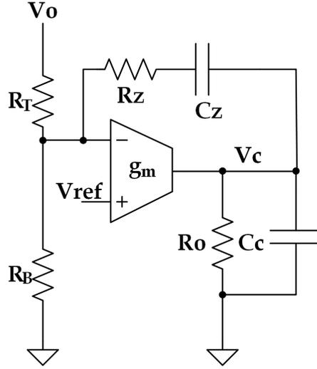
Figure 4.7: Lag Compensator Circuit with Feedback Zero
