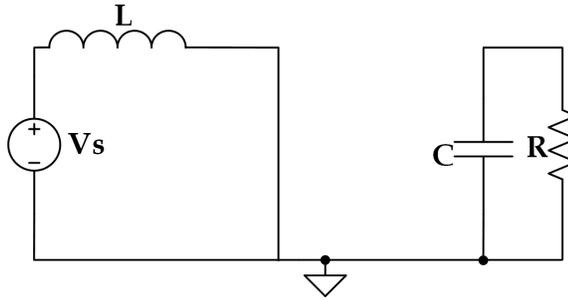
**Figure 3.4:** Ideal Boost Converter with Switch Closed
