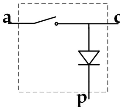
**Figure 3.6:** PWM Switch (adapted from [18] and [19])
