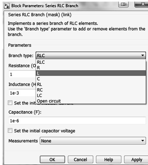
**Figure B.3:** Changing Series RLC Branch Parameters
