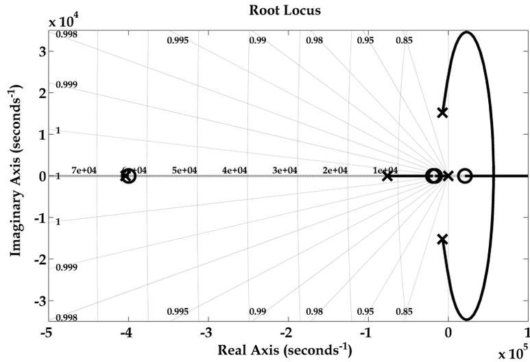
**Figure 5.5:** CCM Boost Converter Root-Locus with PID Control
