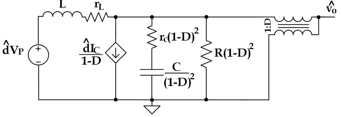
**Figure 3.12:** Equivalent Small-Signal Boost Circuit in CCM with Non-Idealities Included
