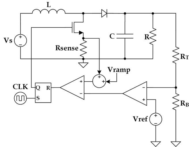
**Figure 4.1:** Boost Converter with Current Mode Control (Adapted from [29])
