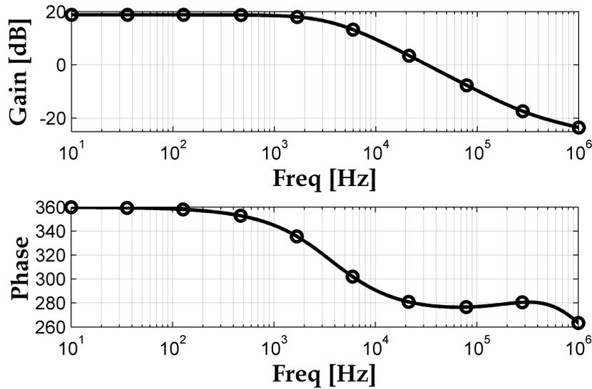
Figure 5.12: DCM Boost Converter Bode Plot
