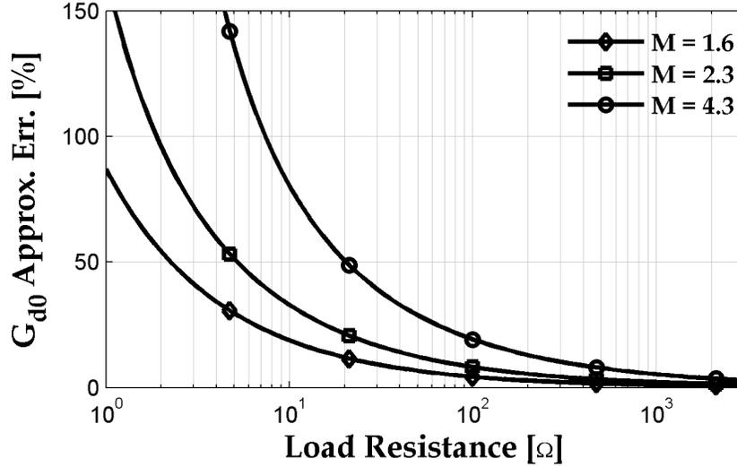
**Figure 3.24:** Open-Loop Gain DCM Approximation Error
