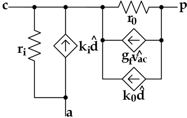
**Figure 3.9:** Equivalent Circuit for Small-Signal PWM Switch in DCM
