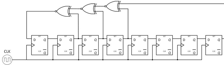
**Figure 6.8:** 8-bit PRBS Circuit.
