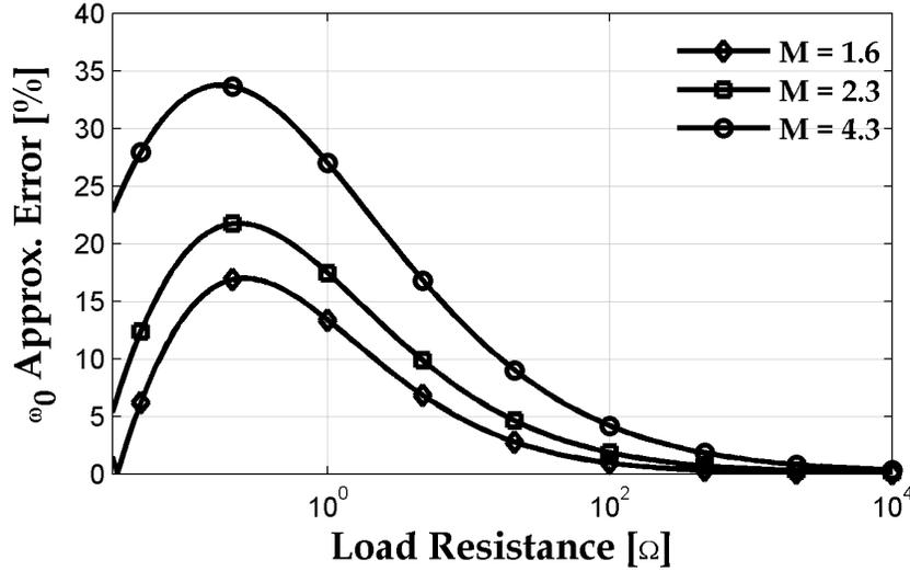
**Figure 3.26:** Resonant Frequency DCM Approximation Error
