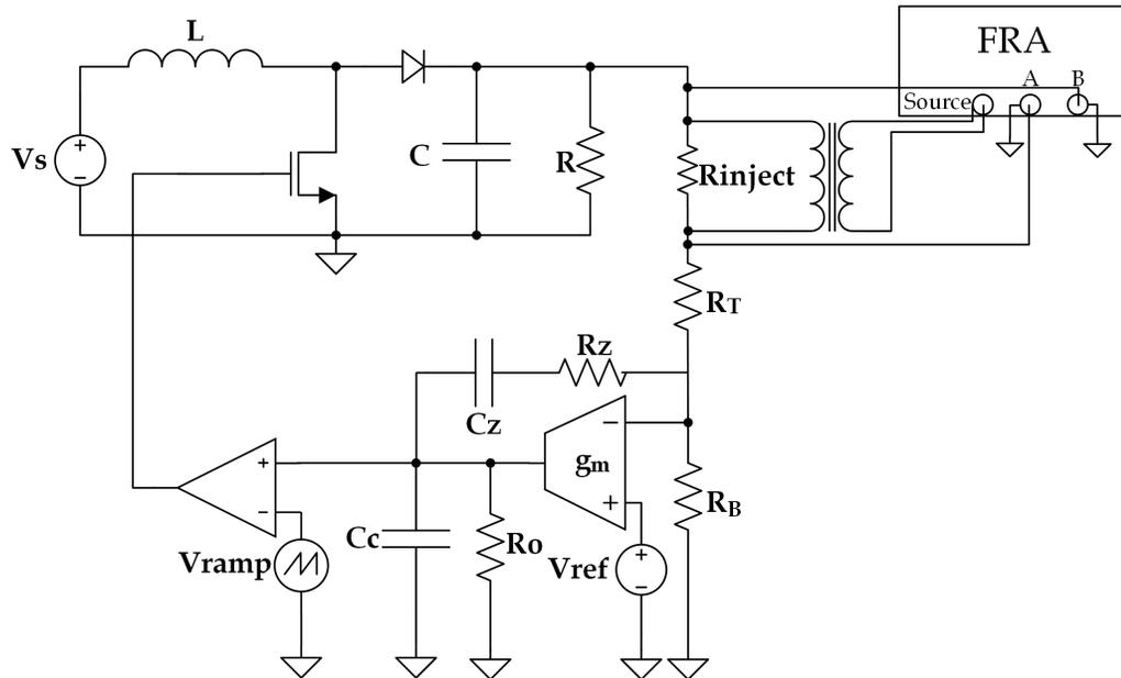
**Figure 6.7:** Voltage Injection Test Setup.
