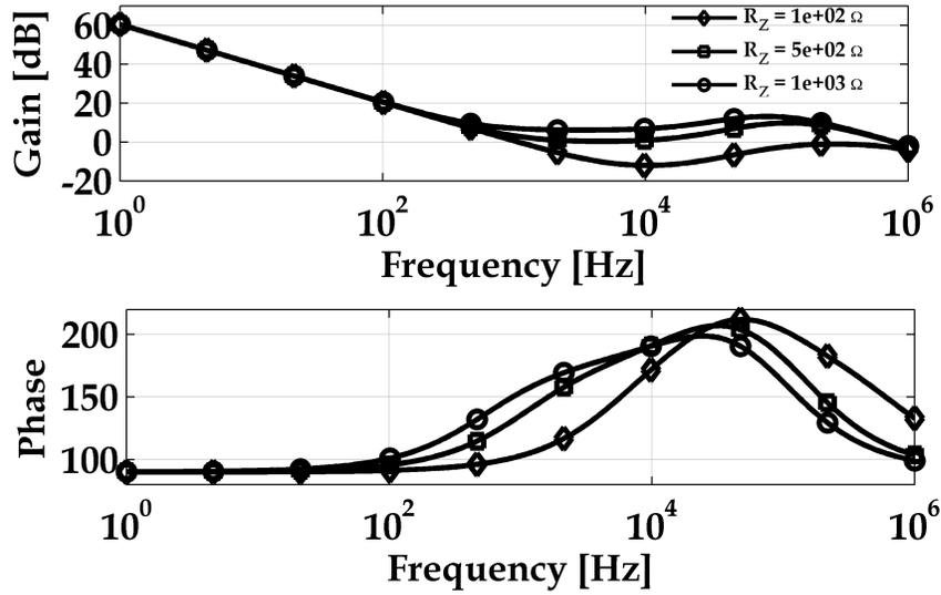
**Figure 4.12:** Bode Plot for Lag-Lead Compensator Circuit with  $C_1 = 0.8\text{ pF}$ ,  $C_C = 2\text{ nF}$ ,  $g_m = -10\text{ }\mu\text{S}$ ,  $R_B = 500\text{ k}\Omega$ ,  $R_T = 2\text{ M}\Omega$ ,  $C_Z = 300\text{ nF}$ , and  $R_Z$  swept with values of  $100\text{ }\Omega$ ,  $500\text{ }\Omega$ , and  $1\text{ k}\Omega$ .
