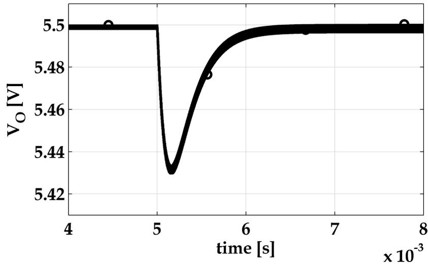
**Figure 6.2:** DCM Boost Converter Load Step from 10 mA to 20 mA with an Overdamped Step Response
