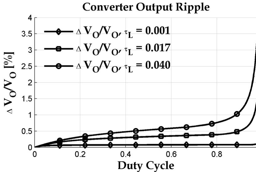
Figure 2.7: Output Ripple Voltage versus Duty Cycle Comparison for DCM and CCM
