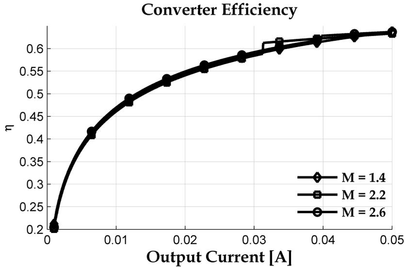
Figure 2.6: Efficiency versus Output Current Comparison for DCM and CCM
