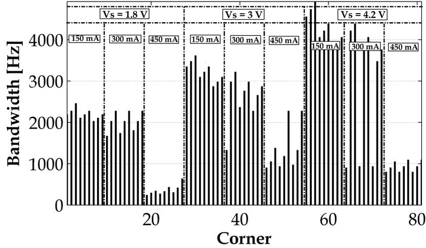
**Figure 5.8:** CCM Boost Converter Bandwidth Over Parameter Corners.  $V_S = [1.8 V, 3 V, 4.2 V]$ ,  $I_O = [150 mA, 300 mA, 450 mA]$ ,  $L = [170 \mu H, 200 \mu H, 230 \mu H]$ ,  $g_m = [0.93 \mu S, 1.03 \mu S, 1.13 \mu S]$ .
