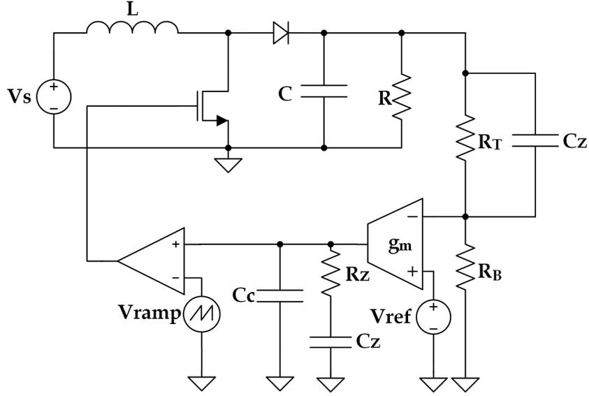
**Figure 5.1:** Boost Converter with PID Control
