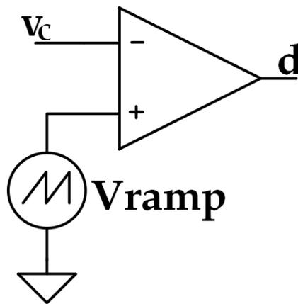
Figure 3.2: PWM Generation Circuit
