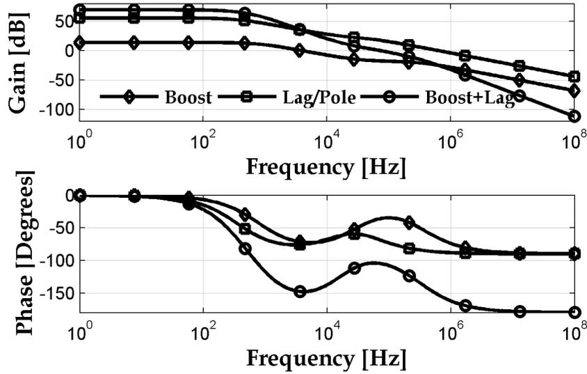
**Figure 4.15:** Bode Plot for Lag Compensator Plus Pole with DCM Boost with  $G_{d0} = 5$ ,  $C_O = 10 \mu F$ ,  $R_{ESR} = 0.5 \Omega$ ,  $Q = 0.05$ ,  $f_0 = 16 kHz$ ,  $R_O = 3 k\Omega$ ,  $R_Z = 100 \Omega$ ,  $C_Z = 10 \mu F$ ,  $C_C = 50 nF$ ,  $g_m = -1S$ ,  $R_T = 2 M\Omega$ , and  $R_B = 500 k\Omega$
