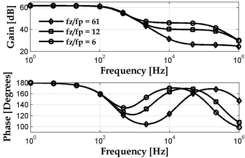
Figure 4.8: Bode Plot for Lag Compensator Circuit Plus Pole with  $R_O = 6 \text{ k}\Omega$ ,  $C_Z = 250 \text{ fF}$ ,  $C_C = 1 \text{ nF}$ ,  $g_m = -1 \text{ S}$ ,  $R_T = 2 \text{ M}\Omega$ ,  $R_B = 500 \text{ k}\Omega$  and  $R_Z$  swept with values of  $40.7 \text{ M}\Omega$ ,  $218 \text{ M}\Omega$ , and  $480 \text{ M}\Omega$ .
