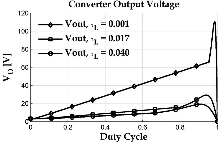
**Figure 2.5:** Output Voltage versus Duty Cycle Comparison for DCM and CCM
