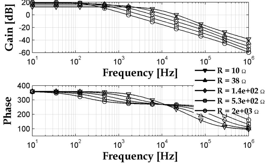
**Figure 3.19:** Bode Plot for Ideal Boost in DCM with  $L = 18 \mu H$ ,  $C = 4.7 \mu F$ ,  $F_S = 350 kHz$ , and  $\frac{V_O}{V_S} = 1.6$ .
