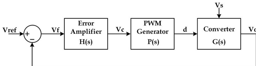
**Figure 3.1:** Regulated DC Converter Block Diagram (Adapted from [13])
