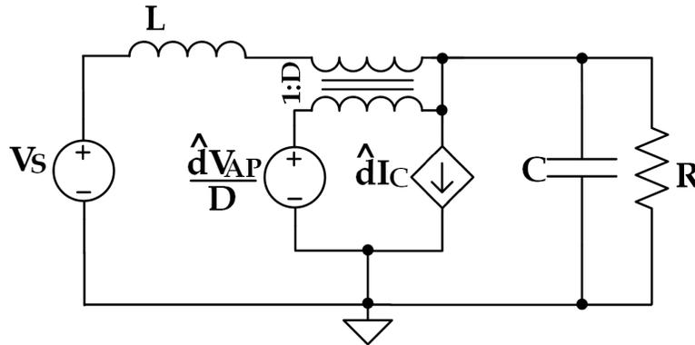
**Figure 3.10:** Equivalent Small-Signal Boost Circuit in CCM
