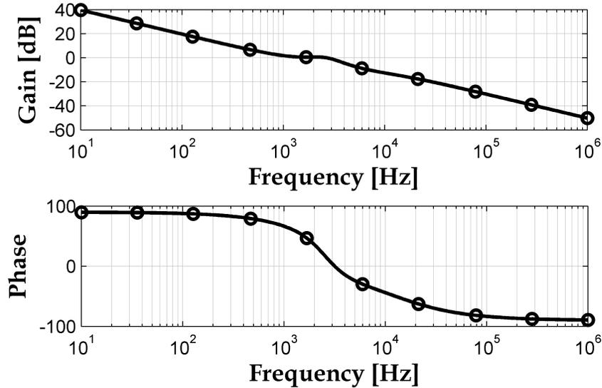
**Figure 5.4:** CCM Boost Converter Bode Plot with PID Control;  $g_m = 1.03 \mu S$ ,  $R_B = 560 k\Omega$ ,  $R_T = 2 M\Omega$ ,  $R_Z = 200 k\Omega$ ,  $C_C = 13 pF$ ,  $C_Z = 260 pF$ ,  $C_1 = 30 pF$ .
