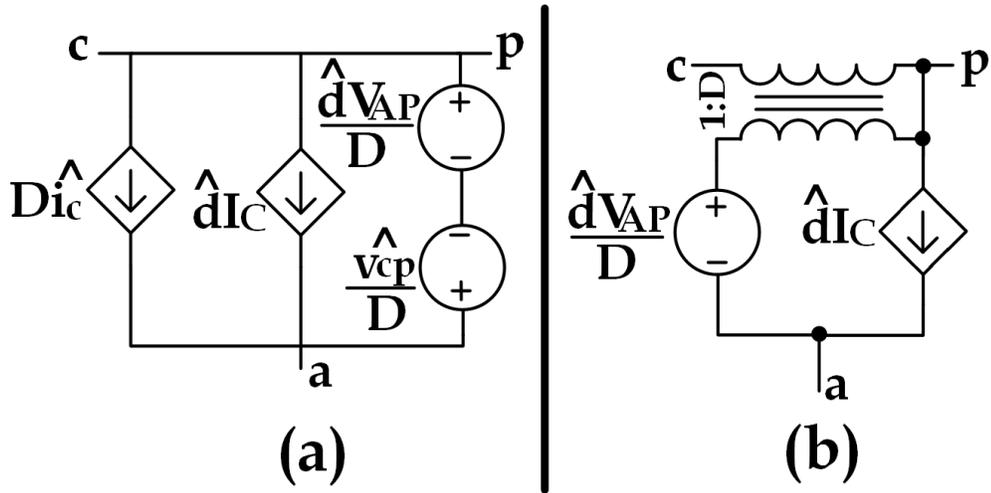
**Figure 3.8:** Common-Active PWM Model in CCM (a) direct equation-to-circuit model (b) transformer model
