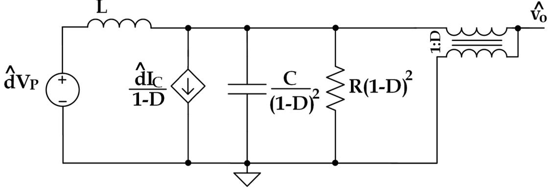
**Figure 3.11:** Equivalent Small-Signal Boost Circuit in CCM After Transformation Given in [21]
