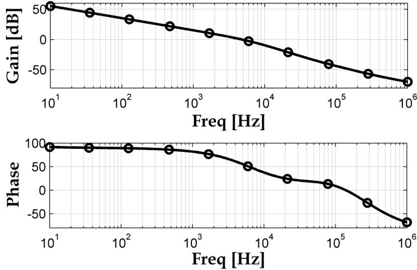
Figure 5.14: DCM Boost Converter with PI Control Bode Plot
