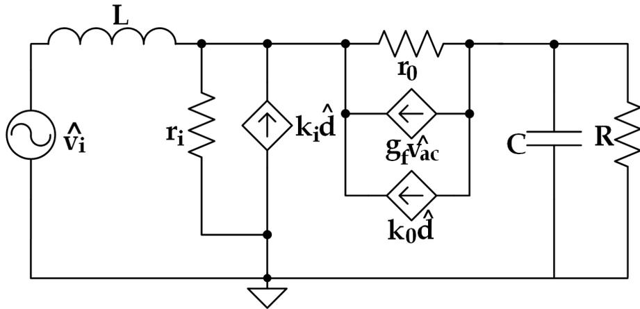
**Figure 3.17:** Equivalent Small-Signal Boost Circuit in DCM
