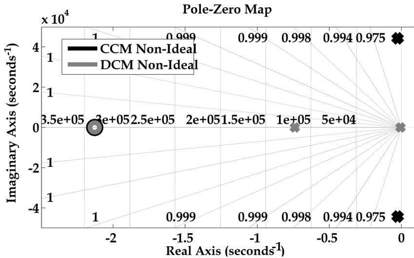
Figure 3.31: Pole Zero plot for Non-Ideal CCM and DCM Transfer Functions (RHPZs Not Plotted)
