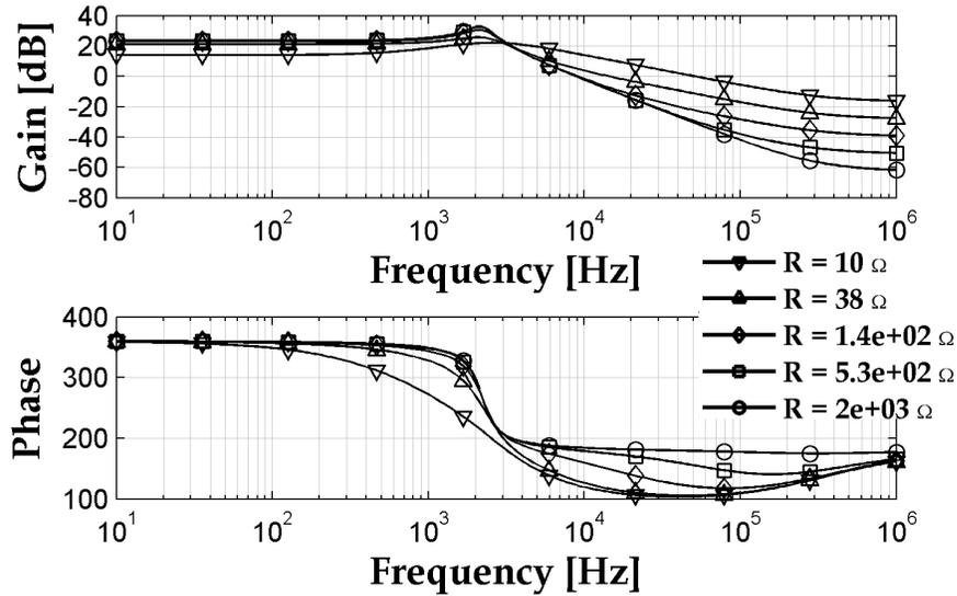
**Figure 3.14:** Bode Plot for Non-Ideal Boost in CCM with  $L = 180 \mu H$ ,  $C = 4.7 \mu F$ ,  $F_S = 350 kHz$ ,  $\frac{V_O}{V_S} = 2.5$ ,  $r_L = 0.8 \Omega$ , and  $r_C = 0.1 \Omega$ .
