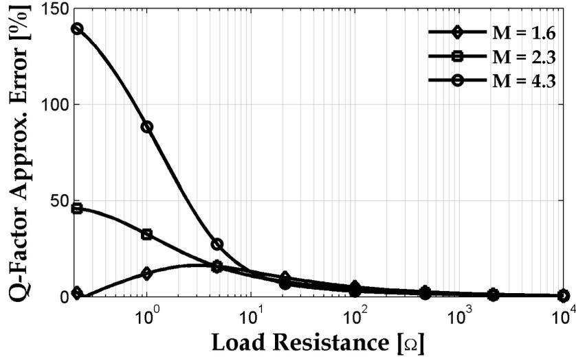
Figure 3.28: Quality Factor DCM Approximation Error
