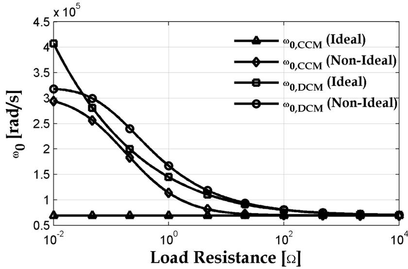
**Figure 3.25:** Resonant Frequency Comparison for Varying Load Resistances with  $L = 18 \mu H$ ,  $C = 4.7 \mu F$ ,  $F_S = 350 kHz$ , and  $M = 1.6$ .
