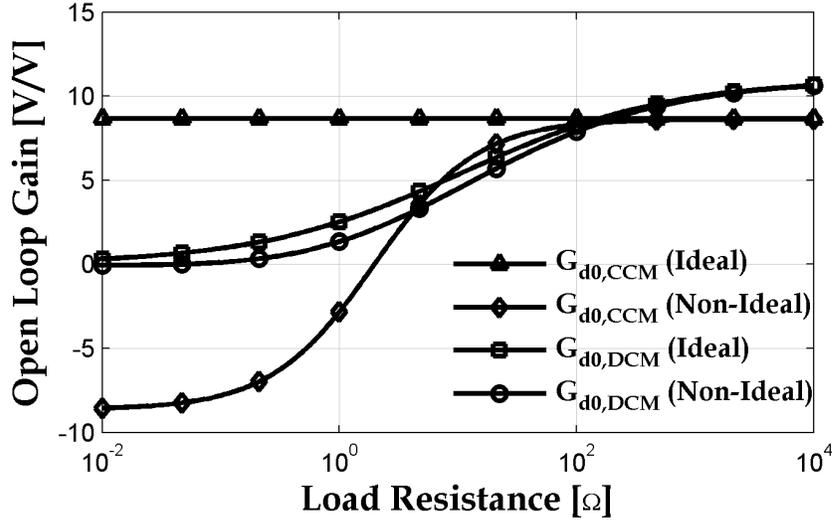
**Figure 3.23:** Open-Loop Gain Comparison for Varying Load Resistances with  $L = 18 \mu H$ ,  $C = 4.7 \mu F$ ,  $F_S = 350 kHz$ , and  $M = 1.6$ .
