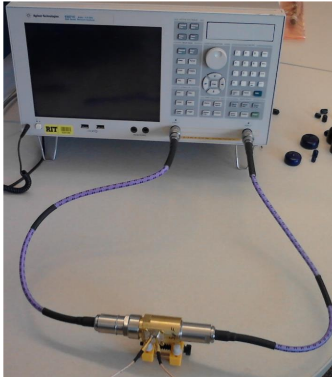
Fig. 5-6: The TXC test structure attached to the VNA with precision phase stable cables.
