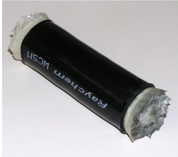
Fig. 3.2. The 2.8cm diameter hand-made glass fiber phantom for MRI measurements.
