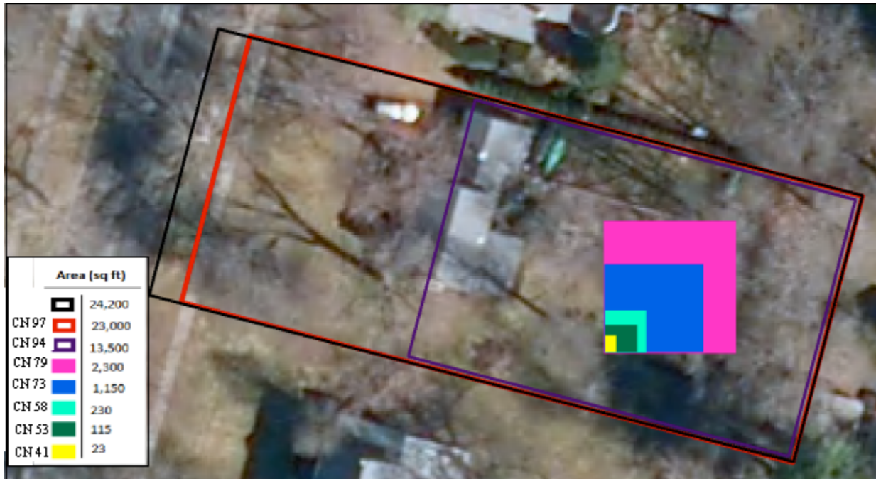
Figure 13. Scale model of an average sized residential property (indicated by the black outline) in the area of interest compared to various abatement burdens (indicated by the red and purple outlines and solid boxes) required by corresponding development scenarios.
