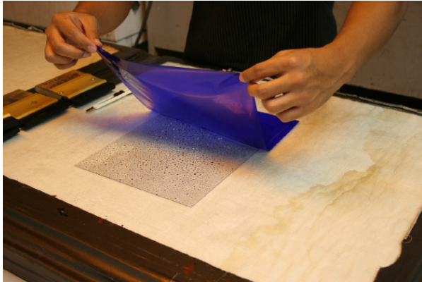
Lamination of ImagOn film onto a PETG (Polyethylene Terephthalate Glycol) Plastic Printmaking Plate, which is an inexpensive alternative to traditional copper plates.
