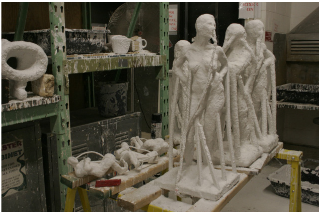
Sculptures during the ceramic shell process. The wax figures being coated with multiple layers of ceramic shell slurry after the sprues and vents are welded.
