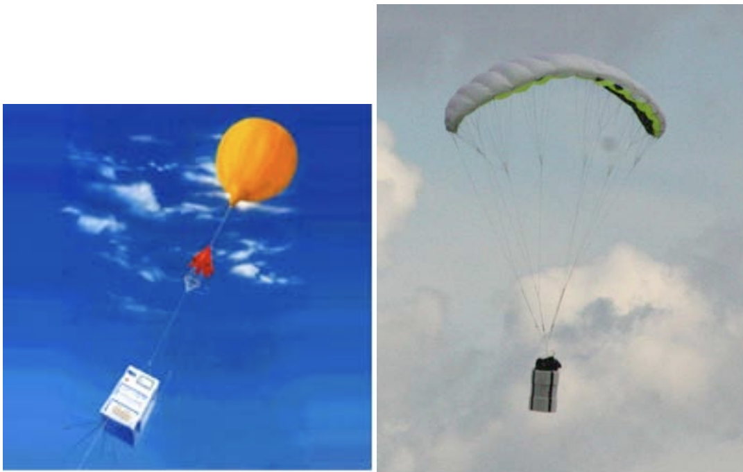
Figure 13. Radiosonde device during ascent phase (left) (Radiosonde, 2009) and descent phase (right)(Radiosonde2, 2009)
