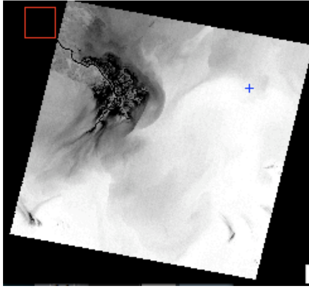
Figure 31. ENVI is used to display a Landsat scene and a shapefile is created from the geographic location of the buoy. ENVI will geometrically place the buoy on the scene (blue crosshair)
