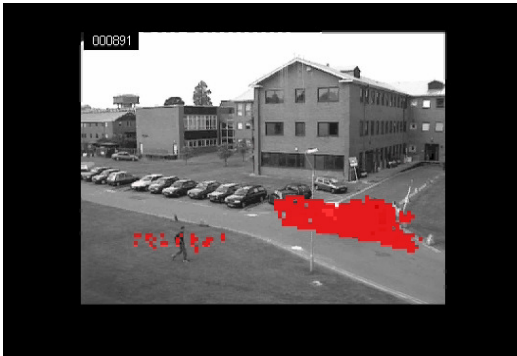
FIGURE 3.10 – Motion Detection “Ghosting” At Low Frame Rates.
