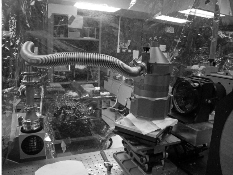
Figure 5.5: Dewar containing an un-biased DMD was setup on a Zygo HeNe interferometer.
