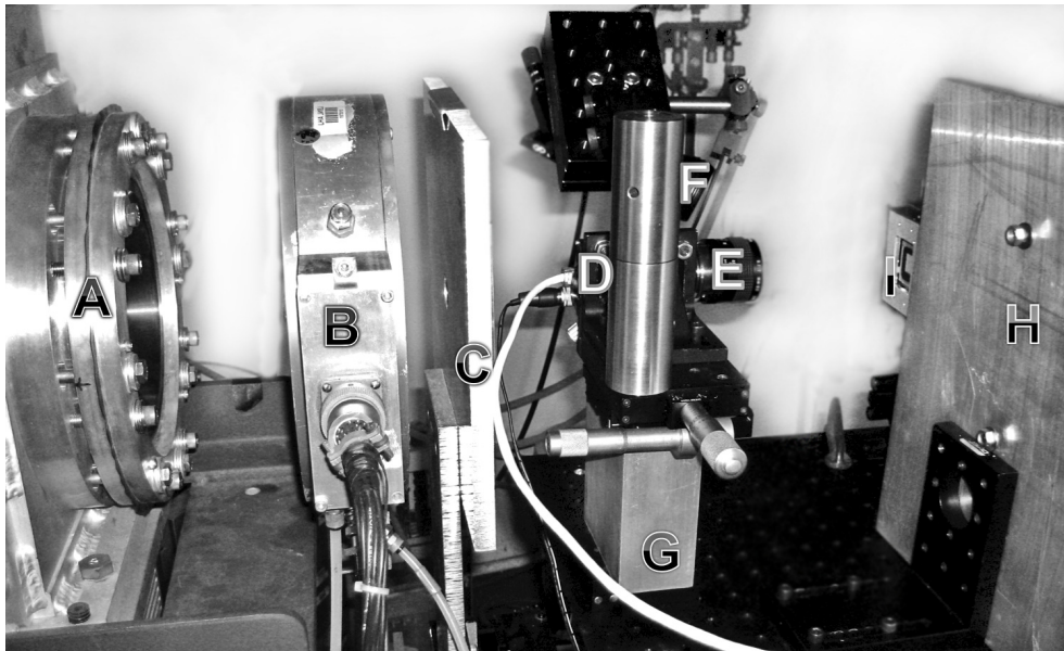
Figure 4.5: Parts of the experimental apparatus are as follows: (A) is the proton beam-line exit port, (B) ionization chamber, (C) aluminum aperture plate, (D) high-speed CCD camera, (E) a macro lens, (F) LED light source, (G) kinematic mount, (H) 0.75" aluminum shielding for the drive electronics, and (I) test DMD.
