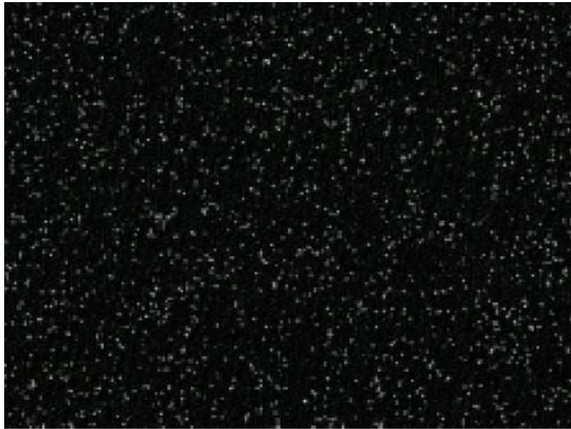
Figure 2.2 A portion of a frame illuminated by the Fe55 X-ray source with Al foil attenuation.
