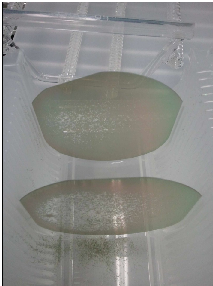
Figure 4.7: NiO de-adhesion from quartz substrates
