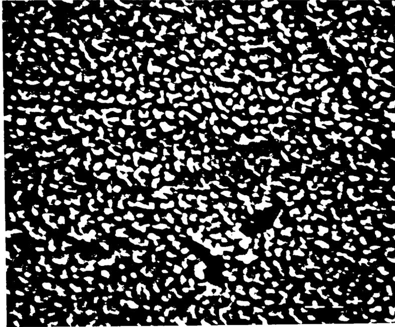
Fig. 3-19. SEM Micrograph of PTFE surface after treatment
