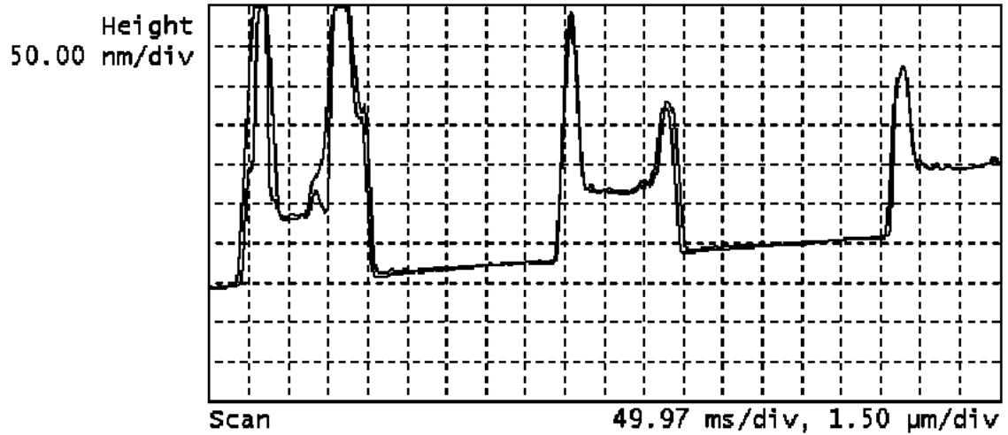
Fig. 3.5. Cross section of repeating regions of thickness loss enhancement, appearing as 10 μm pitch scratches with an 86 nm step height, as measured using AFM.
